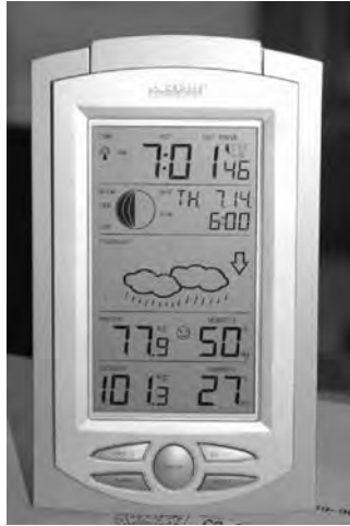
FIGURE 4.8 July 14, 2005. Summertime comfortable temperature spread of 23.4° maintained without mechanical cooling. (Author's photo.)
