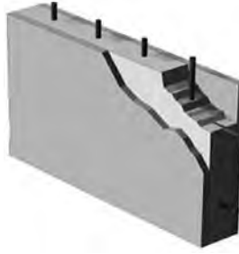
FIGURE 4.3 A state-of-the-art ICF concrete flat wall system. (Courtesy of Portland Cement Association.)
