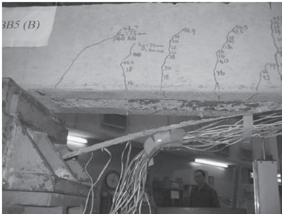
4.8 FRP-plated RC beam: plate-end interfacial debonding.
