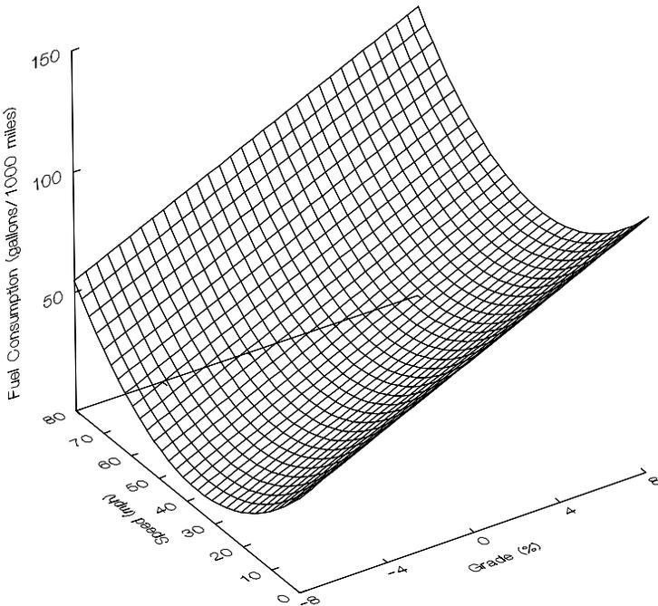
Figure 4.17: Regression function of fuel consumption: medium car.
