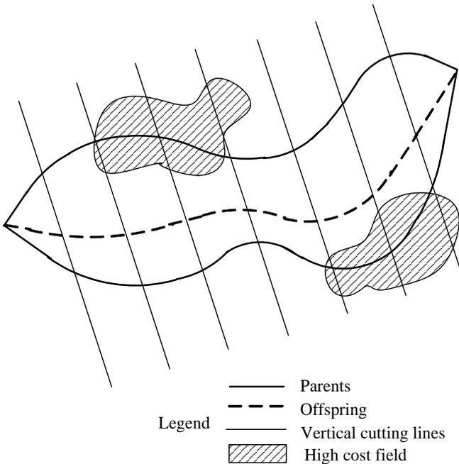
Figure 5.7: An example of an arithmetic crossover operator.
