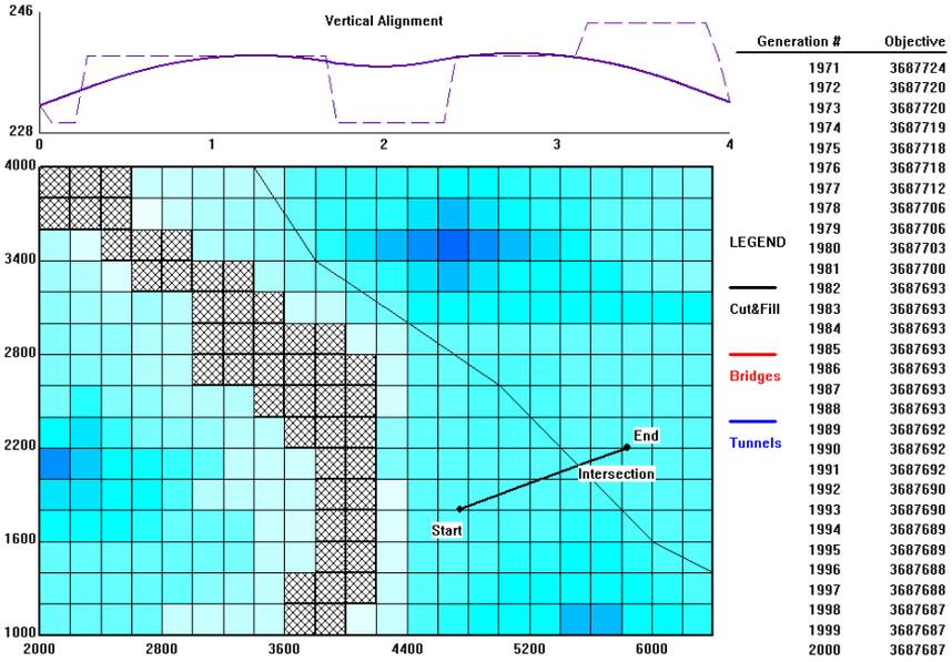
Figure 15.45: Optimized solution for segment 3 under scenario 3.
