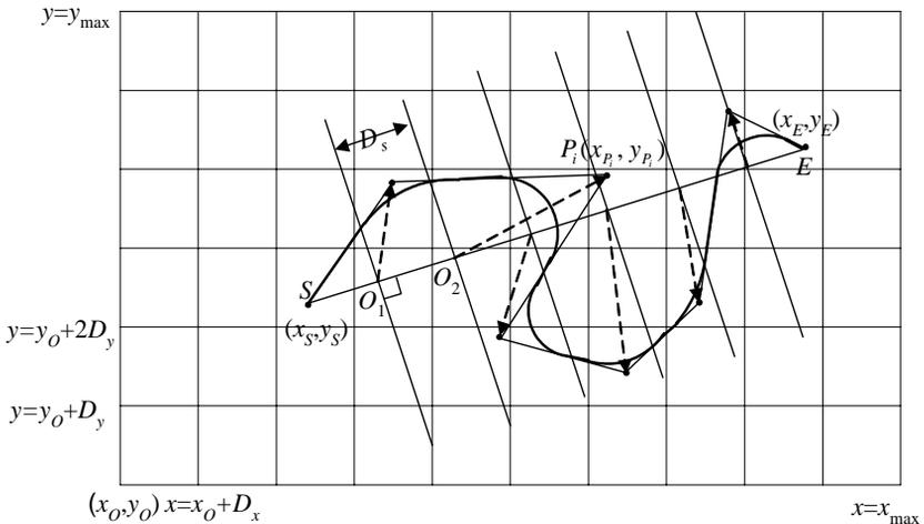
Figure 6.2: An example for modeling backtracking horizontal alignments.
