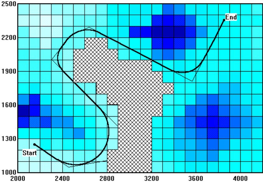
Figure 11.1: Best alignment based on an artificial study area by the developed algorithm.
