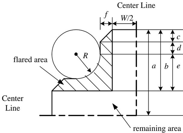
Figure 12.13: Flared and remaining areas of a typical four-legged intersection.
