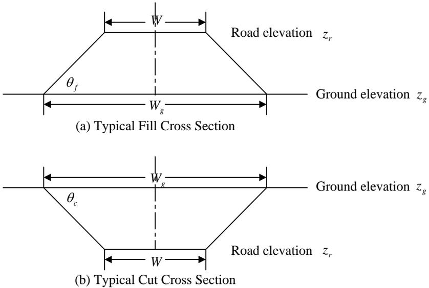
Figure 7.6: Typical fill and cut cross sections.
