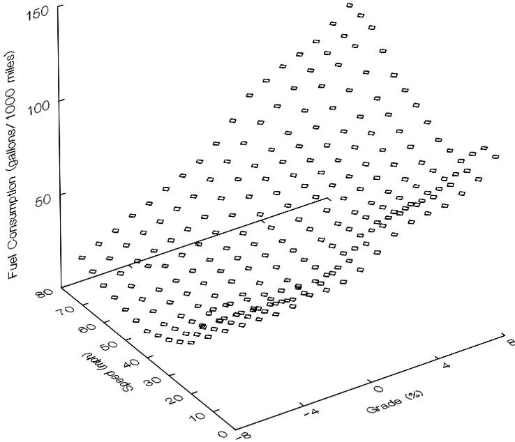
Figure 4.16: Fuel consumption data plots: medium car.
