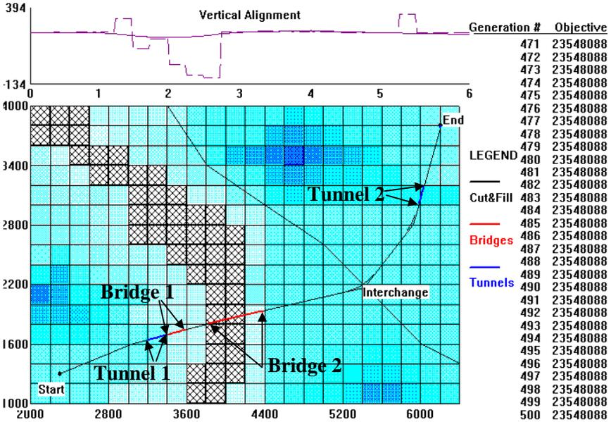
Figure 15.29: Optimized solution, considering a high water constraint and integer numbers of piers.
