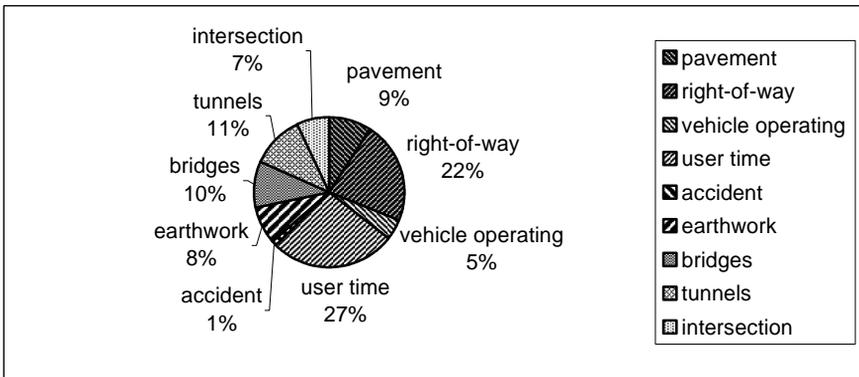
Figure 15.26: Cost breakdown for scenario 2.
