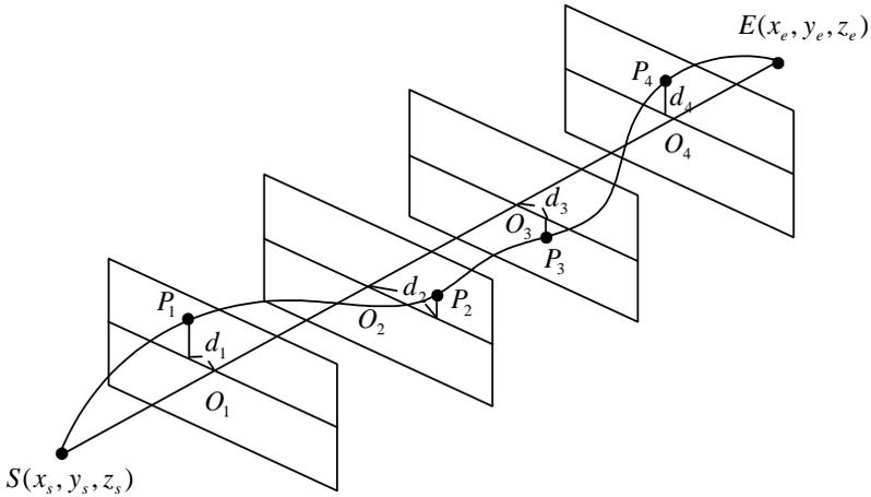
Figure 7.1: The modeling structure for non-backtracking 3-dimensional alignments.
