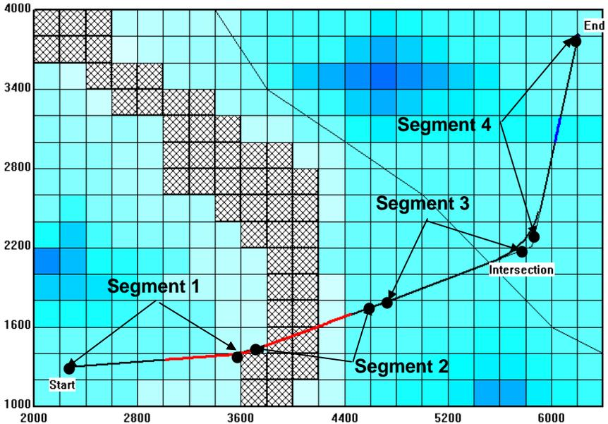
Figure 15.42: Subdividing each segment of the scenario solution 1 for a two-stage optimization.
