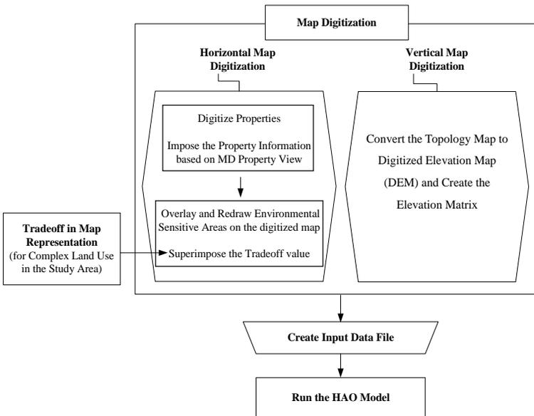
Figure 10.30: Procedure for the HAO model application.
