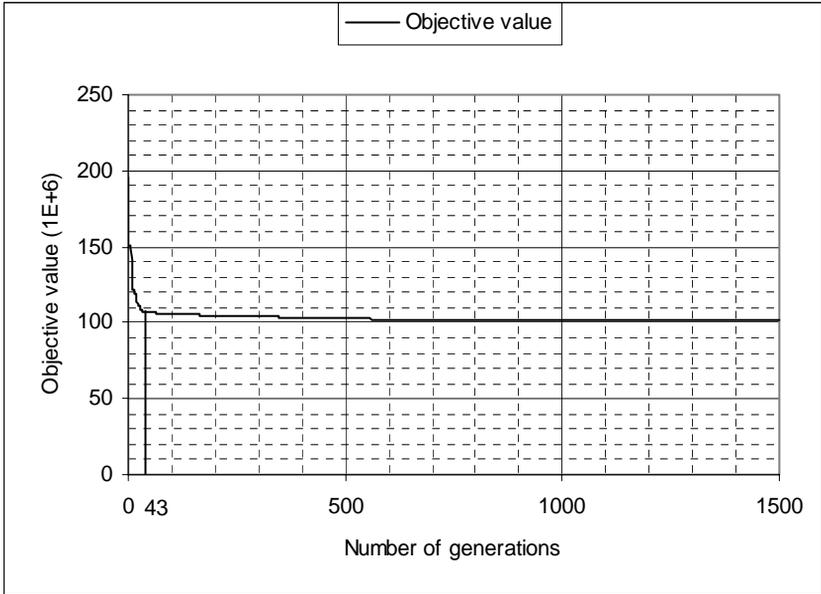
Figure 9.6: Objective value through successive generations for test example 1.
