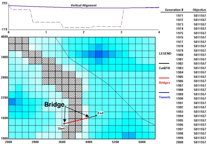
Figure 15.44: Optimized solution for segment 2 under scenario 3.
