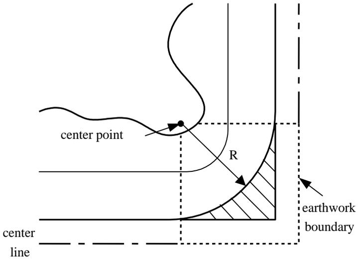
Figure 12.15: A simplified quadrant of a typical fill intersection.
