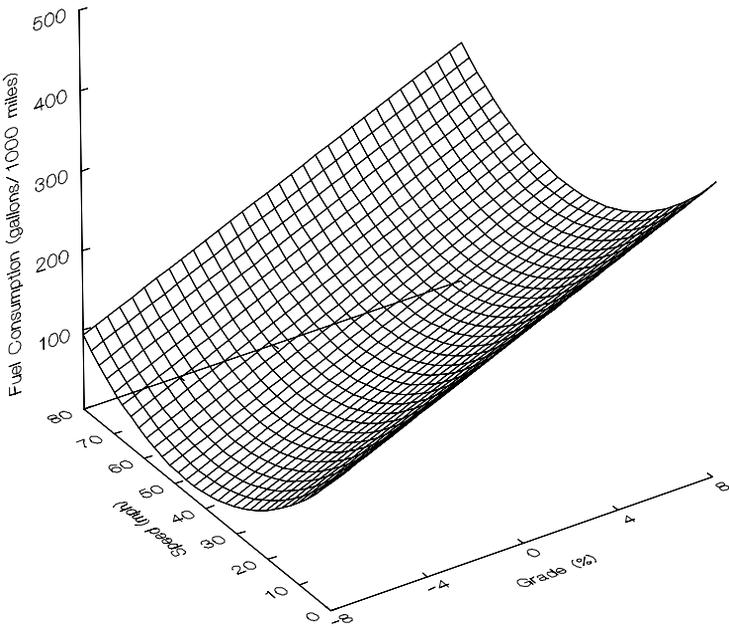
Figure 4.19: Regression function of fuel consumption: 2A-SU truck.
