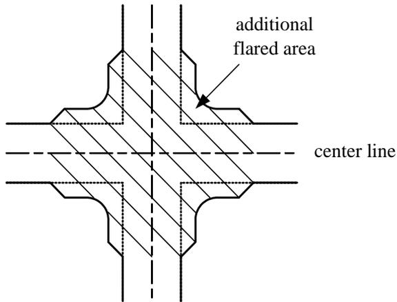
Figure 12.12: A typical four-legged intersection.
