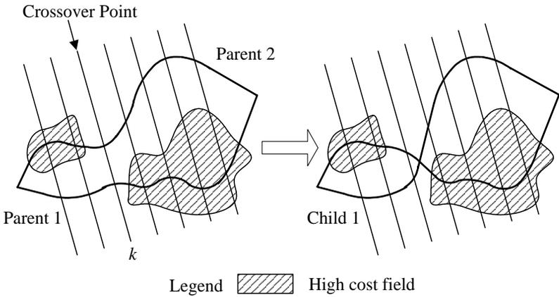
Figure 5.5: An example of a simple crossover operator.
