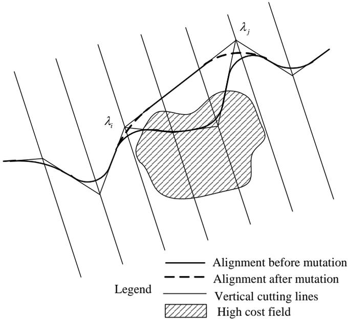
Figure 5.4: An example of a straight mutation operator.
