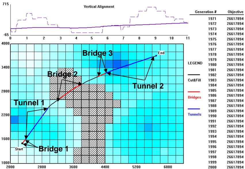
Figure 15.16: Optimized solution (scenario 1) for sensitivity analysis of tunnels.
