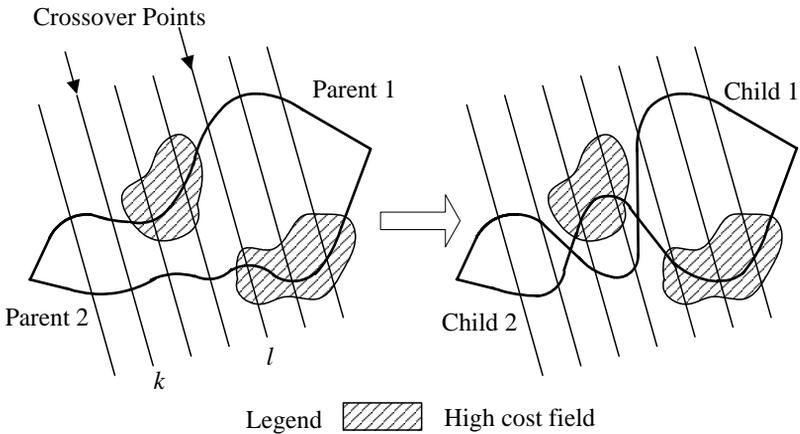
Figure 5.6: An example of a two-point crossover operator.
