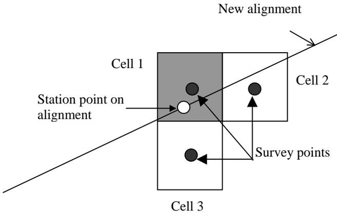
Figure 13.1: A general case for obtaining ground elevations.
