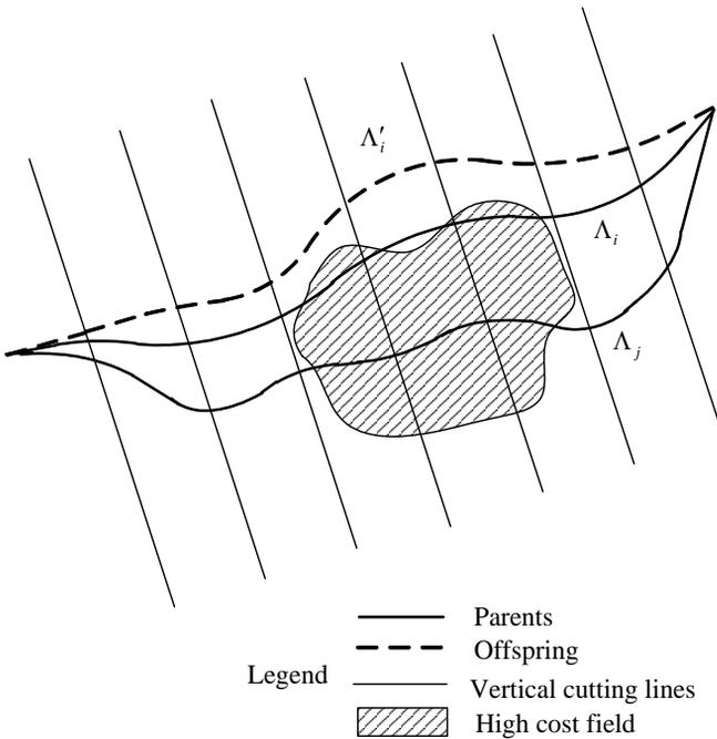
Figure 5.8: An example of a heuristic crossover operator.
