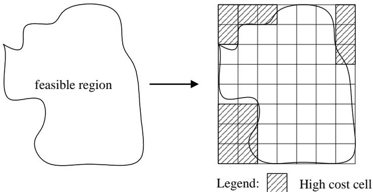
Figure 4.10: The transformation of a non-rectangular shape into a rectangle.
