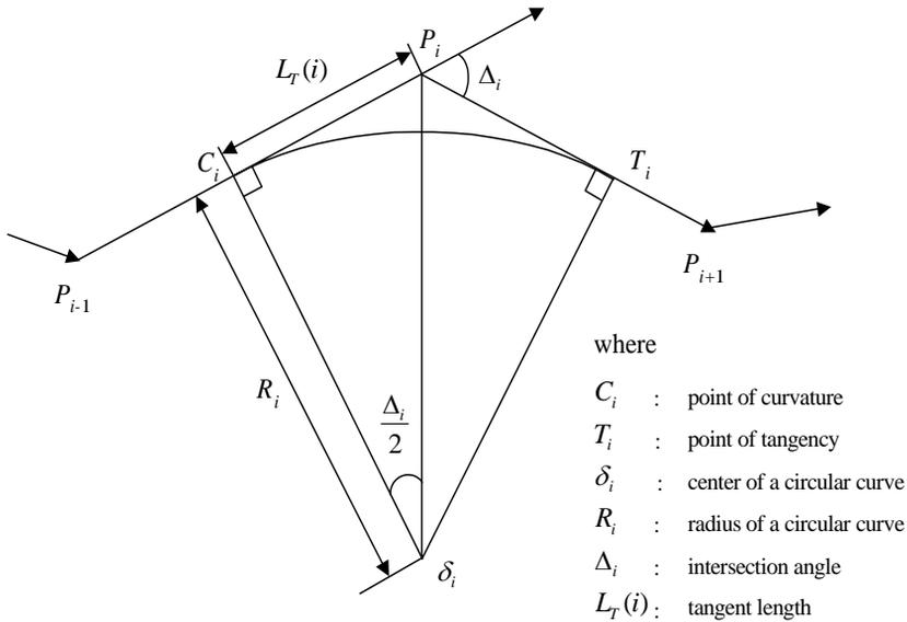
Figure 12.10: Geometric specification of a circular curve.
