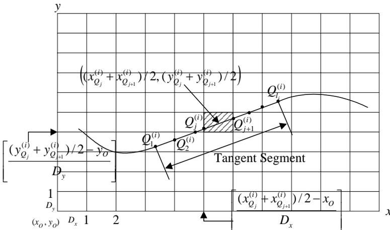
Figure 4.12: Sorted intersection points of a tangent section.
