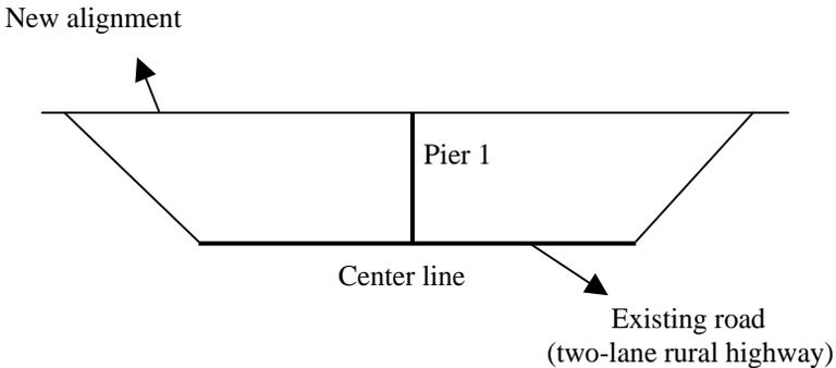
Figure 13.5: A grade separation template for a two-lane rural highway.
