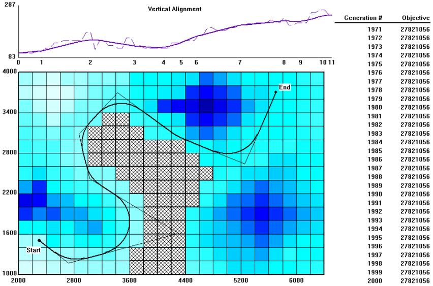
Figure 15.5: Best solution found not incorporating bridges and tunnels for an artificial study area.
