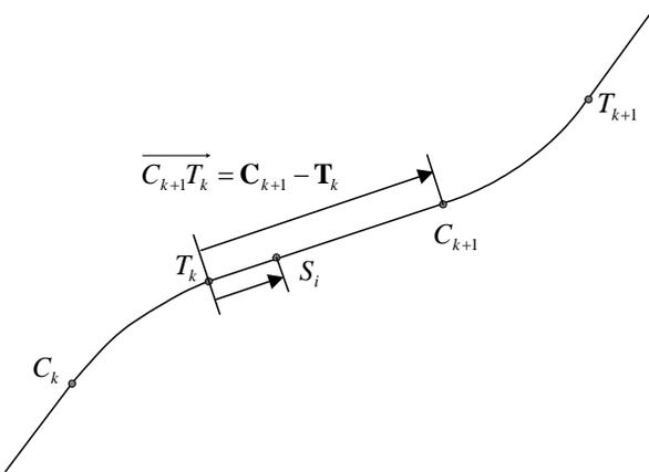
Figure 7.8: Station point on a tangent section of the horizontal alignment.
