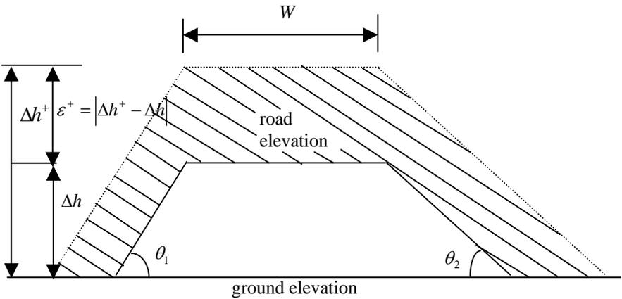
Figure 12.28: Typical cross section with insufficient vertical clearances.
