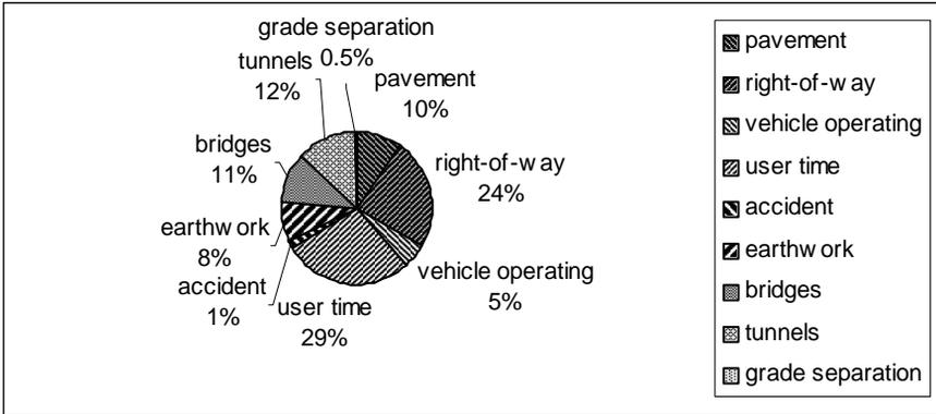
Figure 15.25: Cost breakdown for scenario 1.
