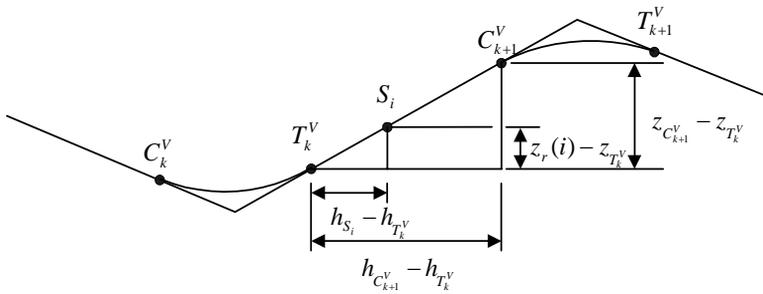
Figure 7.11: Station point on a tangent section of the vertical alignment.
