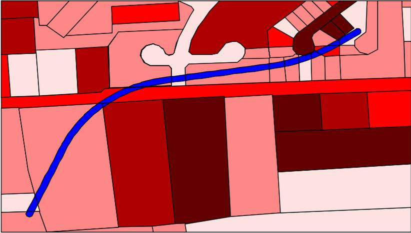
Figure 10.17: Optimized alignment at the 500<sup>th</sup> generation for the Baltimore county case.
