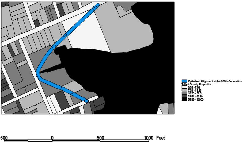
Figure 10.26: Optimized alignment for the Talbot County case obtained at the 100<sup>th</sup> generation.
