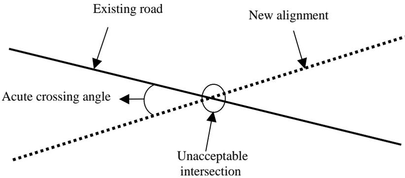
Figure 14.1: Example of intersection with unacceptably acute angle.
