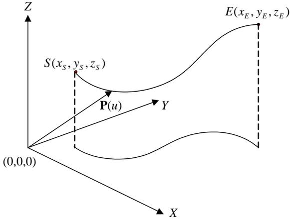
Figure 3.1: The projection of a highway alignment on the  $XY$  plane.
