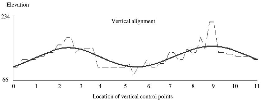
Figure 9.5: The optimized vertical alignment for test example 1.
