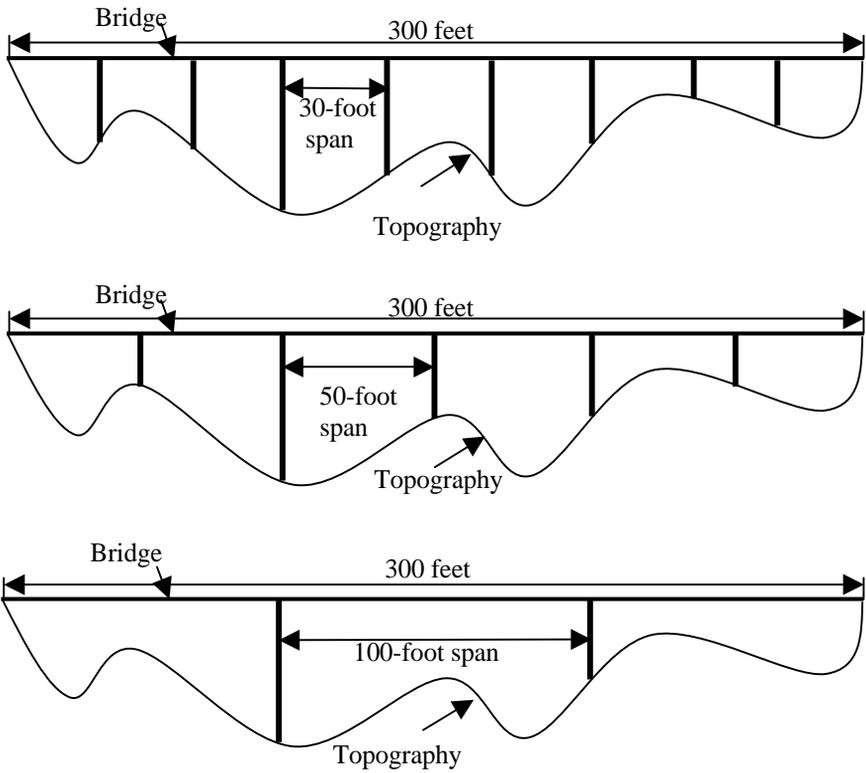
Figure 12.24: Equally spaced piers with varying spans.
