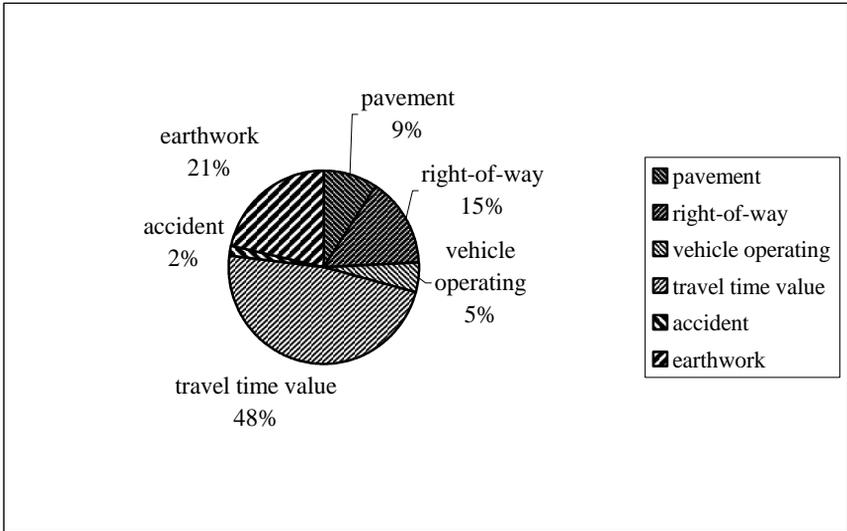
Figure 15.7: Cost breakdown for the alignment in figure 15.5.
