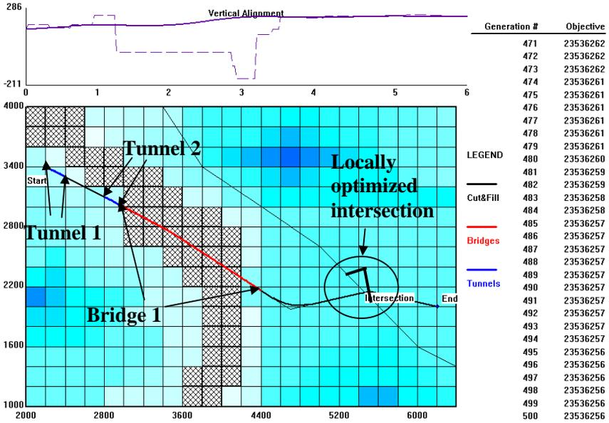
Figure 15.32: The optimized solution involving local intersection optimization with moved start and end points.
