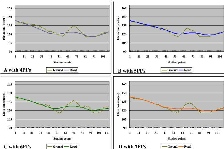
Figure 10.37: Optimized vertical alignments for different PI's.
