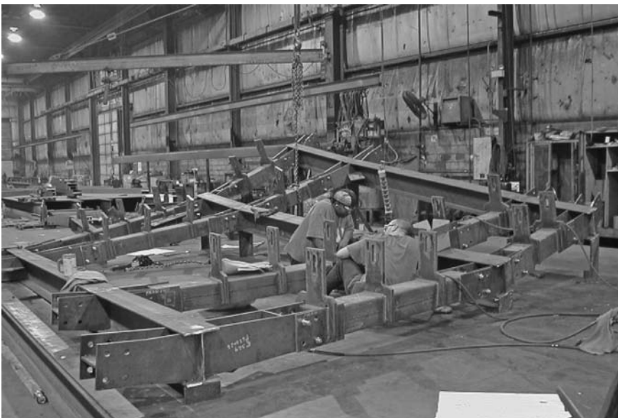
Figure 7.36 Fixture for shop check of subassembly—Millennium Park, Chicago, Illinois.
