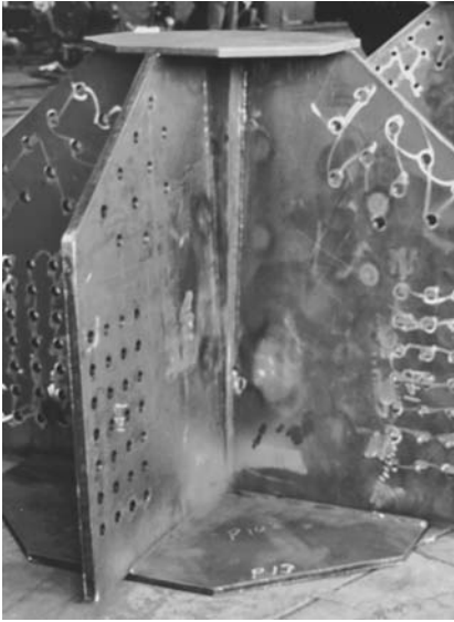
Figure 7.5 Space-frame connector—Carver-Hawkeye Arena, S. E. Geiger—Berger.
