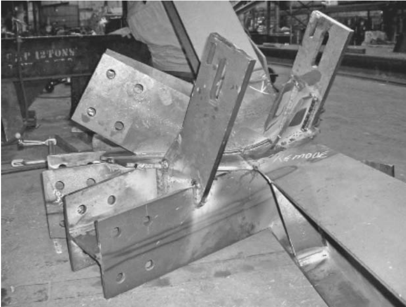
Figure 7.35 Rib connection detail—Millennium Park, Chicago, Illinois.
