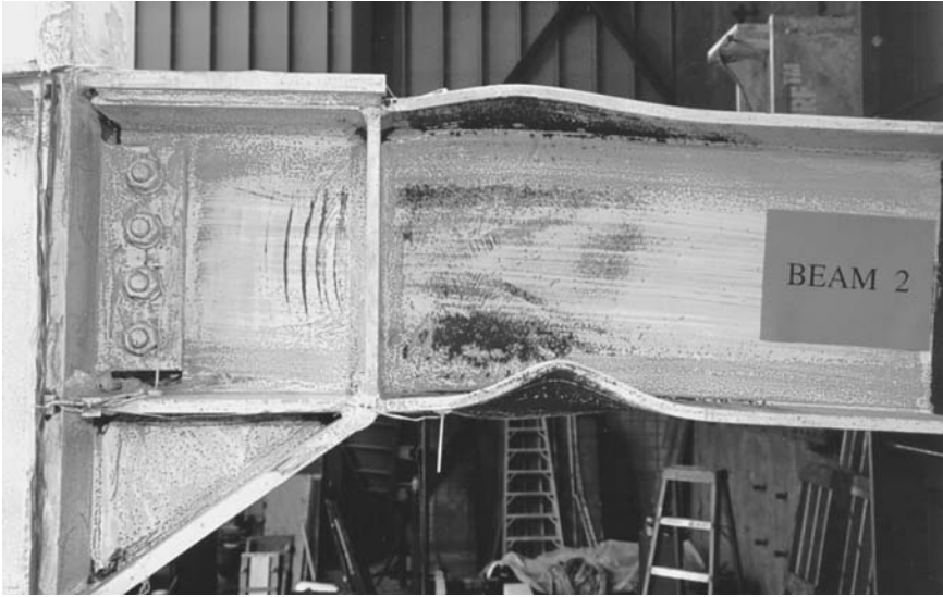
Figure 5.8 Yielding and buckling patterns of a beam subjected to cyclic loading. This connection incorporates both a bottom flange haunch and a top flange cover plate. (Courtesy of Forell/Elsesser Engineers, Inc., San Francisco, CA.)
