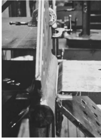
Figure 7.6 Space-frame connector in welding fixture—Carver-Hawkeye Arena.
