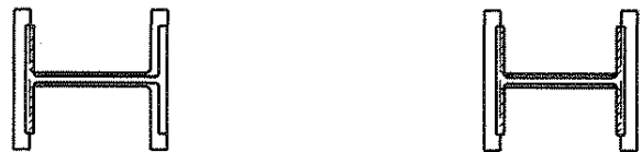
Figure 3-39. Upper and lower column sections not centered, or different nominal sections bearing on each other.
