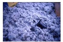
14.26 Loose fill of cellulose fibre.
