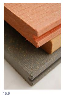
Wood-plastic composite used for cladding, outdoor deck floors, railings and fences. and polyolephines which also quite often include fire retardants. Softeners are, however, not needed in these products. Soft plastic coverings are most often glued to a subfloor of concrete, chipboard, gypsum, etc., usually with an acrylate adhesive or polyvinyl-acetate (PVAC).
