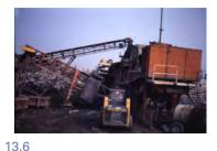
Mobile equipment for producing recycled aggregate.
