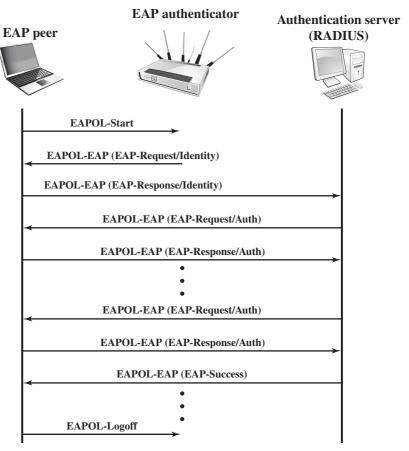
Figure 16.6 Example Timing Diagram for IEEE 802.1X
