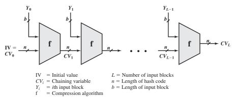
Figure 11.8 General Structure of Secure Hash Code
