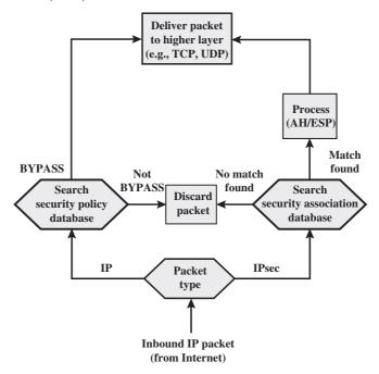
Figure 20.4 Processing Model for Inbound Packets
