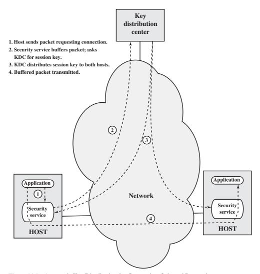
Figure 14.4 Automatic Key Distribution for Connection-Oriented Protocol
