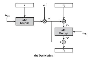
Figure 6.10 XTS-AES Operation on Single Block
