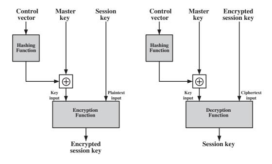
Figure 14.6 Control Vector Encryption and Decryption
