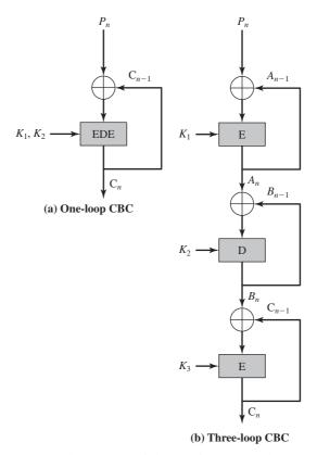
Figure 6.12 Use of Triple DES in CBC Mode
