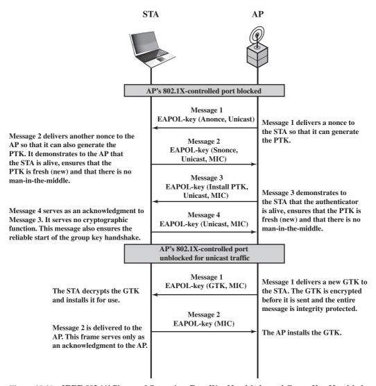
Figure 18.10 IEEE 802.11i Phases of Operation: Four-Way Handshake and Group Key Handshake
