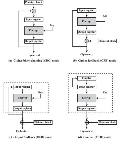
Figure 6.8 Feedback Characteristic of Modes of Operation
