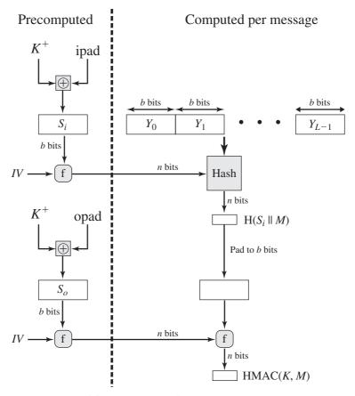
Figure 12.6 Efficient Implementation of HMAC
