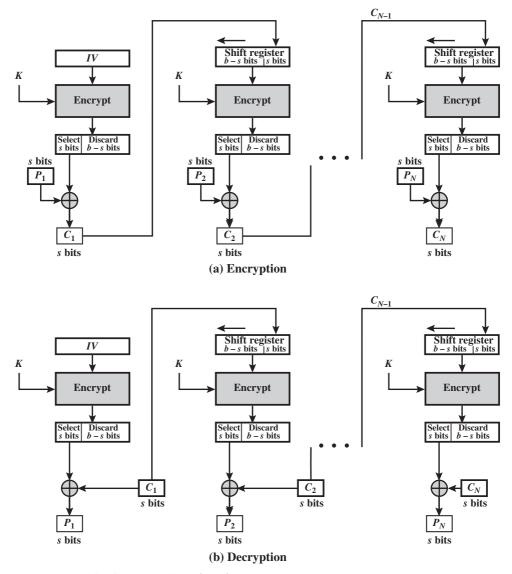
Figure 6.5 s-bit Cipher Feedback (CFB) Mode
