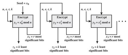
Figure 10.8 Micali-Schnorr Pseudorandom Bit Generator
