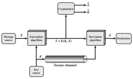
Figure 2.2 Model of Symmetric Cryptosystem
