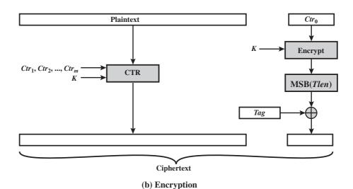
Figure 12.9 Counter with Cipher Block Chaining-Message Authentication Code (CCM)
