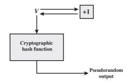
(a) PRNG using cryptographic hash function
