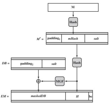
Figure 13.7 RSA-PSS Encoding
