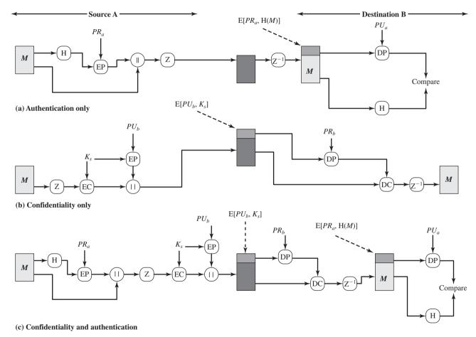
Figure 19.1 PGP Cryptographic Functions
