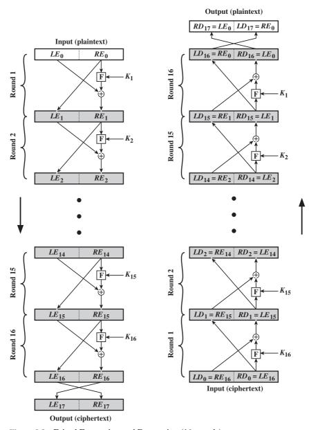
Figure 3.3 Feistel Encryption and Decryption (16 rounds)
