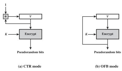
Figure 7.4 PRNG Mechanisms Based on Block Ciphers
