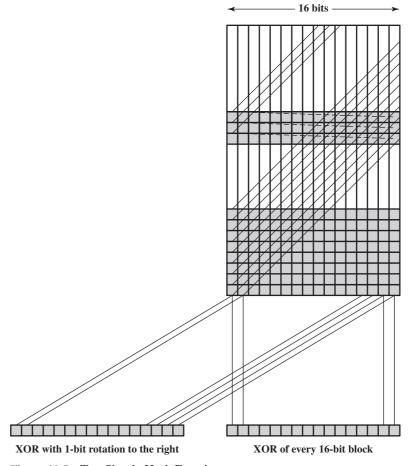
Figure 11.5 Two Simple Hash Functions
