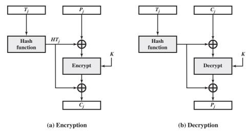
Figure 6.9 Tweakable Block Cipher
