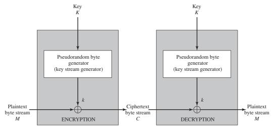
Figure 7.7 Stream Cipher Diagram
