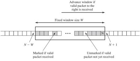
Figure 20.6 Anti-replay Mechanism
