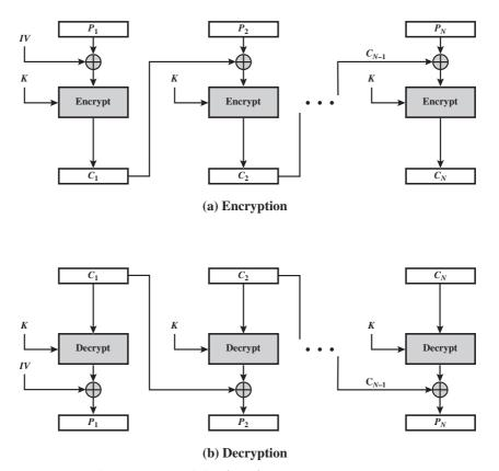
Figure 6.4 Cipher Block Chaining (CBC) Mode
