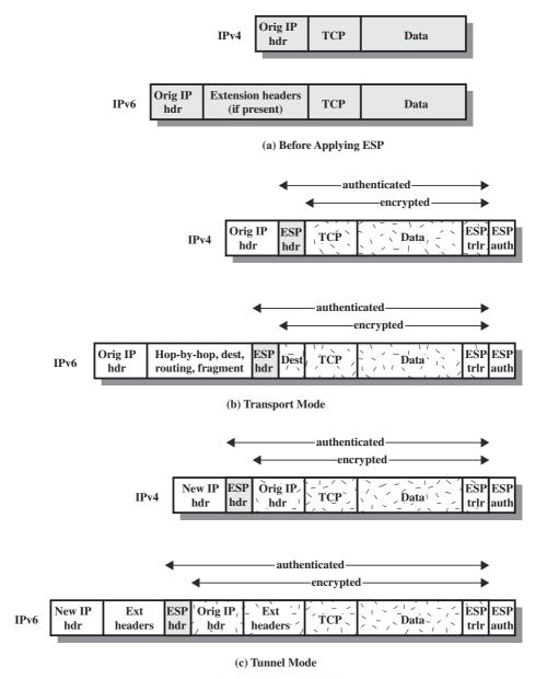
Figure 20.8 Scope of ESP Encryption and Authentication
