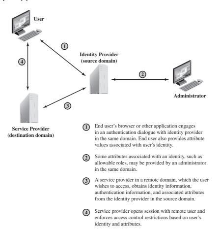
Figure 15.5 Federated Identity Operation
