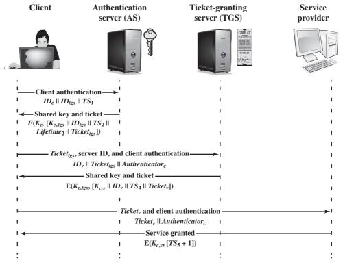
Figure 15.2 Kerberos Exchanges
