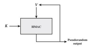
Figure 12.14 Basic Structure of Hash-Based PRNGs (SP 800-90)
