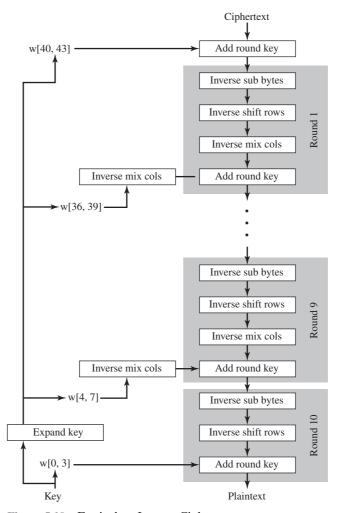
Figure 5.10 Equivalent Inverse Cipher
