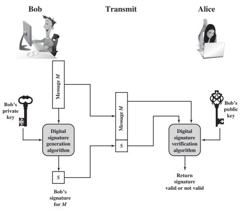
Figure 13.1 Generic Model of Digital Signature Process
