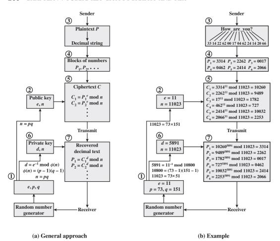
Figure 9.7 RSA Processing of Multiple Blocks
