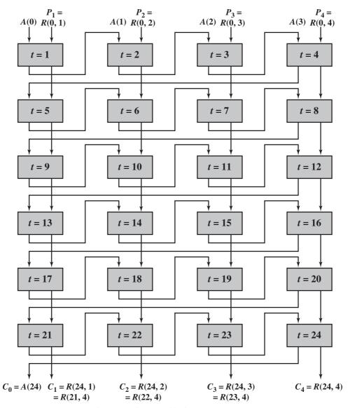
Figure 12.12 Key Wrapping Operation for 256-Bit Key
