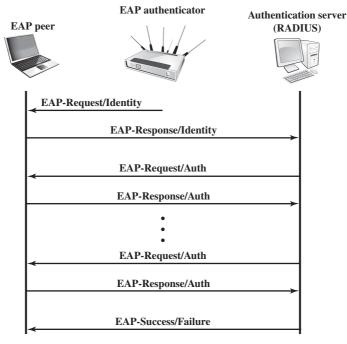
Figure 16.4 EAP Message Flow in Pass-Through Mode
