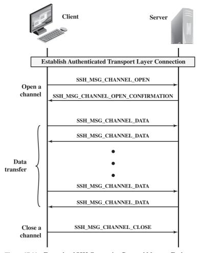
Figure 17.11 Example of SSH Connection Protocol Message Exchange
