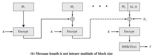
Figure 12.8 Cipher-Based Message Authentication Code (CMAC)
