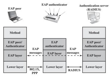
Figure 16.3 EAP Protocol Exchanges
