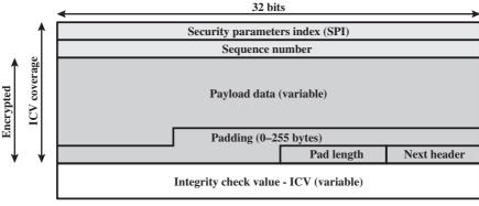
(a) Top-level format of an ESP Packet
