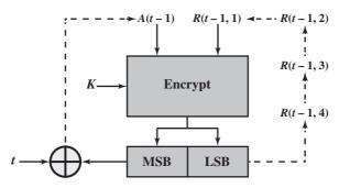
Figure 12.13 Key Wrapping Operation for 256-Bit Key: Stage t
