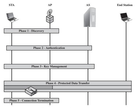
Figure 18.7 IEEE 802.11i Phases of Operation
