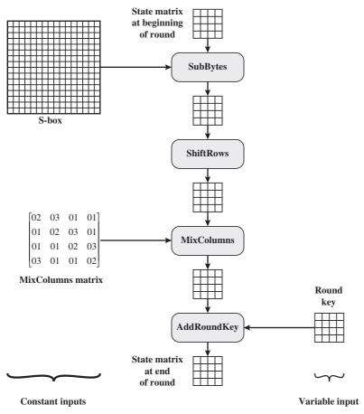
Figure 5.8 Inputs for Single AES Round
