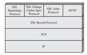
Figure 17.2 SSL Protocol Stack
