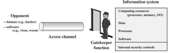
Figure 1.3 Network Access Security Model
