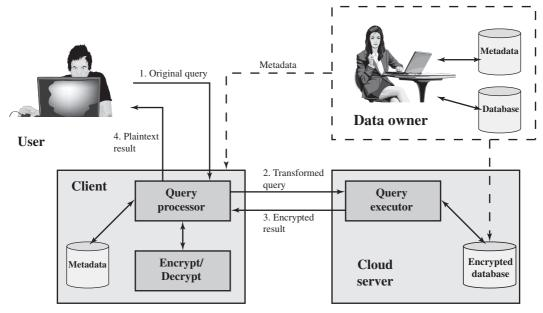
Figure 16.10 An Encryption Scheme for a Cloud-Based Database
