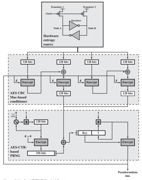
Figure 7.10 Intel DRNG Logical Structure
