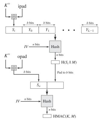
Figure 12.5 HMAC Structure
