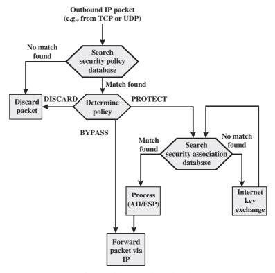
Figure 20.3 Processing Model for Outbound Packets
