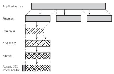
Figure 17.3 SSL Record Protocol Operation
