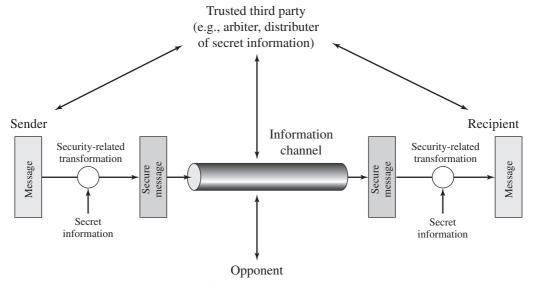
Figure 1.2 Model for Network Security
