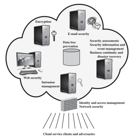
Figure 16.11 Elements of Cloud Security as a Service
