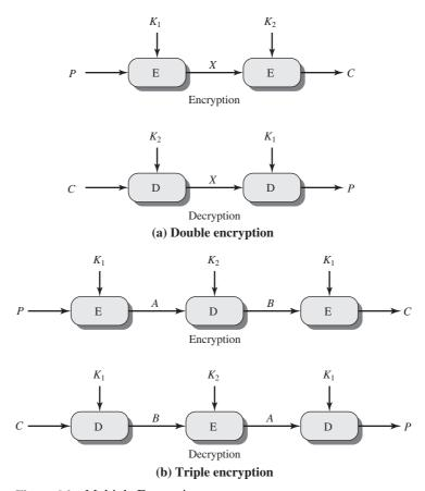
Figure 6.1 Multiple Encryption
