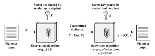
Figure 2.1 Simplified Model of Symmetric Encryption
