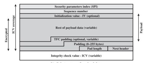
(b) Substructure of payload data
