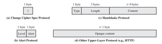
Figure 17.5 SSL Record Protocol Payload
