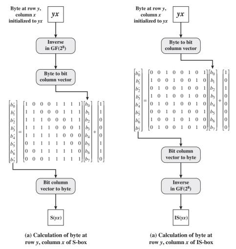
Figure 5.6 Constuction of S-Box and IS-Box
