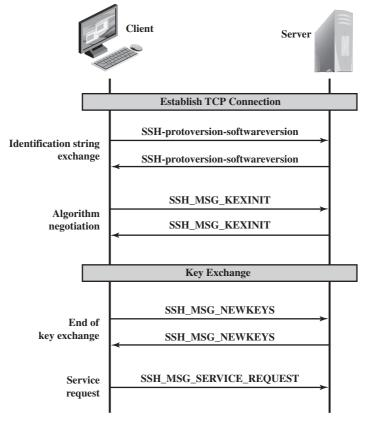
Figure 17.9 SSH Transport Layer Protocol Packet Exchanges
