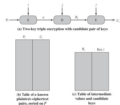
Figure 6.2 Known-Plaintext Attack on Triple DES
