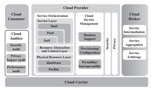
Figure 16.9 NIST Cloud Computing Reference Architecture
