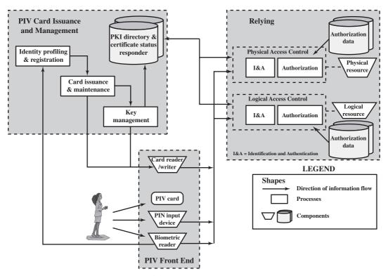
Figure 15.7 FIPS 201 PIV System Model
