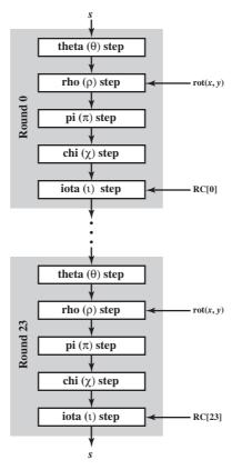
**Figure 11.17** SHA-3 Iteration Function *f*
