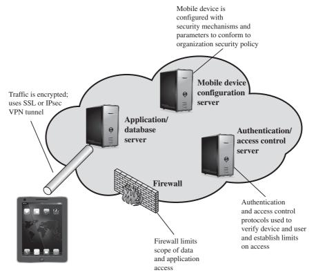
Figure 18.2 Mobile Device Security Elements
