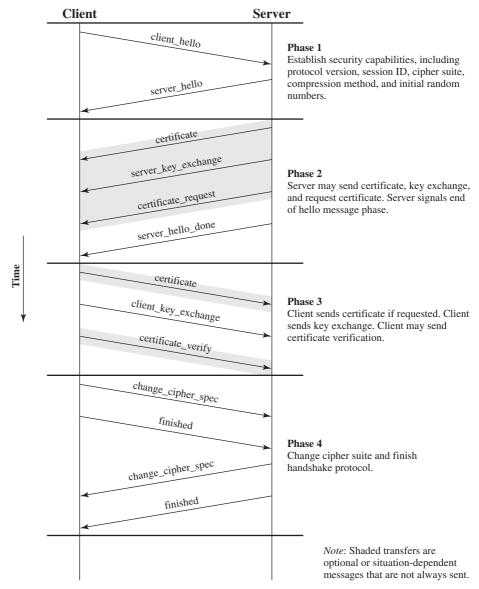
Figure 17.6 Handshake Protocol Action
