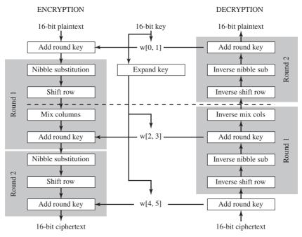
Figure 5.11 S-AES Encryption and Decryption
