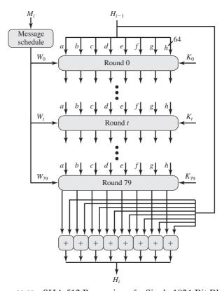
Figure 11.10 SHA-512 Processing of a Single 1024-Bit Block
