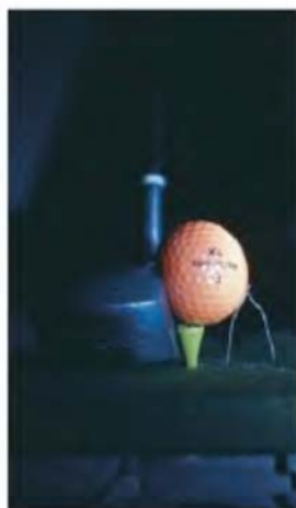
FIGURE 6.4 The force of impact on a golf ball varies throughout the duration of impact.
