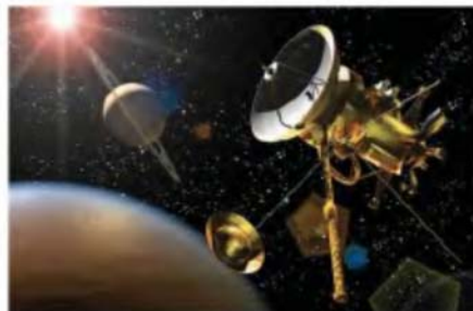
FIGURE 10.35 The European–U.S. spacecraft Cassini beams close-up images of Saturn and its giant moon Titan to Earth. It also measures surface temperatures, magnetic fields, and the size, speed, and trajectories of tiny surrounding space particles.
