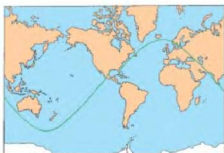
FIGURE A The path of a typical satellite launched in a northeasterly direction from Cape Canaveral. Because Earth rotates while the satellite orbits, each sweep passes overhead some 2100 km farther west at the latitude of Cape Canaveral.
