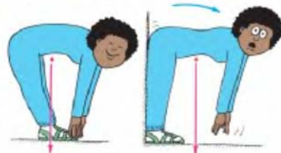
FIGURE 8.31 You can lean over and touch your toes without falling over only if your center of gravity is above the area bounded by your feet.
