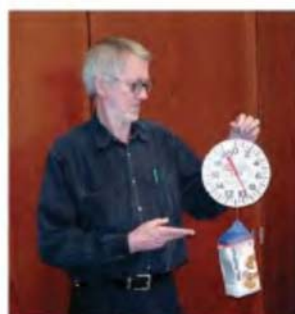
FIGURE 2.7 Burl Grey, who first introduced the author to tension forces, suspends a 2-lb bag of flour from a spring scale, showing its weight and the tension in the string of about 9 N.
