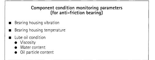
Figure 3.6 Component condition monitoring parameters (for anti-friction bearing)
