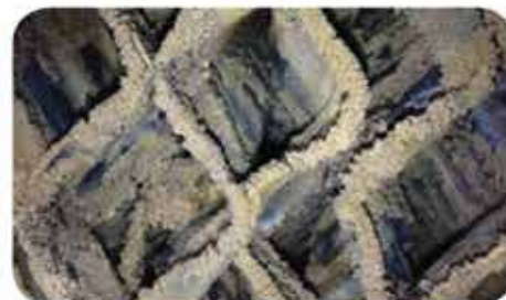
Scale embedded in biofilm on tower pack
