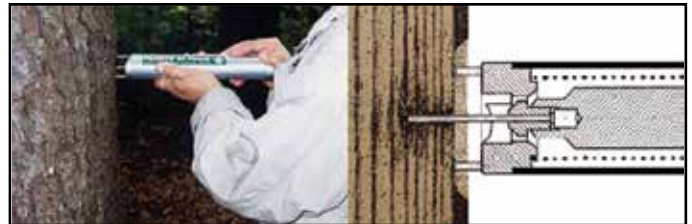
Figure 8: Pilodyn Test Method for Wood Density and Strength
