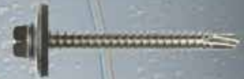
Self-Drilling Hex-Washer Head Screw Type 305 and 316 stainless steel with EPDM sealing washer
