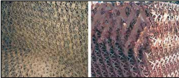
Figure 16: Two different fouled CFTF packs from field installations.
