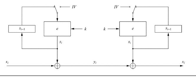
**Encryption (first block):**  $s_1 = e_k(IV)$  and  $y_1 = s_1 \bigoplus x_1$  **Encryption (general block):**  $s_i = e_k(s_{i-1})$  and  $y_i = s_i \bigoplus x_i$ ,  $i \ge 2$  **Decryption (first block):**  $s_1 = e_k(IV)$  and  $x_1 = s_1 \bigoplus y_1$ **Decryption (general block):**  $s_i = e_k(s_{i-1})$  and  $x_i = s_i \bigoplus y_i$ ,  $i \ge 2$
