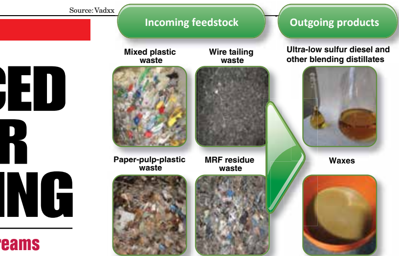
FIGURE 1. The main products from the Vadxx process are diesel additives and wax, with feedstock from sources like materials-recovery facilities (MRF) and paper-processing plants
