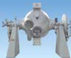
Eccentric agitator with two independent movements
