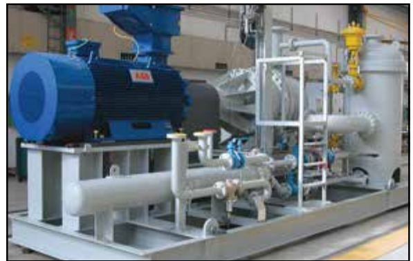
This two-stage liquid-ring compressor handles 2,500 m 3 /h of flare gas at 7.5 bar. Skid-mounted packages like this form an increasingly important business area for the Pompetravaini Group.
