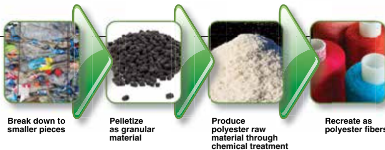
FIGURE 3. The proprietary chemical process behind Teijin's Eco Circle technology creates recycled polyester fibers that are of equal quality to polyester produced from all-new materials
