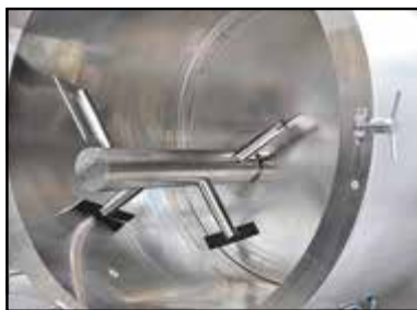
The small diameter of the Planex System agitator reduces thermal stress without compromising drying performance
