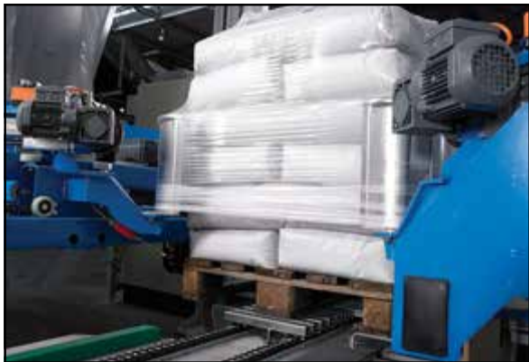
The BEUMER stretch hood packaging machine secures goods on the pallet, minimizes film consumption and protects the product
