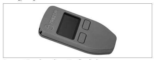
*Figure 5-4. A Trezor device: a bitcoin HD wallet in hardware*
