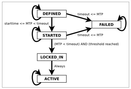
Figure 10-10. BIP-9 state transition diagram
