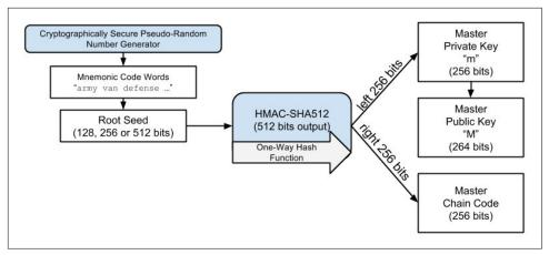
Figure 5-9. Creating master keys and chain code from a root seed
