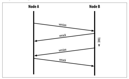
Figure 8-4. The initial handshake between peers
