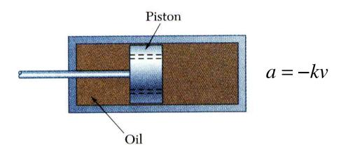
Brake mechanism used to reduce gun recoil consists of piston attached to barrel moving in fixed cylinder filled with oil. As barrel recoils with initial velocity  $v_0$ , piston moves and oil is forced through orifices in piston, causing piston and cylinder to decelerate at rate proportional to their velocity.
