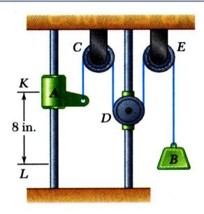
Pulley D is attached to a collar which is pulled down at 3 in./s. At t = 0, collar A starts moving down from K with constant acceleration and zero initial velocity. Knowing that velocity of collar A is 12 in./s as it passes L, determine the change in elevation, velocity, and acceleration of block B when block A is at L.
