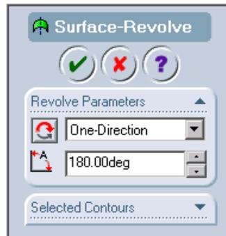
Figure 15-6 The Surface-Revolve PropertyManager
