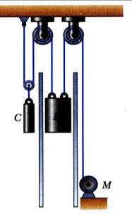
The dumbwaiter D and its load have a combined weight of 300 kg, while the counterweight C weighs 400 kg.
