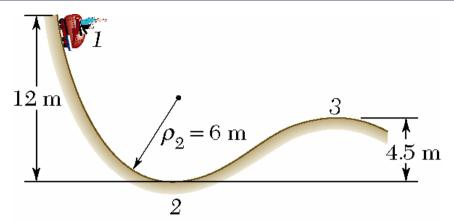
A 1000 kg car starts from rest at point 1 and moves without friction down the track shown.
