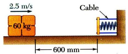
A spring is used to stop a 60 kg package which is sliding on a horizontal surface. The spring has a constant k = 20 kN/m and is held by cables so that it is initially compressed 120 mm. The package has a velocity of 2.5 m/s in the position shown and the maximum deflection of the spring is 40 mm.
