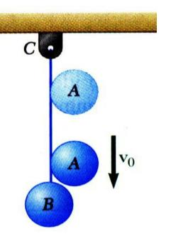
Ball *B* is hanging from an inextensible cord. An identical ball *A* is released from rest when it is just touching the cord and acquires a velocity  $v_0$  before striking ball *B*. Assuming perfectly elastic impact ( $e = \bullet$ 1) and no friction, determine the velocity of each ball immediately after impact.
