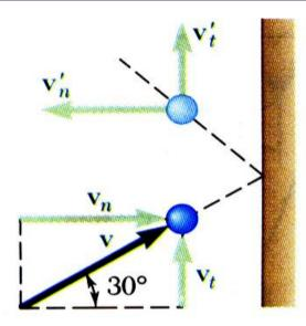
A ball is thrown against a frictionless, vertical wall. Immediately before the ball strikes the wall, its velocity has a magnitude v and forms angle of 30° with the horizontal. Knowing that e = 0.90, determine the magnitude and direction of the velocity of the ball as it rebounds from the wall.
