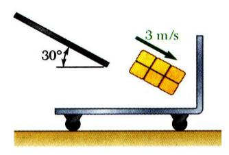
A 10 kg package drops from a chute into a 24 kg cart with a velocity of 3 m/s. Knowing that the cart is initially at rest and can roll freely, determine (a) the final velocity of the cart, (b) the impulse exerted by the cart on the package, and (c) the fraction of the initial energy lost in the impact.
