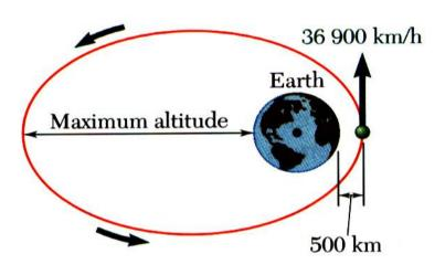
A satellite is launched in a direction parallel to the surface of the earth with a velocity of 36900 km/h from an altitude • of 500 km.
