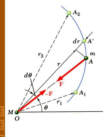
Work of a gravitational force (assume particle *M* occupies fixed position *O* while particle *m* follows path shown),
