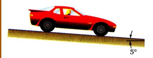
An automobile weighing 1800 kg is driven down a 5° incline at a speed of 100 km/h when the brakes are applied, causing a constant total braking force of 6.5 kN.
