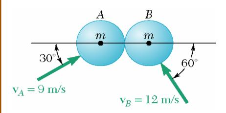
The magnitude and direction of the velocities of two identical frictionless balls before they strike each other are as shown. Assuming e = 0.9, determine the magnitude and direction of the velocity of each ball after the impact.
