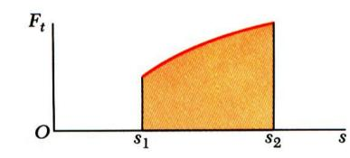
Mc Tav • Work is represented by the area under the curve of *F<sub>t</sub>* plotted against *s*.
