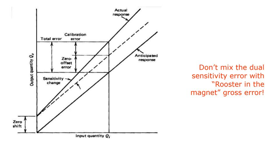
Here, due to change in temperature we got both the offset change and the change in the sensitivity (calibration and offset errors)
