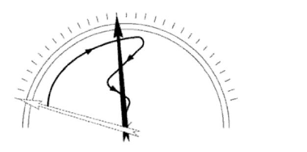
Figure 3.3. The movement of the pointer after connection of the device to the measured current
