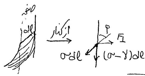
$$\sum F_{11} = 0 \Rightarrow \sigma dl \cos \varphi + (\sigma - \gamma) dl = 0 \Rightarrow \cos \varphi = \frac{\gamma - \sigma}{\sigma} \Rightarrow \varphi = \cos^{-1} \left( \frac{\gamma}{\sigma} - 1 \right)$$
