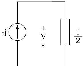
$$Z_c \parallel Z'_L \parallel R \rightarrow (-j) \parallel \left(\frac{1+j}{2}\right) \parallel (1) = \frac{1}{2}$$
