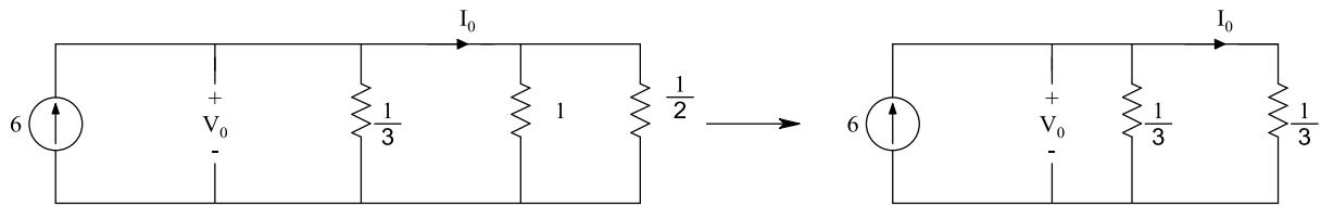
$$I_0 = \frac{\frac{1}{3}}{\frac{1}{3} + \frac{1}{3}} = \frac{\frac{1}{3}}{\frac{2}{3}} \times 6 = 3 \quad , \quad V_0 = 3 \times \frac{1}{3} = 1$$
