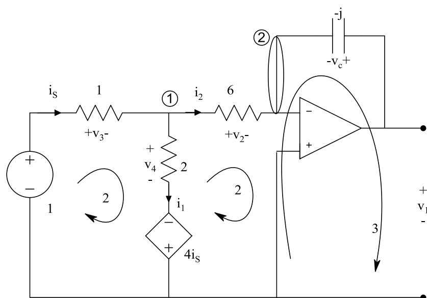
$$\text{Kcl 1: } i_s = i_1 + i_2 \rightarrow v_3 = \frac{v_4}{2} + \frac{v_2}{6} \quad (1)$$
