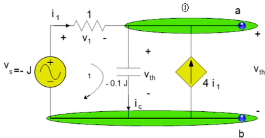
$$kcl \ 1: i_1 + 4i_1 = i_c \rightarrow 5i_1 = i_c \rightarrow 5v_1 = \frac{V_{th}}{-0/1j} = 10jv_{th} \rightarrow v_1 = 2jv_{th} \quad (1)$$
