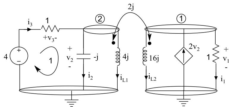
$$\text{Kcl 1: } 2v_2 = i_1 + i_{L2} \rightarrow -2ji_2 = i_1 + i_{L2} \quad (1)$$
