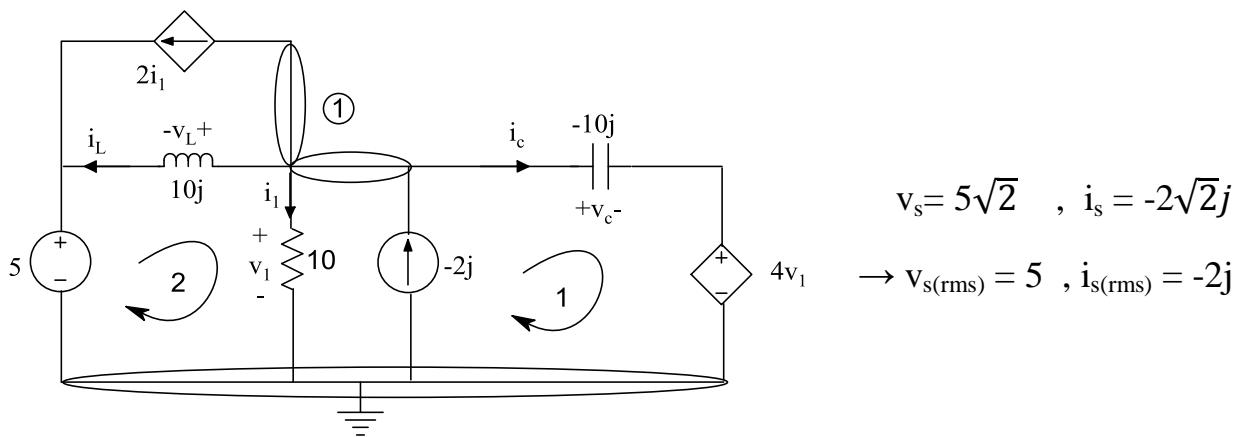
$$\text{Kcl 1: } -2j = i_c + i_L + 3i_1 \rightarrow -2j = \frac{1}{10}jv_c - \frac{1}{10}jv_L + \frac{3}{10}v_1 \quad (1)$$
