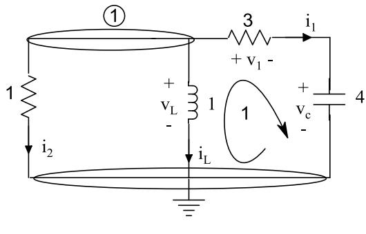
$$\text{Kcl 1: } i_1 + i_2 + i_L = 0 \quad (1)$$
