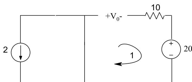
$$\text{Kvl 1: } V_0 + 20 = 0 \rightarrow V_0 = -20$$
