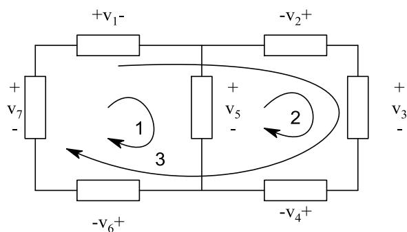
$$\text{KVL 1: } V_1 + V_5 + V_6 - V_7 = 0$$
