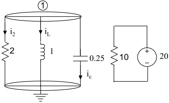
$$\text{Kcl 1: } i_c + i_L + i_2 = 0 \quad (1)$$
