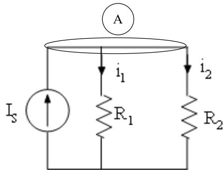
$$i_1 = \frac{R_2}{R_1 + R_2} \times I_S \quad , \quad i_2 = \frac{R_1}{R_1 + R_2} \times I_S$$
