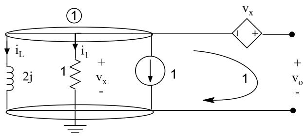
$$KCl 1: i_L + i_1 + 1 = 0 \rightarrow \frac{v_x}{2j} + v_x + 1 = 0 \rightarrow v_x = \frac{-4}{5} - \frac{2}{5} j$$
