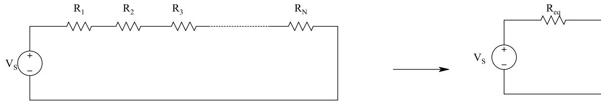
$$R_{eq} = R_1 + R_2 + R_3 + \dots + R_N$$
