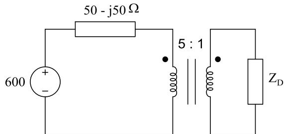
$$\frac{V_{S2}}{V_{S3}} = 5 \rightarrow V_{S3} = \frac{600}{5} = 120$$
