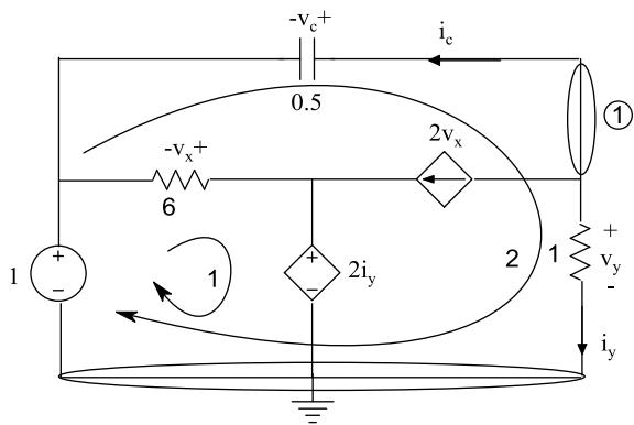
$$\text{Kcl 1: } i_c + 2v_x + i_y = 0 \rightarrow 0/5 \frac{dv_c}{dt} + 2v_x + v_y = 0 \quad (1)$$
