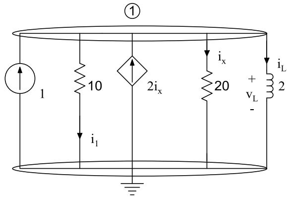
$$\text{Kcl } I: 2i_x + I = i_x + i_L + i_I \rightarrow i_x + I = i_L + i_I \quad (I)$$
