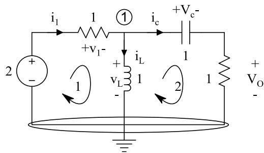
$$\text{Kcl 1: } i_1 = i_L + i_c \rightarrow v_1 = \int_{-\infty}^t v_L(t) dt + \frac{dv_c}{dt} \quad (1)$$
