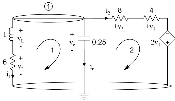
$$\text{Kcl 1: } i_1 + i_c + i_2 = 0 \rightarrow \frac{v_2}{6} + \frac{1}{4} \frac{dv_c}{dt} + \frac{v_1}{4} = 0 \quad (1)$$
