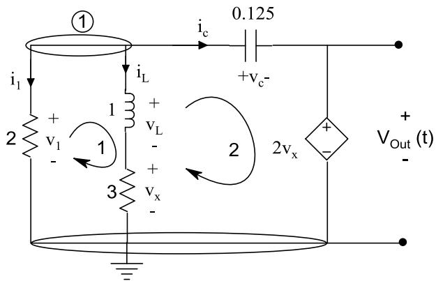
$$\text{Kcl 1: } i_1 + i_L + i_c = 0 \rightarrow \frac{v_1}{2} + \frac{v_x}{3} + 0/125 \frac{dv_c}{dt} = 0 \quad (1)$$
