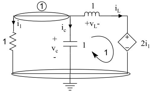
$$\text{Kcl 1: } i_1 + i_c + i_L = 0 \rightarrow v_c + \frac{dv_c}{dt} + \int_{-\infty}^t v_L(t) dt = 0 \quad (1)$$
