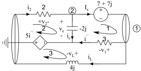
$$\begin{aligned} V_s &= 7\sqrt{2} e^{j45^\circ} = 7\sqrt{2} (\cos 45^\circ + j \sin 45^\circ) \\ &= 7\sqrt{2} \left( \frac{\sqrt{2}}{2} + j \frac{\sqrt{2}}{2} \right) = 7 + 7j \end{aligned}$$
