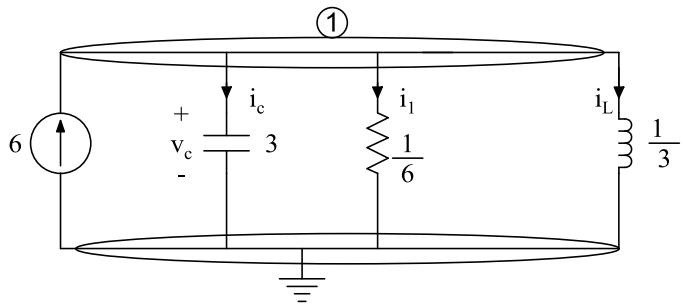
$$\text{KCl 1: } i_c + i_1 + i_L = 6 \rightarrow 3 \frac{dv_c}{dt} + 6v_c + 3 \int_{-\infty}^t v_c(t) dt = 6$$
