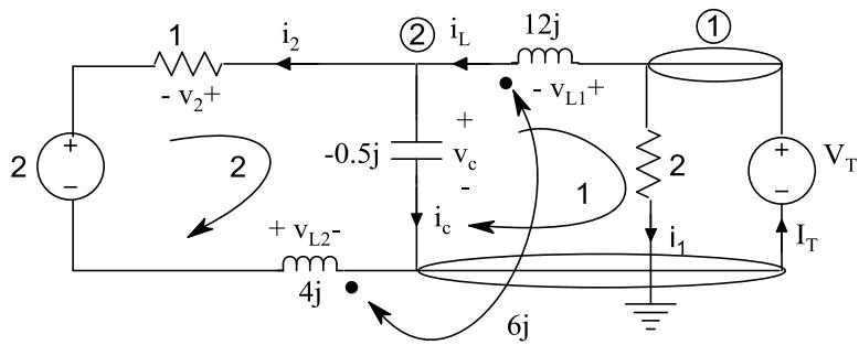
$$\text{Kcl 1: } I_T = i_1 + i_L \rightarrow I_T = \frac{V_T}{2} + i_L \quad (1)$$
