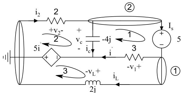
$$\text{Kvl 1: } 5 + v_1 - v_c = 0 \rightarrow 5 + 3i' + 4ji_c = 0 \quad (1)$$
