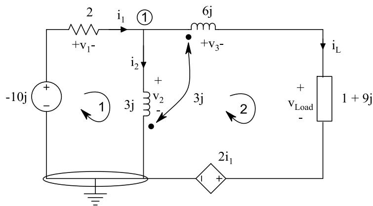
$$\text{Kcl 1: } i_1 = i_L + i_2 \quad (1)$$
