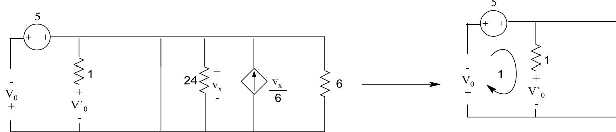
$$KVL 1: 5 + V'_0 + V_0 = 0 \rightarrow -V'_0 - V_0 = 5$$
