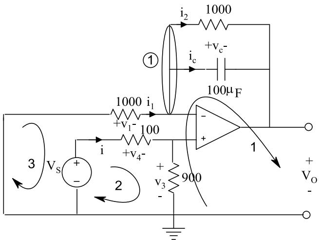
$$KCl 1: i_1 = i_2 + i_c \rightarrow \frac{v_1}{1000} = \frac{v_c}{1000} + 10^{-4} \frac{dv_c}{dt} \rightarrow v_1 = v_c + 0/1 \frac{dv_c}{dt} \quad (1)$$
