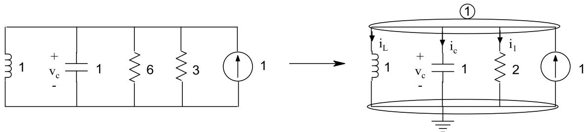
$$\text{Kcl 1: } i_1 + i_c + i_L = 1 \rightarrow \frac{v_c}{2} + \frac{dv_c}{dt} + \int_{-\infty}^t v_c(t) dt = 1 \rightarrow \frac{d^2v_c}{dt^2} + \frac{1}{2} \frac{dv_c}{dt} + v_c = 0$$
