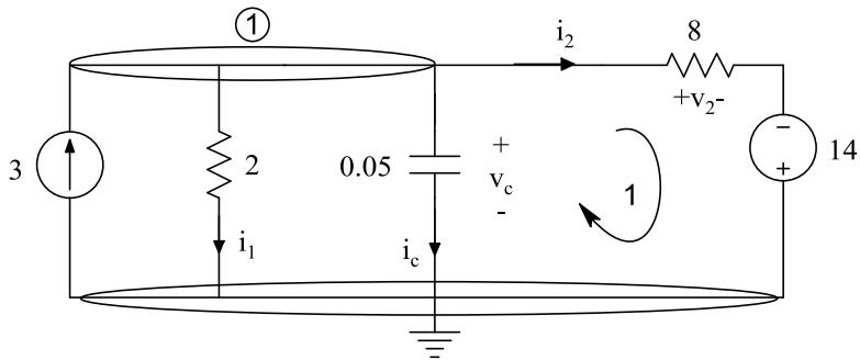
$$KCL 1: 3 = i_1 + i_c + i_2 \rightarrow 3 = \frac{v_c}{2} + 0/05 \frac{dv_c}{dt} + \frac{v_2}{8} \quad (1)$$
