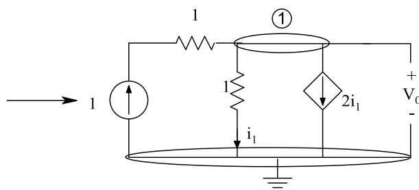
$$KCl 1: 1 = i_1 + 2i_1 = 3i_1 \rightarrow i_1 = \frac{1}{3} \rightarrow V_0 = \frac{1}{3}$$
