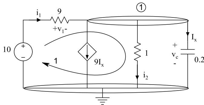
$$\text{Kcl 1: } i_1 = 9I_x + i_2 + I_x \rightarrow i_1 = 10I_x + i_2 \rightarrow \frac{v_1}{9} = 2 \frac{dv_c}{dt} + v_c \quad (1)$$
