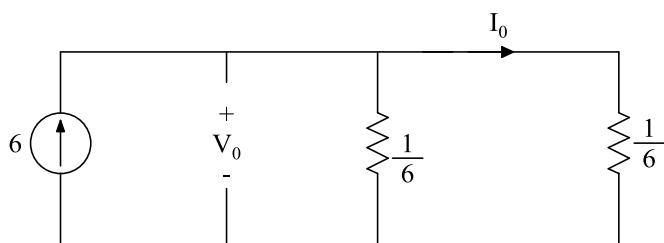
$$I_0 = \frac{\frac{1}{6}}{\frac{1}{6} + \frac{1}{6}} \times 6 = \frac{1}{2} \times 6 = 3 \quad , \quad V_0 = 3 \times \frac{1}{6} = \frac{1}{2}$$
