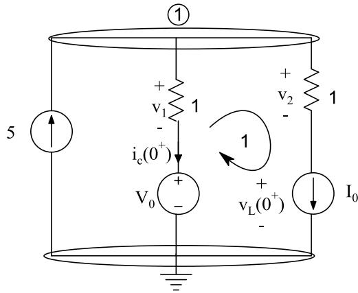
$$\text{Kcl 1: } 5 = i_c(0^+) + I_0 \xrightarrow{I_0=0} i_c(0^+) = v_1 = 5$$
