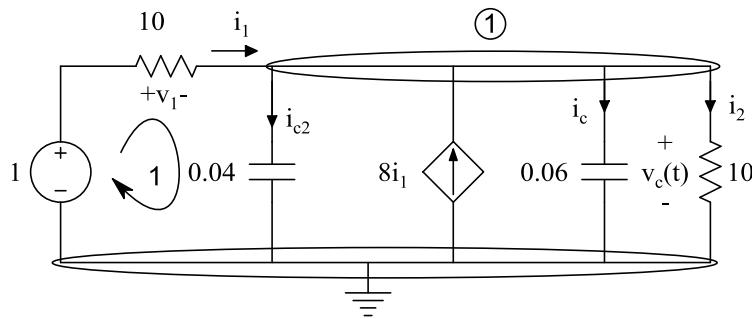
$$KCL 1: 9i_1 = i_c + i_{c2} + i_2 \rightarrow \frac{9}{10}v_1 = 0/04 \frac{dv_c}{dt} + 0/06 \frac{dv_c}{dt} + \frac{v_c}{10}$$
