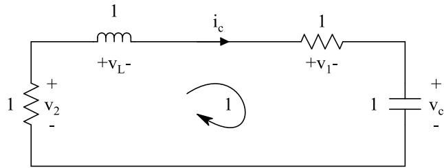
$$\text{Kvl 1: } v_L + v_1 + v_c - v_2 = 0 \quad (1)$$
