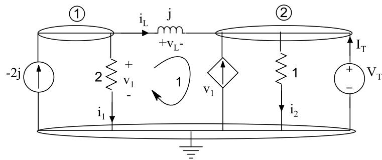
$$\text{Kcl 1: } -2j = i_1 + i_L \rightarrow -2j = \frac{v_1}{2} + \left(\frac{v_L}{j}\right) \quad (1)$$
