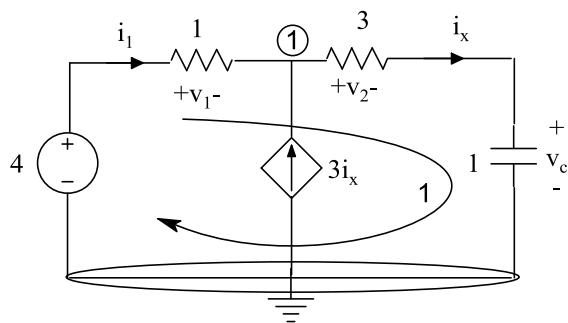
$$\text{KCL 1: } i_1 + 3i_x = i_x \rightarrow i_1 + 2i_x = 0 \rightarrow v_1 + 2 \frac{dvc}{dt} = 0 \quad (1)$$
