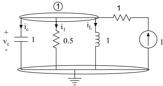
$$\text{KCL 1: } 1 = i_c + i_1 + i_L \rightarrow 1 = \frac{dv_c}{dt} + 2v_c + \int_{-\infty}^t v_c(t) dt \rightarrow \frac{d^2v_c}{dt^2} + 2 \frac{dv_c}{dt} + v_c = 0$$
