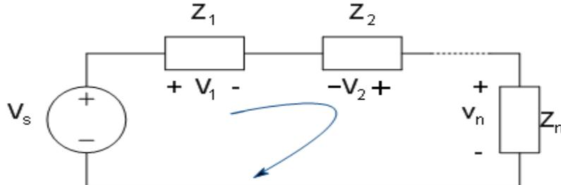
$$v_k = \frac{z_k}{(z_1 + z_2 + \dots + z_n)} v_s \quad (k = 1, 2, \dots, n)$$
