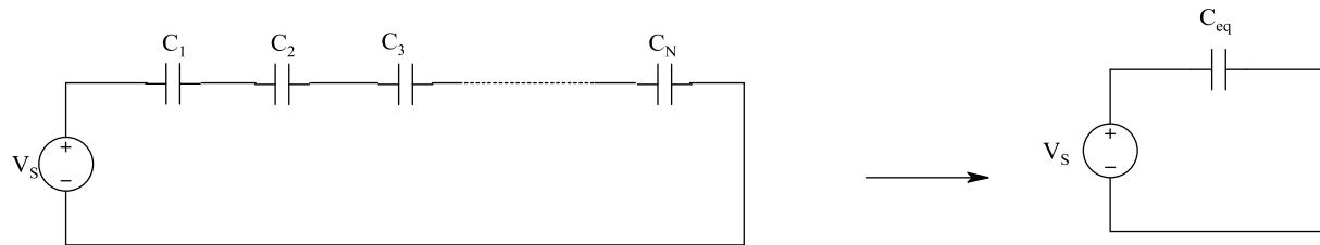
$$\frac{1}{C_{eq}} = \frac{1}{C_1} + \frac{1}{C_2} + \frac{1}{C_3} + \dots + \frac{1}{C_N}$$
