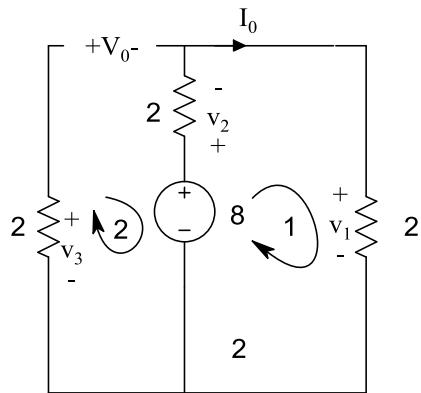
$$\text{Kvl 1: } v_1 - 8 + v_2 = 0$$
