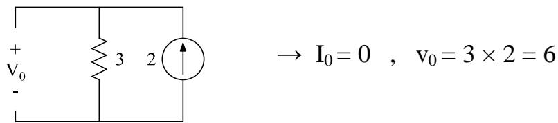
$$\rightarrow I_0 = 0, \quad v_0 = 3 \times 2 = 6$$
