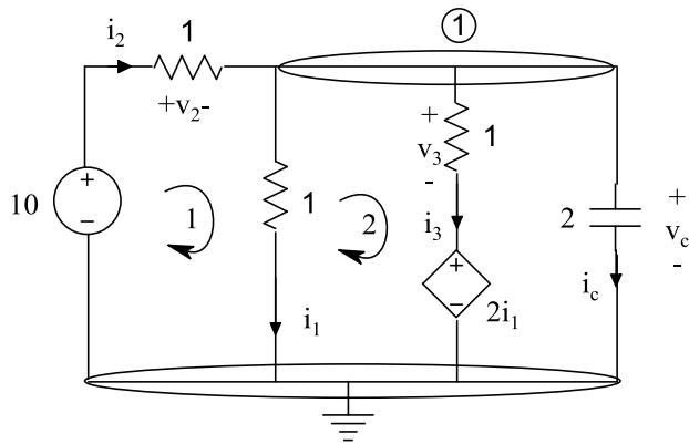
$$\text{Kcl 1: } i_2 = i_1 + i_3 + i_c \rightarrow v_2 = v_c + v_3 + 2 \frac{dv_c}{dt} \quad (1)$$
