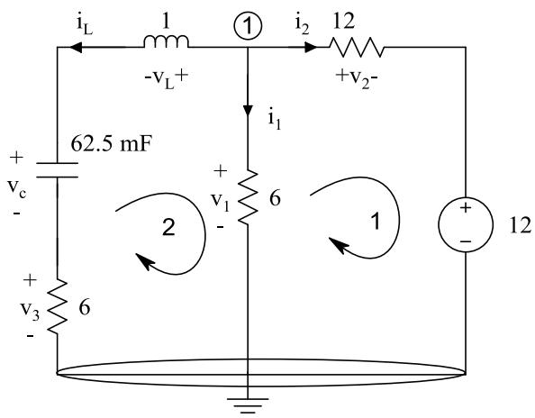
$$\text{Kcl 1: } i_L + i_1 + i_2 = 0 \quad (1)$$
