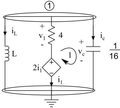
$$\text{Kcl 1: } i_L + i_1 + i_C = 0 \xrightarrow{\text{قانون اهم}} \frac{1}{L} \int_{-\infty}^t v_C(t) dt + \frac{v_1}{4} + \frac{1}{16} \frac{dv_C}{dt} \quad (1)$$
