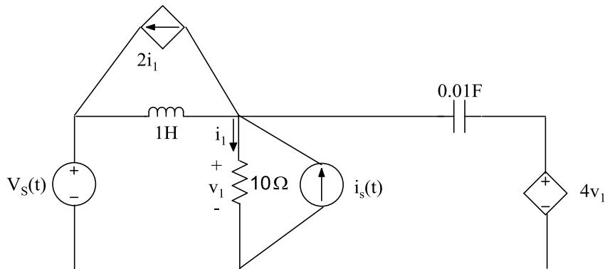
$$V_s(t) = 5\sqrt{2} \cos(10t) \text{ V}, \quad i_s(t) = 2\sqrt{2} \sin(10t) \text{ A}$$
