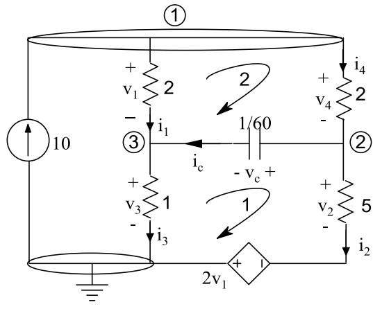
$$Kvl\ 1: -v_c + v_2 - v_3 - 2v_1 = 0 \quad (1)$$
