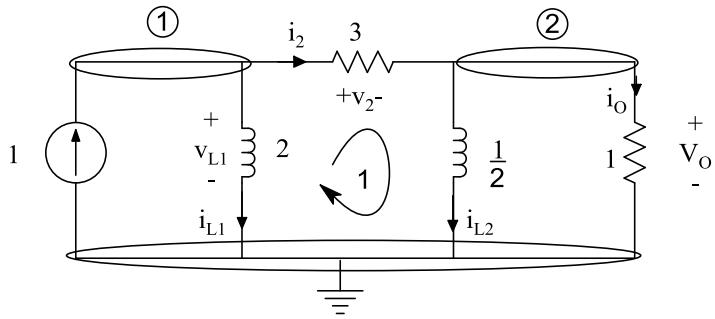
$$\text{Kcl 1: } 1 = i_{L1} + i_2 \rightarrow 1 = \frac{1}{2} \int_{-\infty}^t v_{L1}(t) dt + \frac{v_2}{3} \quad (1)$$
