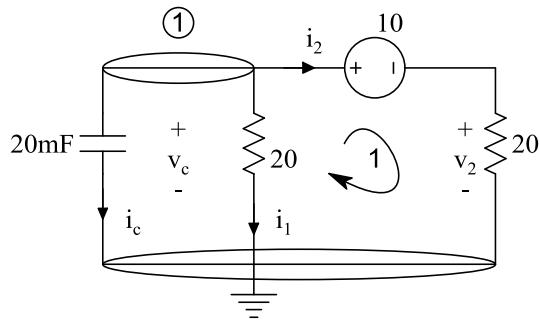
$$\text{Kcl 1: } i_c + i_1 + i_2 = 0 \rightarrow 0/02 \frac{dv_c}{dt} + \frac{v_c}{20} + \frac{v_2}{20} = 0 \quad (1)$$
