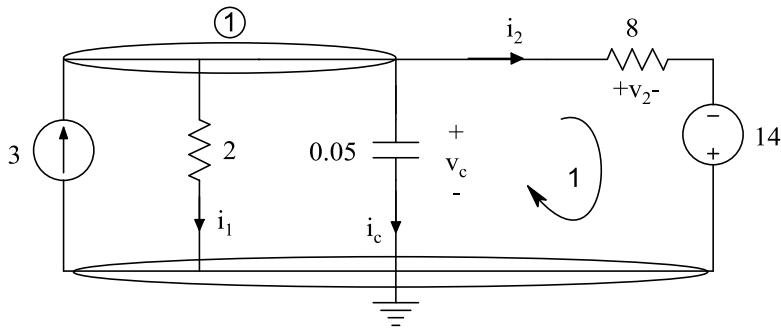
$$\text{Kcl 1: } 3 = i_1 + i_c + i_2 \rightarrow 3 = \frac{v_c}{2} + 0/05 \frac{dv_c}{dt} + \frac{v_2}{8} \quad (1)$$
