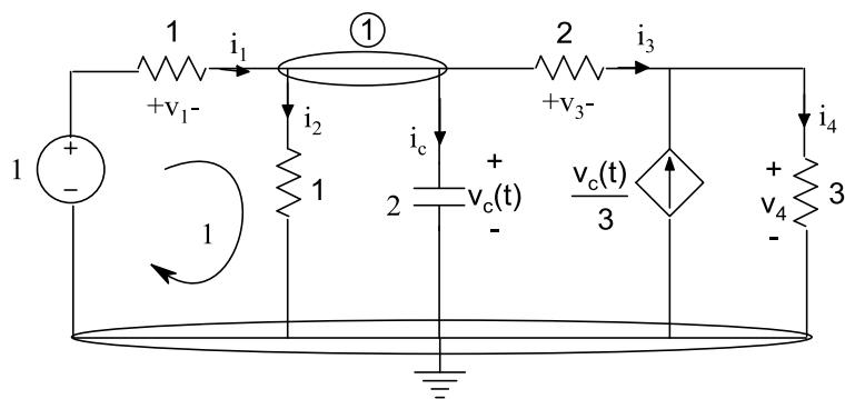
$$\text{Kcl 1: } i_1 = i_2 + i_c \rightarrow v_1 = v_c + 2 \frac{dv_c}{dt} \quad (1)$$
