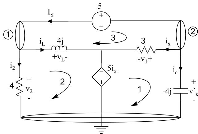
$$\text{Kvl 1: } -v_1 + v'_c + 5i_x = 0 \rightarrow -v_1 + v'_c + 5\left(\frac{v_1}{3}\right) = 0 \rightarrow \frac{2}{3}v_1 + v'_c = 0 \quad (1)$$
