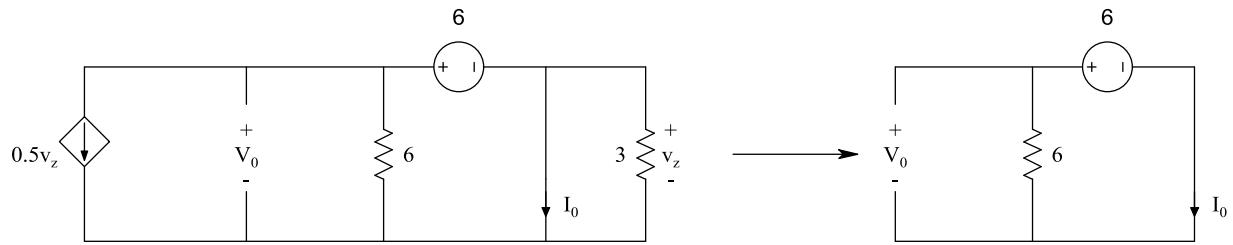
$$V_0 = 6 \quad , \quad I_0 = \frac{-V_0}{6} = -1$$
