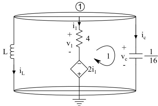
$$\text{Kcl 1: } i_L + i_1 + i_c = 0 \rightarrow \frac{1}{L} \int_{-\infty}^t v_c(t) dt + \frac{v_1}{4} + \frac{1}{16} \frac{dv_c}{dt} = 0 \quad (1)$$
