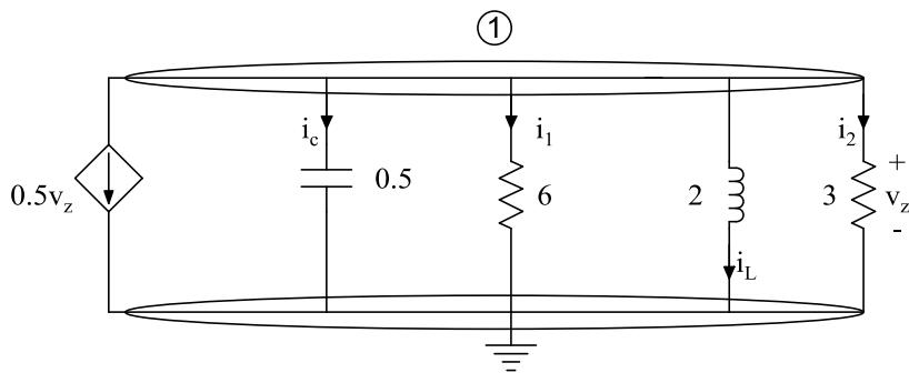
$$KCL 1: 0/5v_z + i_c + i_1 + i_L + i_2 = 0 \quad (1)$$
