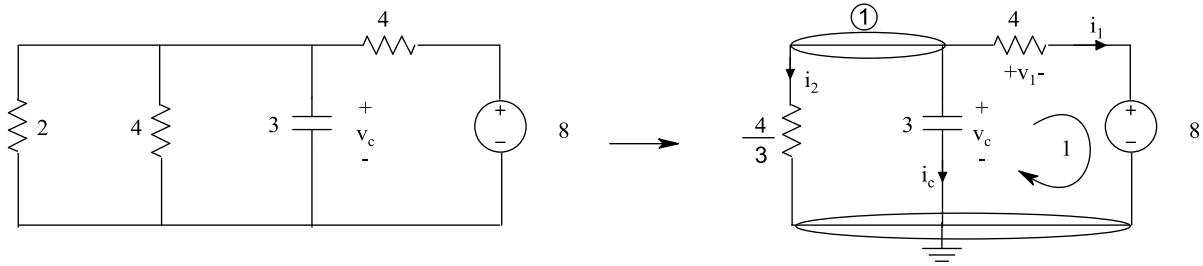
$$\text{Kcl 1: } i_2 + i_c + i_1 = 0 \rightarrow \frac{3}{4} v_c + 3 \frac{dv_c}{dt} + \frac{v_1}{4} = 0 \quad (1)$$
