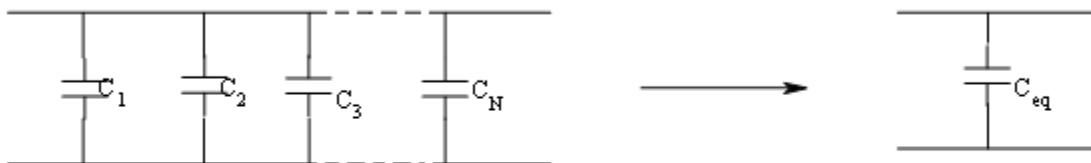
$$C_{eq} = C_1 + C_2 + C_3 + \dots + C_N$$
