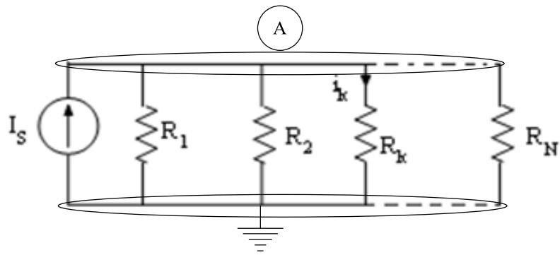
$$i_k = \frac{G_k}{\sum_{i=1}^n G_i} \times I_S \quad , \quad G_k = \frac{1}{R_k}$$
