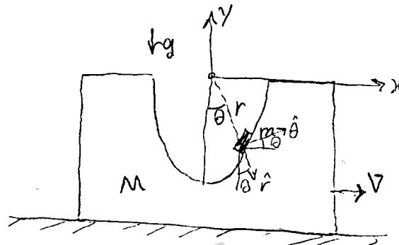
$$z(\vec{v}_{\text{rel}}) : \ddot{\theta} = -g r \cos \theta + \frac{1}{2} M v^2 + \frac{1}{2} m [(r s \sin \theta - r' c \cos \theta)^2 \dot{\theta}^2 + (v + (r's \sin \theta + r c \cos \theta) \dot{\theta})^2]$$
