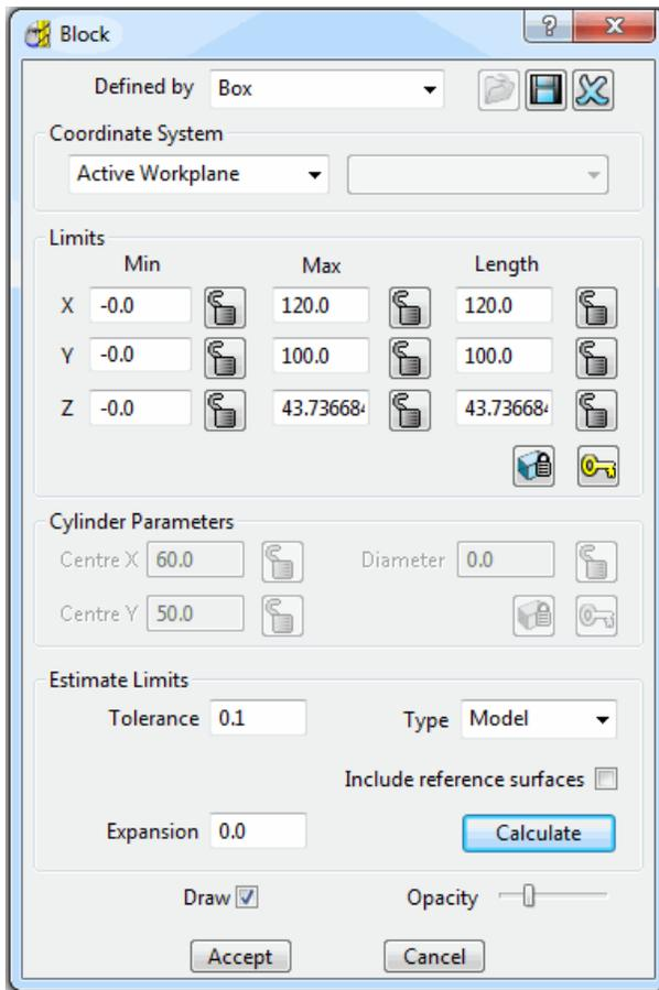
The **Block Form** is used to define the 3D working limits. This could be the actual raw material size or a user defined volume, localised to a particular part of the component.
