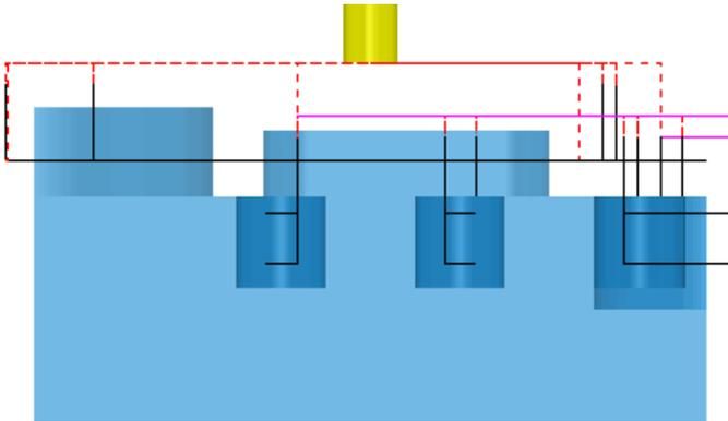
With **Machine flats - Off** the toolpath has totally ignored the *flat surfaces* of the **model**. It has maintained the defined, **Stepdown** value and performed *area clearance* across the material **Block** at each **Z Height**.
