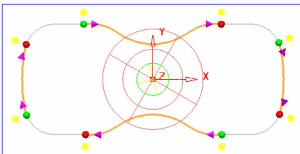
The sections of the **Pattern** included in the original toolpath are displayed, along with the user defined, **Start** (green) and **End** (red) points.
