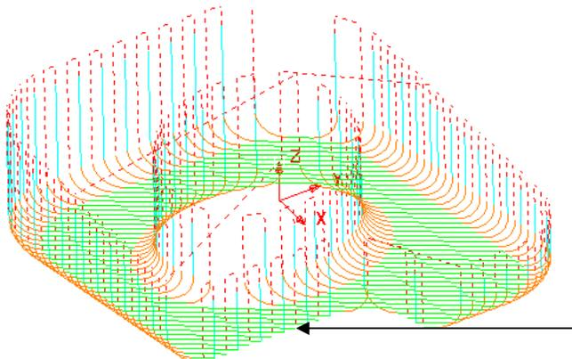
Where the operation is gouge free a **Lead Out** move, similar to the **Lead In** is applied at the end of each tool track.
