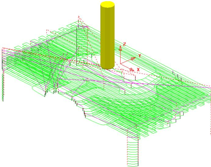
The tool will now plunge locally (pale blue move) from the defined **Incremental - Start Z** relative to each *slice* and rapid across the roughed areas using an **Incremental - Safe Z** (purple move).
