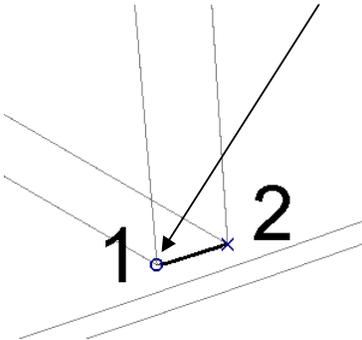
The **Anchor Point** is now selected and is represented by a small circle. The x, y and z values seen in the above form are relative to the **Active Workplane 'Datum'**.
