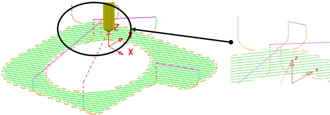
As shown above the **Vertical Arc - lead** moves no longer exist on the **Short links (Circular Arcs)**.
