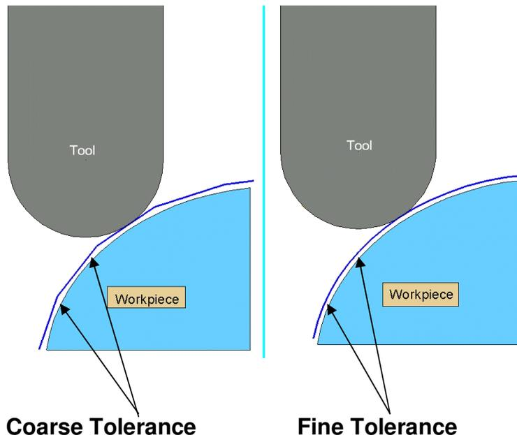
**Tolerance** controls the accuracy to which the cutter path follows the shape of the work-piece. For roughing a Coarse tolerance can be used but for finishing a Fine tolerance must be used.
