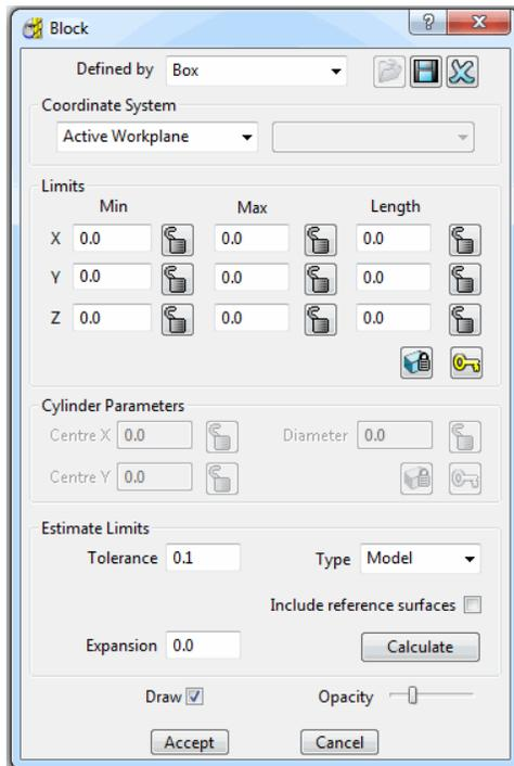
The default option for **Block** is **Box** (A rectangular volume). Other options include **Cylinder** (a Cylindrical volume), a **Triangle** model (Casting) available in PowerMILL PRO only, and **Picture/Boundary** (Extruded 2D wireframe contours).
