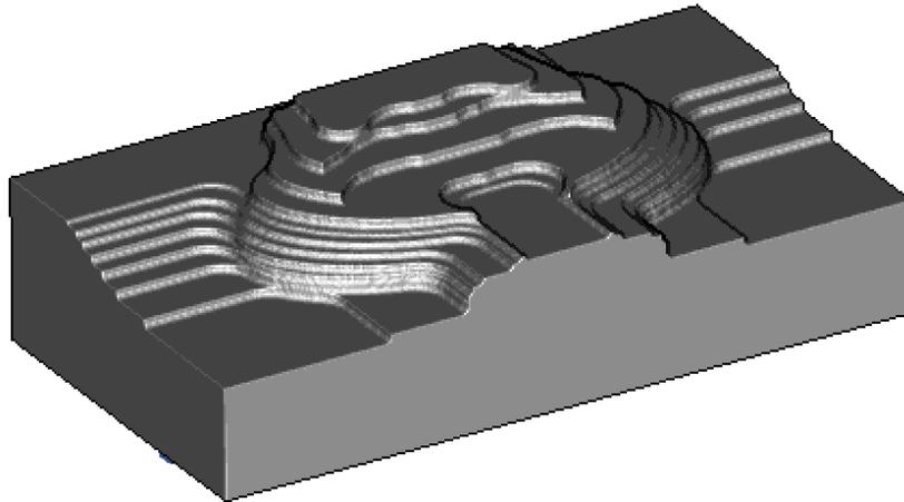
Sometimes known as Waterline Roughing the cutter steps down to a specified **Z Height** and fully clears an area (**Slice**) before stepping down to the next **Z Height** to repeat the process.
