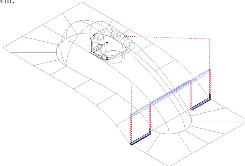
The machining strategies have been localised and the tooltrack shape controlled with the help of edited **Boundaries** originating from a single **Rest Boundary**.
