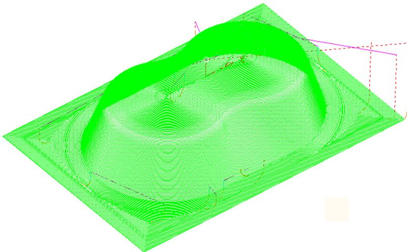
The component form includes 2 *Flat* areas which are currently machined with the same *small stepover* as the angled walls. For more efficiency, an option is available for a larger **stepover** to be independently applied to the **shallow (Flat)** areas.
