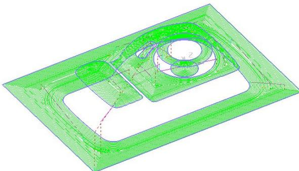
The **Spiral** option is essential for HSM (High Speed Machining) applications where ideally toolpaths should be as continuous as possible.
