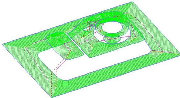
The toolpath has now is now more efficient with the rapid moves at **skim** height and the **short links** being forced onto the surface.
