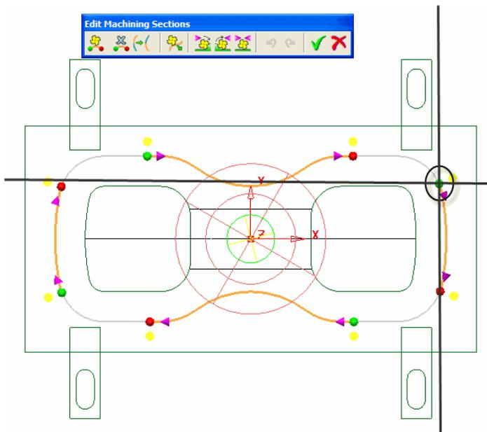
When defining the **Start** and **End** points along the **Pattern** allow room for suitable **Lead** moves.
