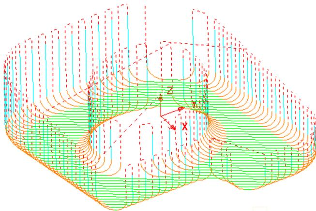
Wherever it is *gouge free* the **1st Choice** of a **Radius 6, Vertical Arc, Lead In/Out** is applied.
