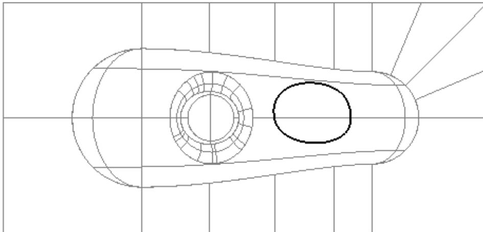
The **Boundary** segment is *splined* through the *polyline points* where doing so maintains the original form to within a *maximum deviation* of **0.5**. In instances where this is not possible a tangency will remain either side of the point.
