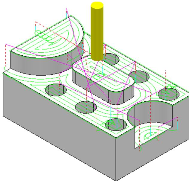
The cutter now passes across the top of the holes without lifting, producing a smoother toolpath. Note that **Ignore Holes** refers to the slice definition at the top of the holes. The flat base of any hole will still be machined.
