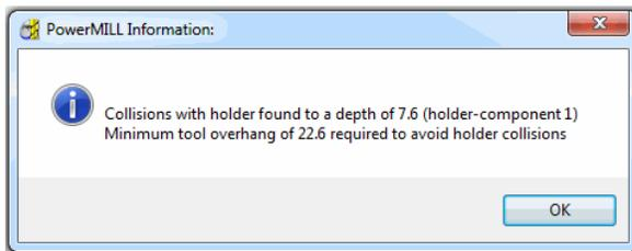
In this case **PowerMILL** has detected that with the current tool **Holder** and **Shank** settings collisions will be present at a **depth of 6mm**. A suggested tool **Overhang** of **21mm** will be required to avoid this.
