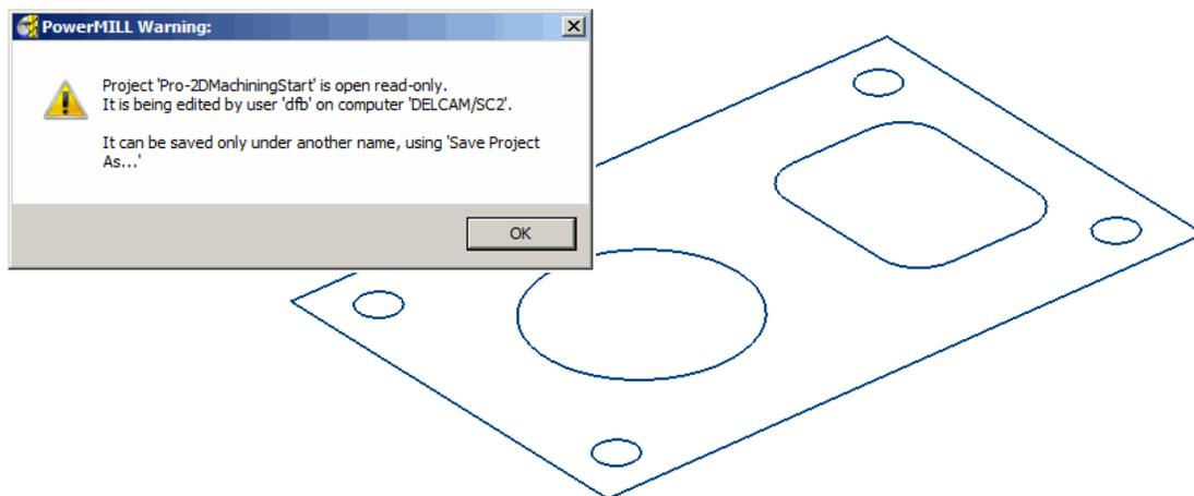
The imported **Project** contains **4 Tools** and **3 Patterns** defining the **2D geometry** to be used in the **2D Machining** options. The **Project** is **Locked** to prevent it from being altered hence the first step is to **Save As** a separate **Project** locally with a different name.
