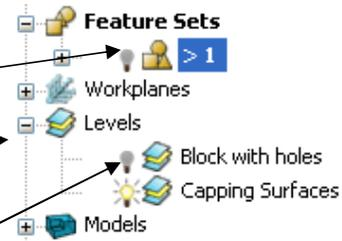
The new **capping surfaces** may be created inside out (*Surface Normals reversed*). If required they can be **selected** and from the local **surfaces** menu **Reverse Selected** can be applied.
