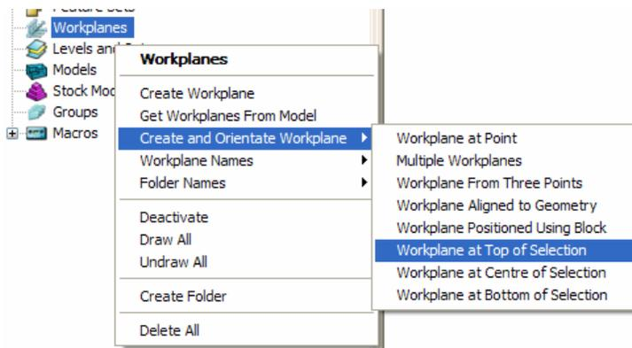
**Workplanes** are additional datums that can be moved and/or orientated within the global environment. One **Workplane** can be **Active** at any one time. If no **Workplanes** are active then the original global **Transform** is the datum.
