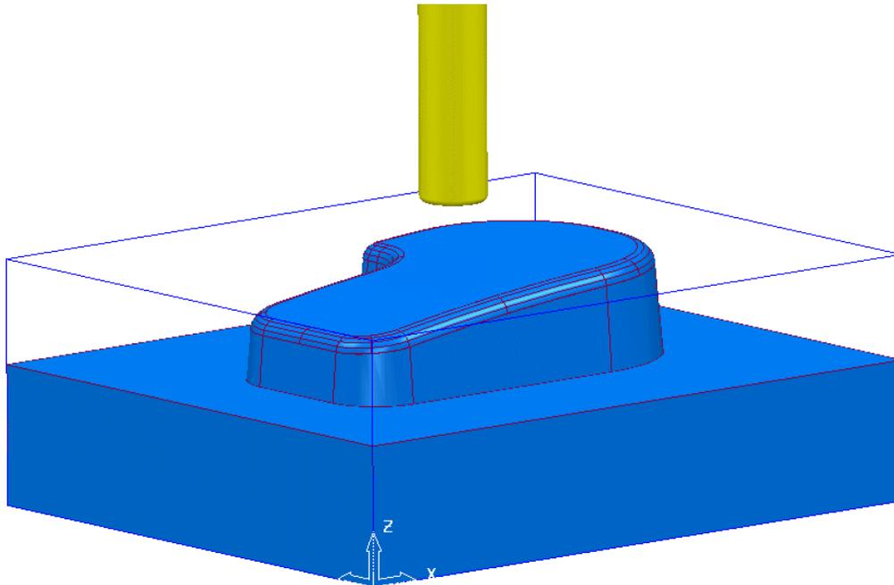
The **D12t1** tool is positioned at the **Block Centre Safe** position ready for the user to create the first toolpath.
