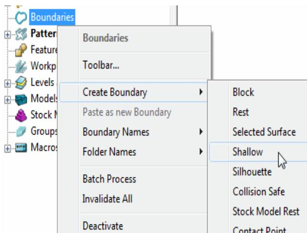
Specific *Finishing strategies* are more effective on either **Steep** or **Shallow** parts of the *3D component model*. For example, *Constant Z finishing* is most effective on *steep sidewalls* while *Raster Finishing* is most effective on *shallow areas*.
