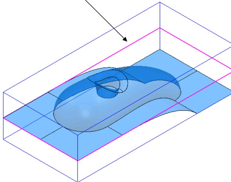
The resultant **2D Boundary** is defined around the outside edge of the **Block** at **Z0**.
