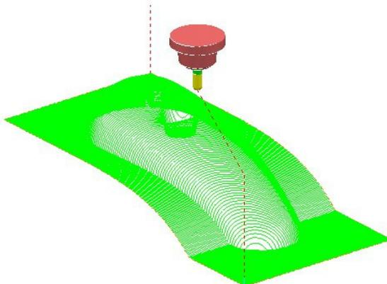
The new, gouge free, **Toolpath** is generated but at this stage no collision checking has been applied in relation to the **Shank** and **Holder**.
