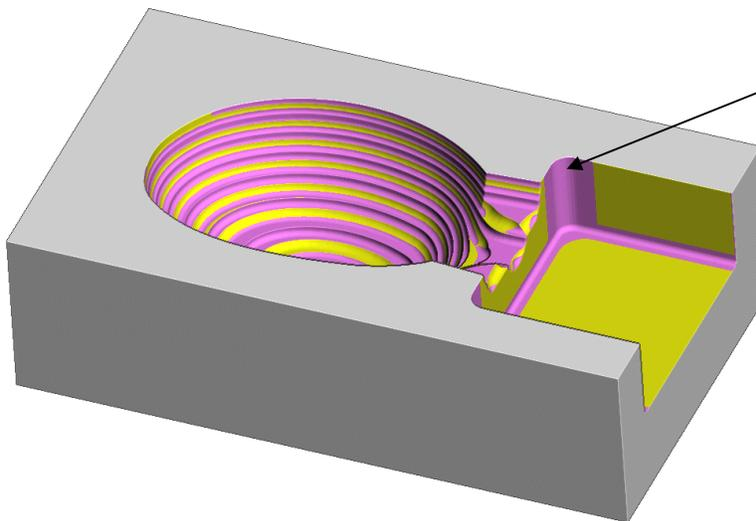
The **ViewMILL** simulation shows this next toolpath shaded in a different colour where it has machined in areas the previous toolpath did not cover
