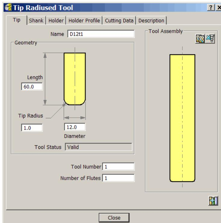
The **Tip Radiused Tool** form opens ready for the user to input the required values. When a diameter value is input the tool length automatically defaults to five times this value. This value can be edited if required.
