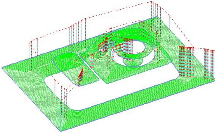
The toolpath follows the contours of the **Boundary** segments and is produced only on the shallow areas of the model (**Inside the Boundary**).
