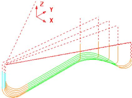
A **Vertical Arc Extension** has successfully been added to all of the **Lead In/Out** moves.
