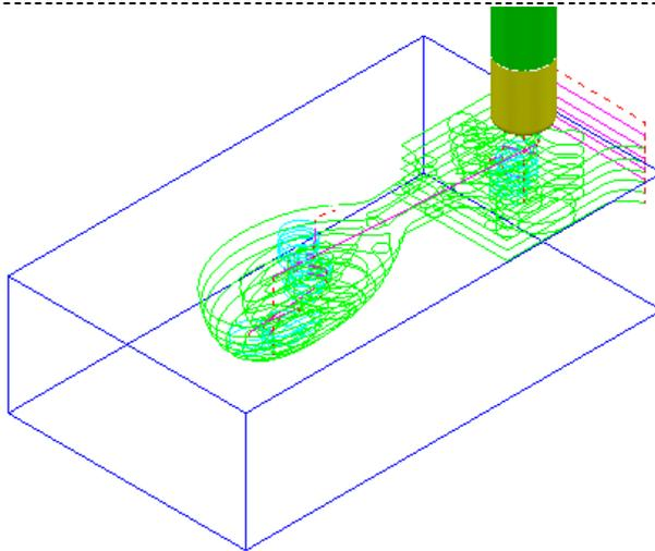
The **Offset all - Area Clearance** strategy follows both the contours of both the **Model** and **Block** then gradually offsets into the remaining material at each **Z Height**.
