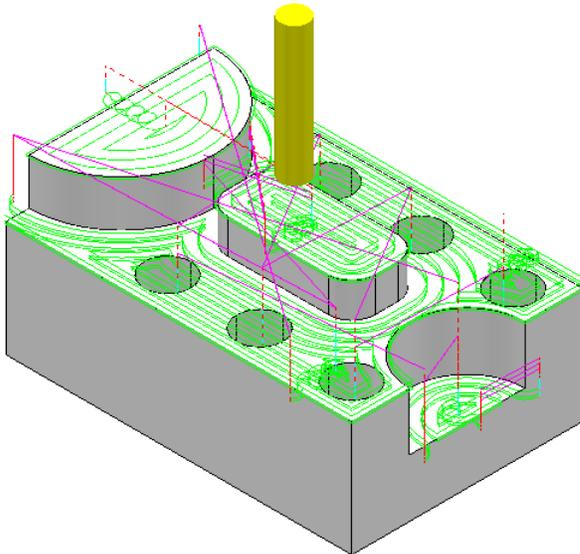
Note the 'D' shaped **Flat** area at the very top level is not using **Multiple Cuts** as the top of the **Block** is the overall **Z limit** for the strategy.
