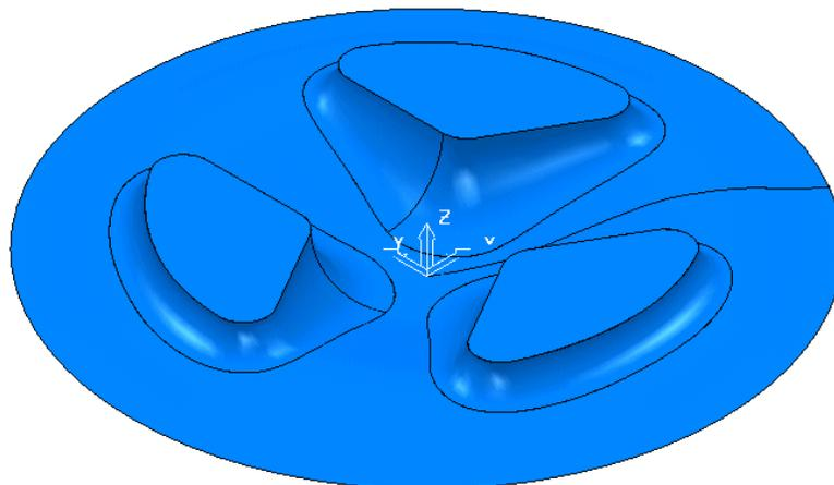
The component is circular as a result of which the **Block - Z Minimum** and **Z Maximum** will be developed as a **Circular** billet.
