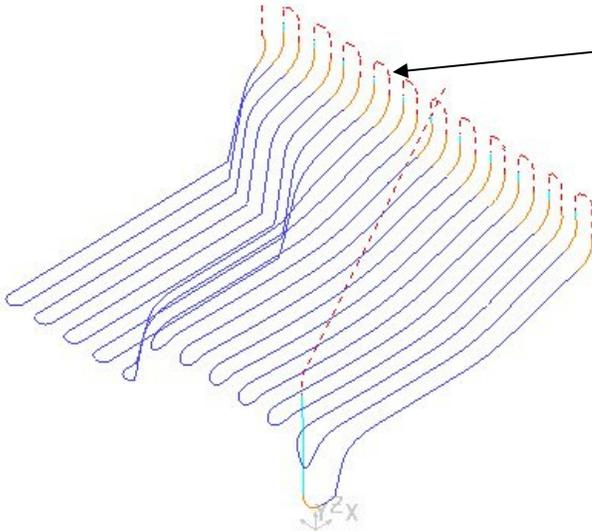
Note that **arcs** can be applied to the **Rapid Moves** (If the individual Machine tool controller supports the option).
