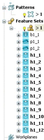
The contents of the **Feature Set (1)** should be similar to the illustration on the left (Note: The Author has opted to use a naming system where a **Boss** is prefixed with a **b**, a **Pocket** with a **p**, and a **Hole** with an **h**).
