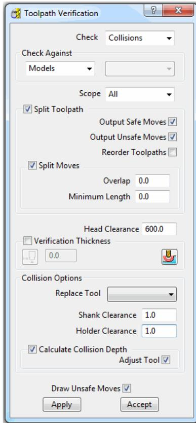
The two **Check** options here are **Collisions** and **Gouges**. **Scope** contains options to control which actual elements of a toolpath are checked.
