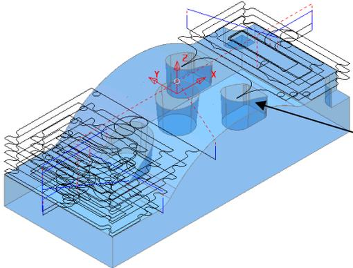
**Area Filter** has been applied to prevent the cutter attempting to machine into confined areas.
