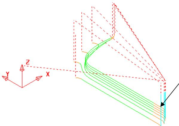
An additional (**Distance**) extension move is added to the **tool track** before the original **Lead In** option 'kicks in'.
