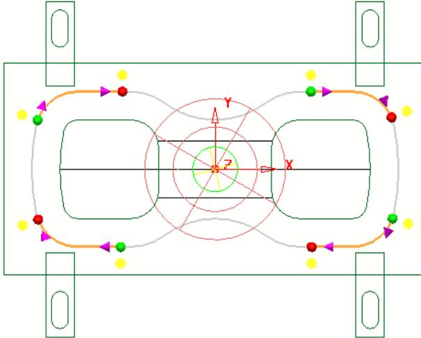
The sections of the **Pattern** included in the original toolpath are displayed, along with the user defined, **Start** (green) and **End** (red) points.
