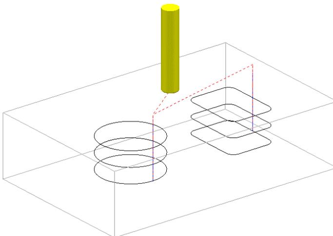
Note the tool is plunging directly onto the form down Z. This situation will be changed retrospectively by applying appropriate options in the **Leads and Links** form.
