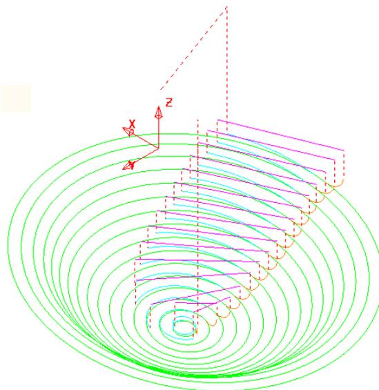
**Overlap Distance** continues the cutter before or after the natural end point (Along the original toolpath) by a specified distance based on the *Tool Diameter (TDU)*.
