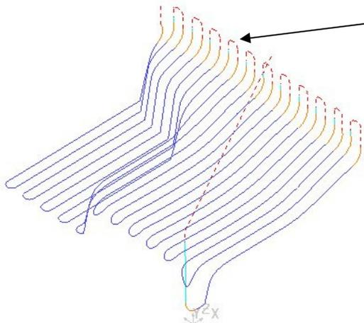
If the **Short** links are set to **Skim** and **Arc Fit Rapid Moves** is set, then arcs are added to the rapid moves.
