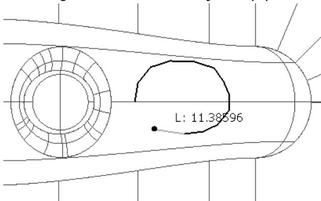
Note: Do not attempt to close the segment by trying to snap the 'final span' back on to the start point. Use the Close segment icon to achieve an exact match.
