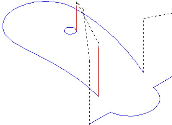
The toolpath is produced. The steep area is not machined.
