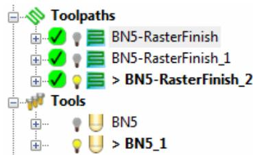
**PowerMILL** has created two new toolpaths, **BN5-Raster Finish\_1** and **BN5-RasterFinish\_2**. A new tool named **BN5\_1** has also been created in the tools area of the explorer. This new tool has been created with the new valid adjustments made i.e. **Overhang 21**.
