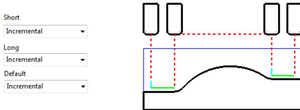
**Incremental** applies the *rapid feed rate* all the way down to an **Incremental Start Z** measured from the *full plunge depth* at which point the slow **plunge feed rate** ‘cuts in’. The **Plunge** option differs from **Skim** in that all **rapid link** moves occur at the **Absolute Safe Z**.
