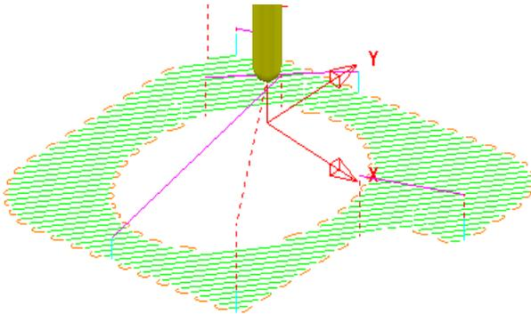
Note that by increasing the value of the **Short/Long Threshold** the number of **Short Link Circular Arcs** has greatly increased.
