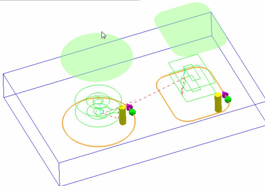
Note: While the **Curve Area Clearance** form is open, the areas to be machined are displayed as a shaded preview.
