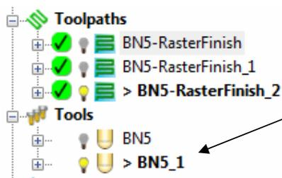
PowerMILL has replaced the *newly created* Tool **BN5\_1** (with an extended overhang) into **BN5-RasterFinish** and **BN5-RasterFinish\_2**.
