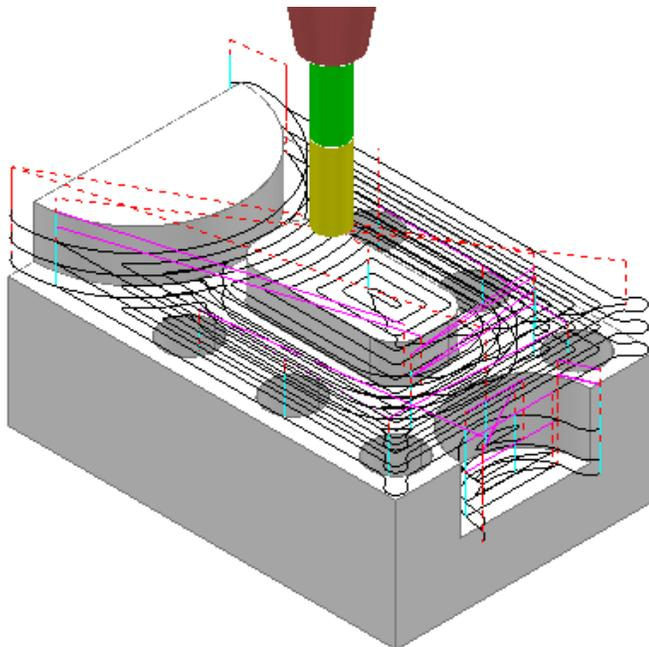
The **Model Area Clearance** toolpath now removes material across the *whole block area* leaving **0.6mm** stock above each **Flat face** (The **thickness** plus the **tolerance**).
