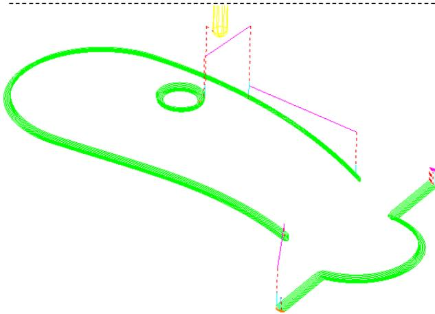
**MultiPencil** appears to be very similar to the **Corner Along** strategy. There however fundamental differences one being the toolpath segments in **Corner Along** are offset from the outer profile inwards, whereas in **MultiPencil** the toolpath segments are offset outwards from the true intersection.
