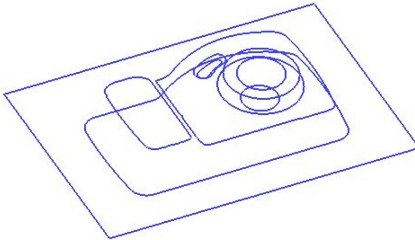
With the model and toolpaths undrawn the **Boundary** should look something like this. It is made up of numerous segments each one dividing the model into steep and shallow areas. Any of which can be selected and individually deleted at any time except when **Locked** due being assigned to a toolpath.
