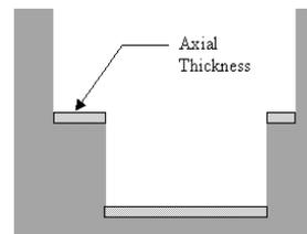
Clicking the **Thickness** button on the **Area Clearance** forms opens the **Axial Thickness** box allowing the user to set separate values for **Radial** and **Axial** thickness. This facility is also available on the finishing forms.
