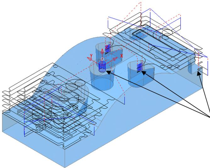
The existing toolpath is allowing the cutter to machine into confined areas. This is resulting in sudden sharp changes of cutting direction and excess loading on the tool.
