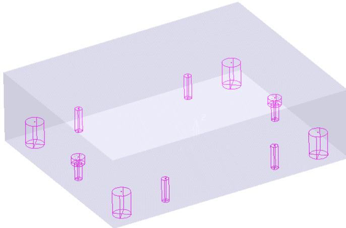
A **Hole Feature** is created for each of the selected *holes in the model* (including the counter-bores).
