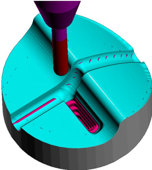
The **Pale Blue** area shows where the **Dia 10 Ball Nosed** tool has successfully machined. The deep pocket (**Purple**) is inaccessible and still includes large steps down the side wall. This excess stock could cause a smaller finishing tool to break if it attempts to **Corner Finish** down the pocket. To prevent this, the **Remove Deep Cuts** option will be used as demonstrated below.
