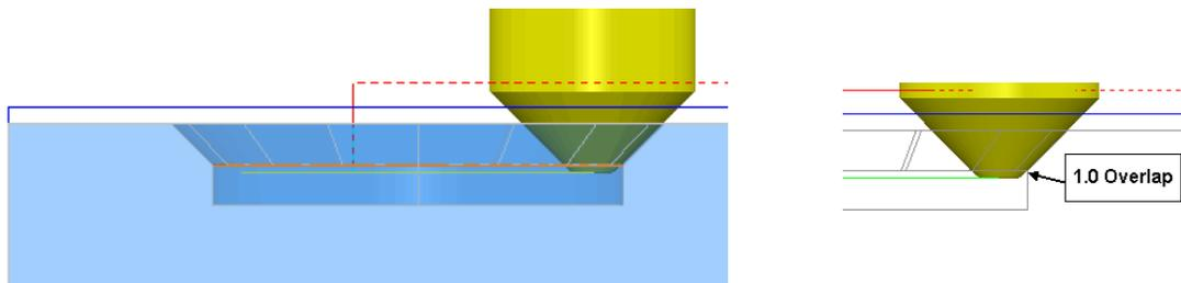
A **surface** model of the finished component has been imported to provide a visual check of the **Chamfer Machining**. The **1mm tool overlap** at the base of the chamfer is clearly visible in the above illustrations.
