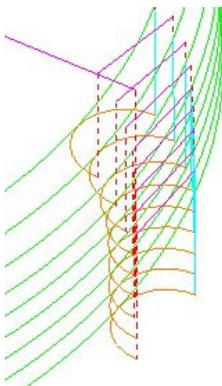
The tool now **leads in** and **out** of the toolpath with a **horizontal arc**. If the tool lifts it will only lift by the **skim** distance taken from the first page of the **Leads and Links** form (**Z Heights** tab). The **Rapid** moves at **skim** height are purple in colour while the **plunge** moves are light blue.
