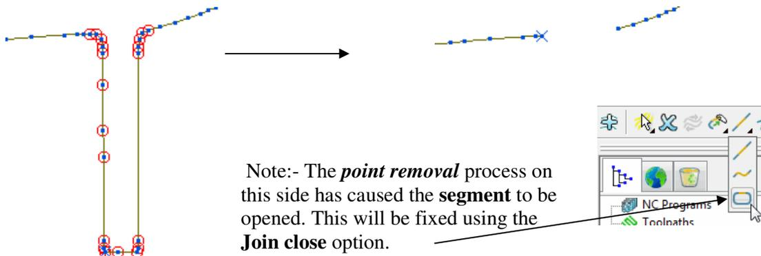
Note:- The **point removal** process on this side has caused the **segment** to be opened. This will be fixed using the **Join close** option.
