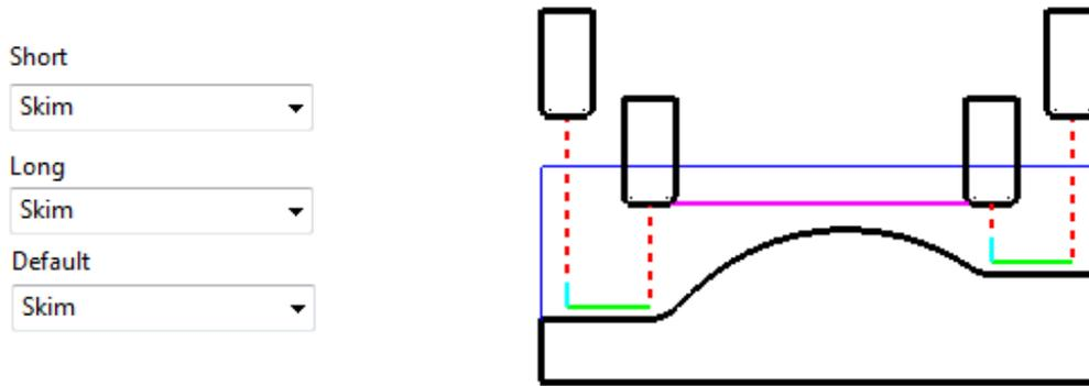
**Skim** enables the downward, *rapid feed rate* to continue to a specified **Incremental Start Z** above the *full plunge depth* before the slow **plunge feed rate** ‘cuts in’. **Skim** then applies a **rapid retract** to an **Incremental Safe Z** above the *highest point* on the component ‘in line’ with a *linear link* move to the next *plunge* position. To cater for all types of *machine tool* this move is a (*Purple*) **Skim Feed Rate** (G1) as instead of a (*Dashed red*) **Rapid** (G0).
