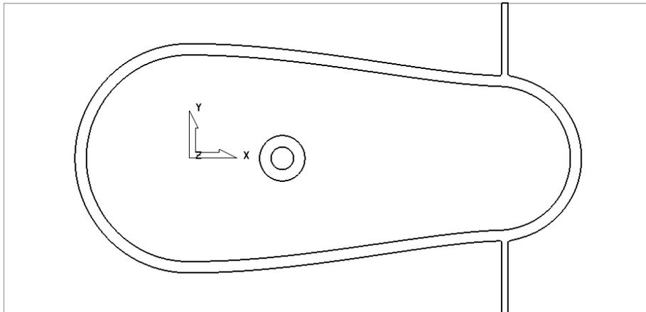
The above **Boundary** identifies areas on the component that are inaccessible to the **bn16** tool geometry to be locally machined with the **bn8** tool. On closer inspection the central pocket area would be more effectively machined with a flat bottomed tool and a smoother more continuous toolpath will be achieved if the 2 spurs were removed from the outer segment, to be machined later as a separate toolpath.
