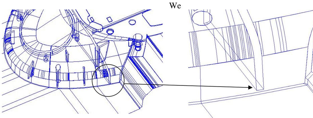
The gap at the bottom of the slot will be measured to determine its size and depth. Note that it is essential to **Zoom** in close to be able to discriminate the close proximity node points.
