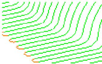
All unnecessary **retract** moves have been eliminated with a **circular arc** move now forming the **link** between adjacent tool tracks.
