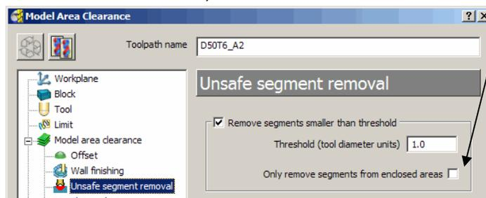
All tooltracks spanning a distance less than the **Tool Diameter (TDU)** will be filtered out and not appear in the final **Toolpath**.
