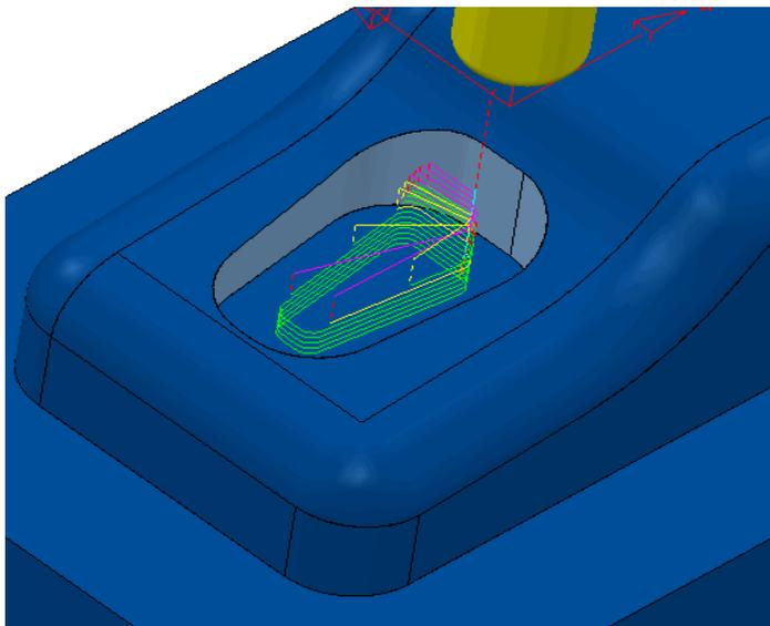
The **Toolpath** now follows a direction, parallel to the base of the selected **Surface**.
