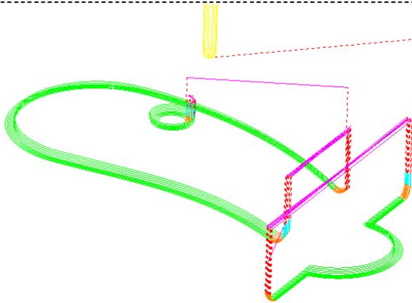
The **Vertical Arc** lead provides a smoother transition onto the work piece with the tool already moving at the specified cutting feed rate.
