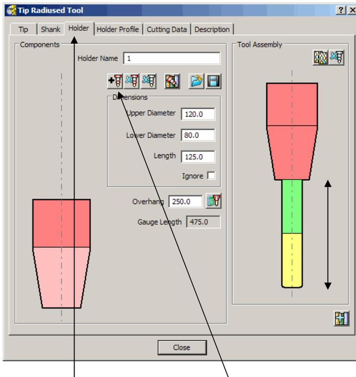
The **Overhang** is the vertical distance from the bottom of the holder to the tip of the cutter.
