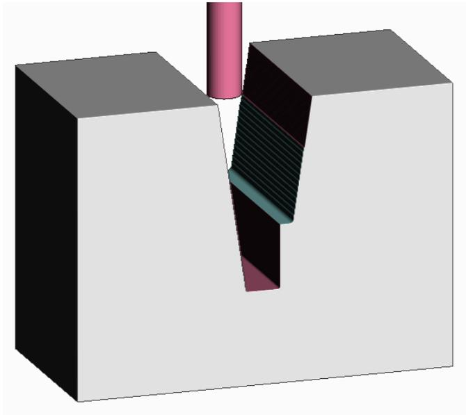
The existing **Constant Z** finishing strategy is ploughing into the stock that was inaccessible to the previously *simulated* **Roughing** toolpath. The excessive loading is likely to result in *tool breakage*. To avoid this problem the **Constant Z** strategy will be modified to include the **Add Stock** option.
