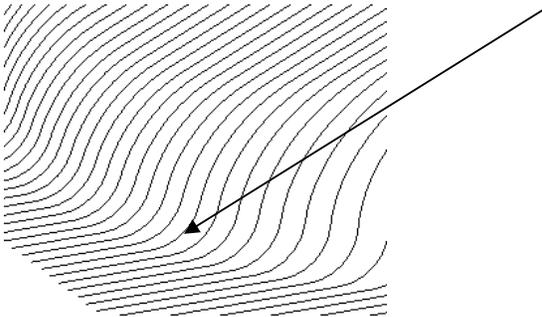
At the end of each **tool track** the cutter **retracts** to the **Safe Z height**. This is a waste of time as these lifts are unnecessary. To make the toolpath a more efficient **Link** option can be applied.
