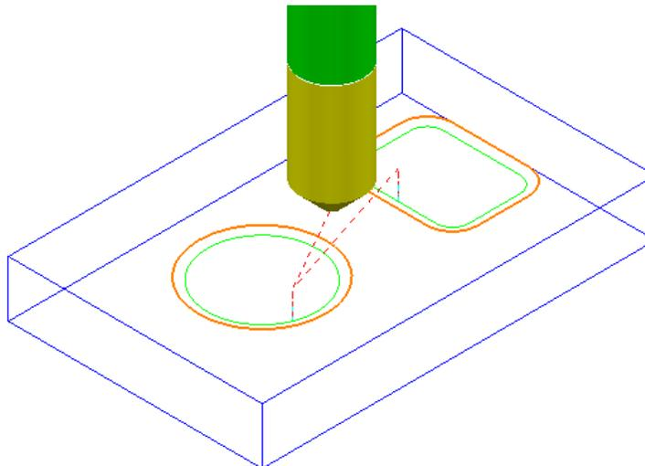
The **Chamfer Milling** options selected result in the angled part of the tool overlapping the base of the Chamfer by **1mm**.
