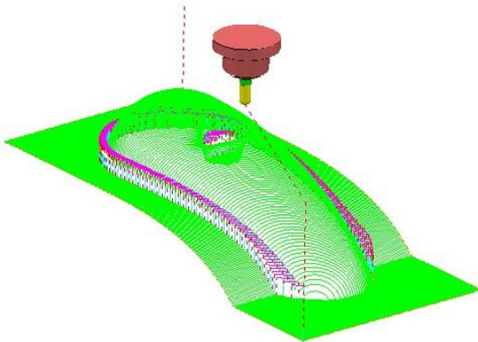
This toolpath only contains segments of the original toolpath, **RasterFinish**, that do not have any collisions so the original tool and tool holder, **BN5** is still associated with it. If your preference is to run with the shorter overhang then you could run this toolpath on these areas shown.
