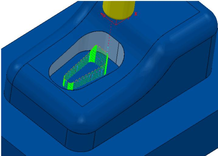
Due to the natural direction based on **along or across** the surface, the **tool tracks** run up and down the sidewalls. This is not the correct choice as it is required to step the **tool tracks** down the sidewalls.
