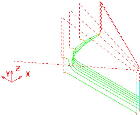
There is no need to input a **2nd choice** as the **Horizontal Arc - Leads In/Out** have appeared on all the tool tracks. With **Horizontal Arc** set, **PowerMILL** decides whether to use **Left** or **Right** hand arcs. They are also calculated to comply with the **Gouge Check** flag. If it is not possible to apply the specified lead due to a gouge situation it will remain as the default **vertical** move unless the **Gouge Check** flag is unchecked (not recommended).
