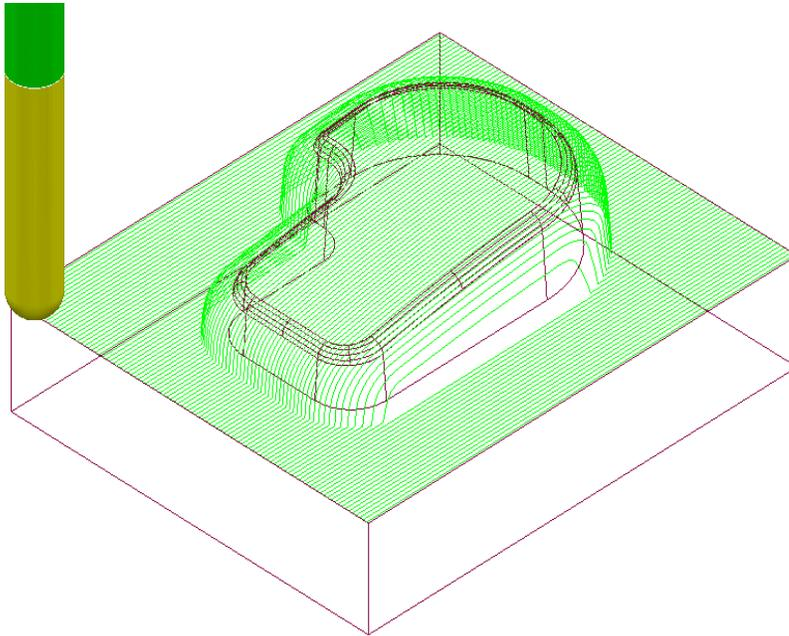
The **Raster Finishing** pattern is projected down Z onto the component taking into account tool geometry and machining settings. Note:- The toolpath link moves, clear of the job are not displayed in this illustration for clarity.
