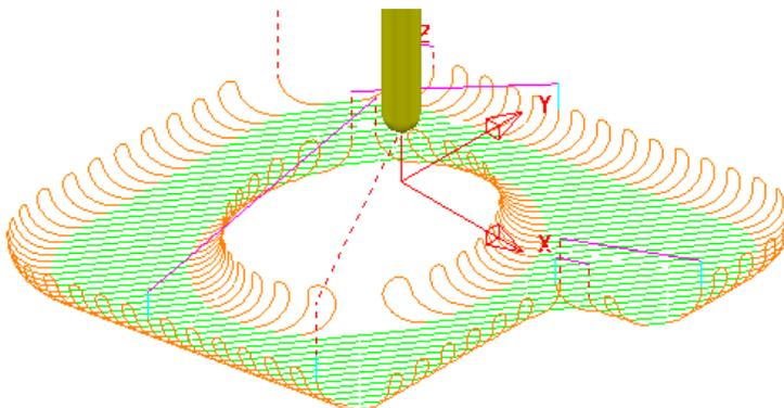
The **Vertical Arc - Leads** are currently adding to the **Circular Arc - Short link** moves.
