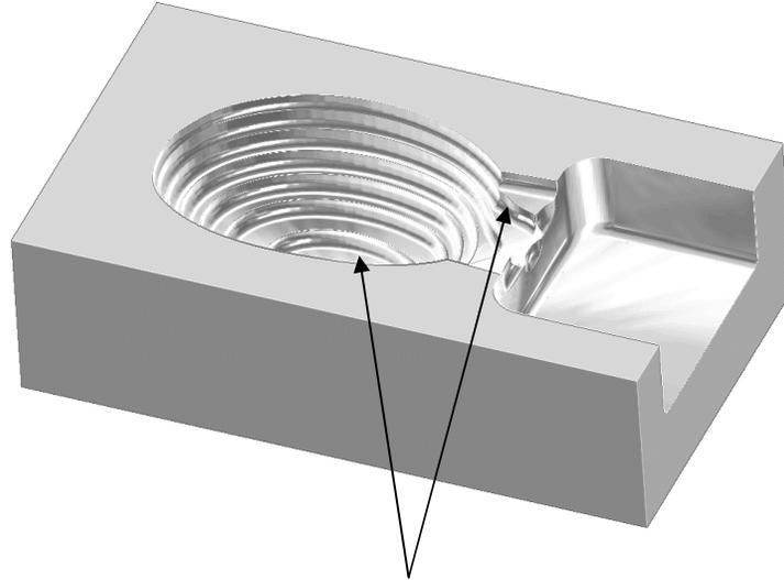
The finished result indicates that the current tool has not been able to remove enough material from some areas of the model.
