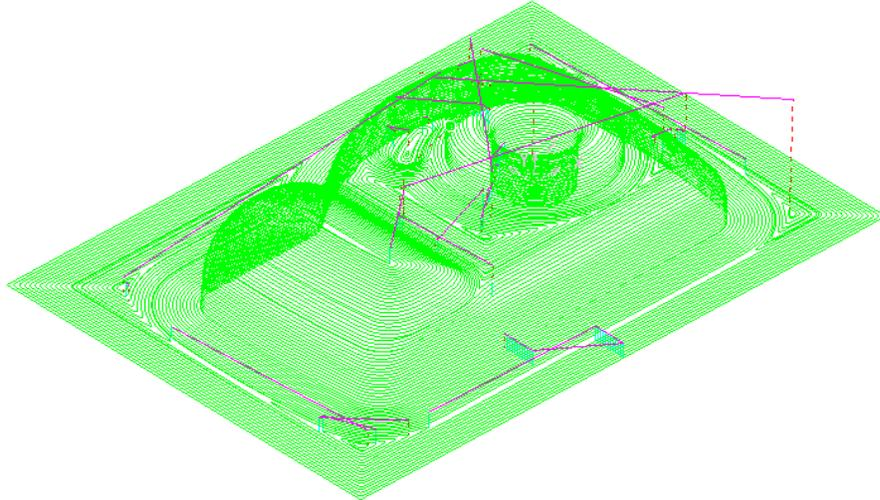
**Optimized Constant Z** generally performs well on **Models** that contain extreme **Steep** and **Shallow** areas, with a minimum of areas around 45 degrees to the vertical. A typical application would include many types of Thermoform Packaging.
