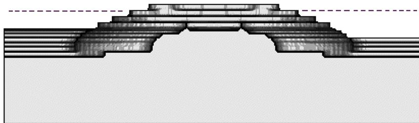
For some components a secondary **Area Clearance** strategy is applied using the **Rest Machining** options in conjunction with a smaller roughing tool. This will locally remove pockets of excess material inaccessible to the original **Reference Toolpath** or **Stock Model**. This will reduce the degree of tool overload and provide a more consistent material removal rate for any subsequent **Finishing** operations.
