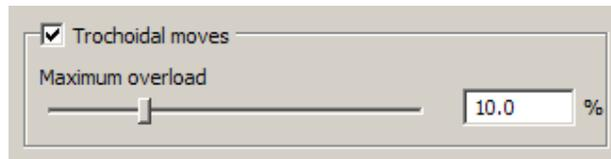
If the tool reaches a specified overload situation **PowerMILL** automatically inputs a **trochoidal** path to eliminate full width cuts. This will occur in corners, narrow channels, slots, etc and the degree of movement is controlled with the slider as a percentage value in the form.
