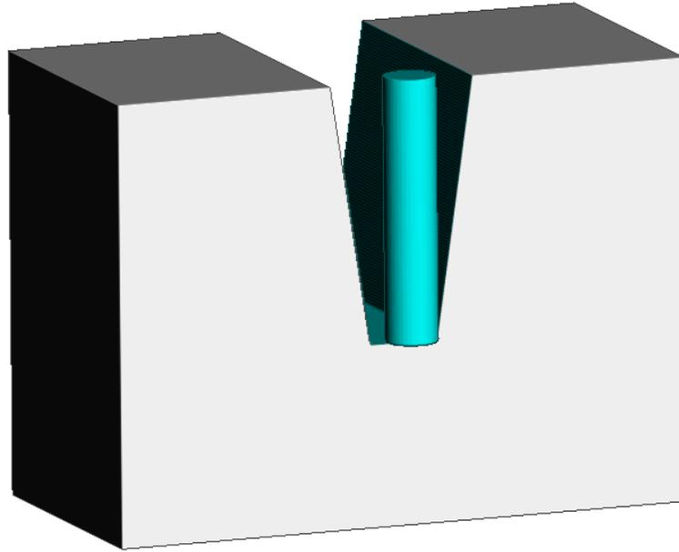
The new **Constant Z** finishing strategy **Pocket** machines continuously down each side of the slot up to the depth where the width of the slot is equal to **TDU + 8**. The strategy then continues but with the **Pocket** option ignored for the remaining **tool tracks**, which alternate between each side wall in descending order.
