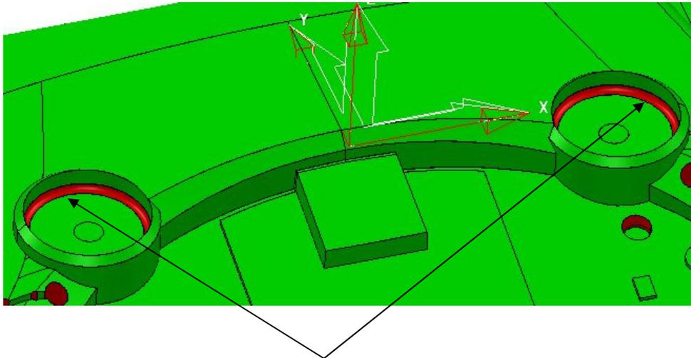
The two internal radii can be seen shaded **red** visually identifying that they will not be machined to their correct size if the default value tool was used.
