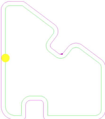
The effect of the **Cutter Compensation** is not visibly displayed in **PowerMILL** for this type of **2D Strategy** but is applied during post-processing for the **ncdata** output file.
