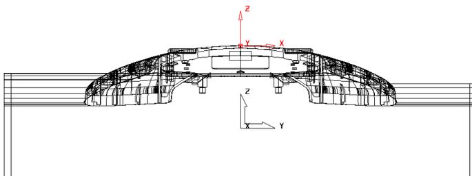
The **Workplane** is shown positioned on the top of the model, which has the longer edge aligned to **X**.
