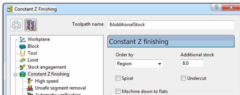
The choice of the selected **Additional Stock** value requires user intervention in estimating the width of the slot, just above the depth of material accessible to the **Roughing** strategy.
