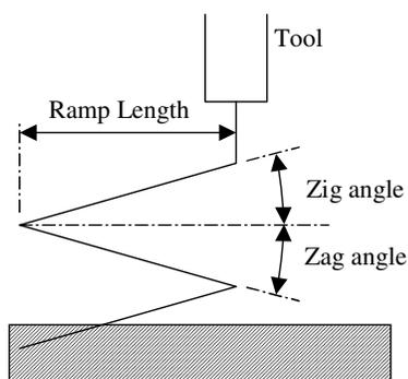
The **Zig** angle is the angle of descent along the machining direction as the tool **ramps** into the material. There are 3 different types of **ramp** move following the geometry of the **Toolpath**, a **Circle**, or a **Line**. If the **length** of the **Zig** angle is limited to a **finite distance** a ramp move in the opposite direction (**Zag** angle) can also be applied.
