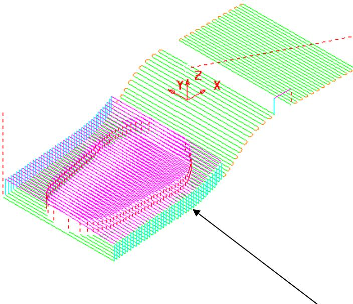
Where the **Link** move from the end of a **tool track** to the start of the next is within 3mm, an (orange) arc move will be implemented.
