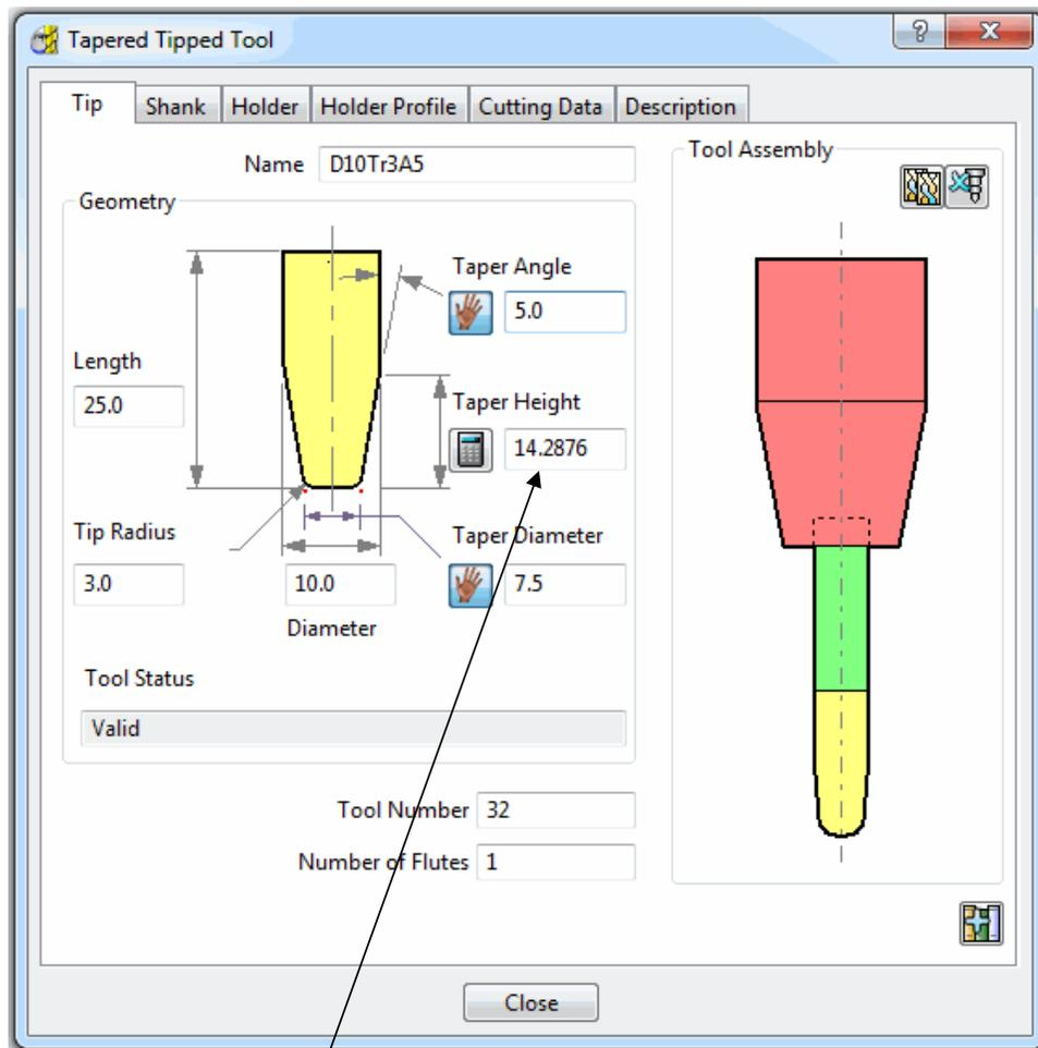
Note:- To calculate the **Taper Height** based on the **Taper Angle** and base **Taper Diameter**
