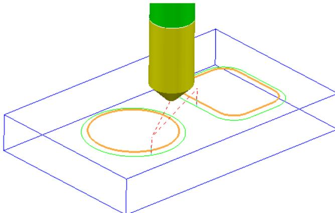
The resultant **Chamfer Milling** strategy has appeared on the wrong side of the **Pattern**.
