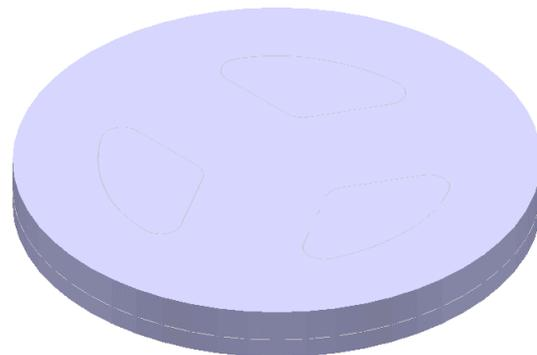
Before the **Pattern** finishing strategy is created, a preliminary **Area Clear** strategy is required to remove the bulk of the material, leaving **0.5mm**, followed by a **Semi Finishing** strategy leaving **0.2mm** prior to the final **Finishing**.
