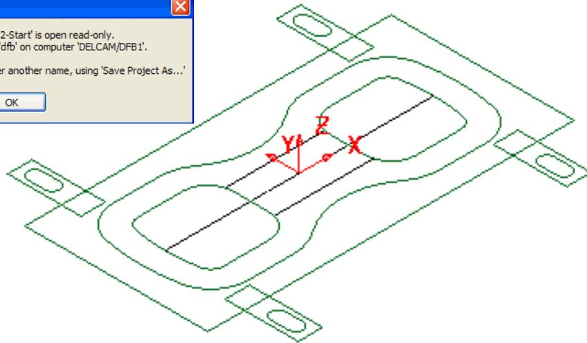
The imported **Project** also contains a **Dia16 End Mill** and a **Pattern** defining the **2D geometry** used in the existing **2D Machining Strategy**. The **Project** is **Locked** to prevent it from being modified, hence the first step is to **Save As** a separate **Project** locally with a different name.
