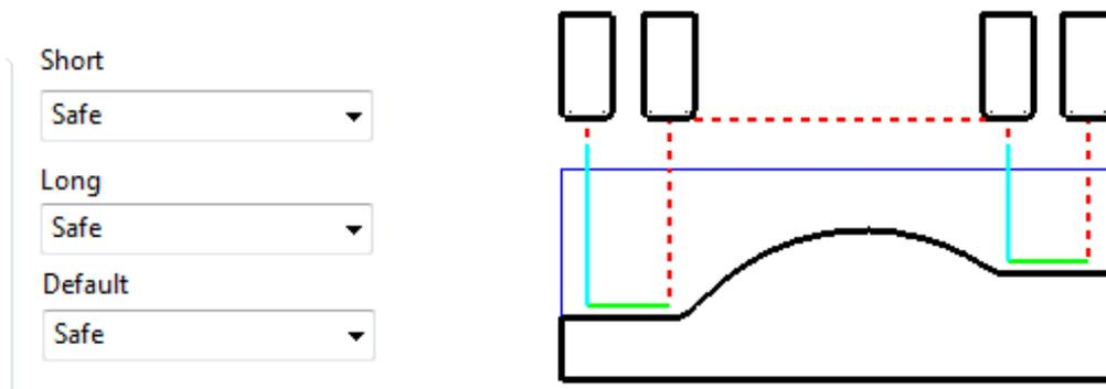
**Safe** (default) sets the **plunge feed rate** to apply at a specific height above the job. This is more predictable and reassuring for the *machine tool operator* but the time take by the non-cutting (air) moves is inefficient especially in the case of large, deep components. In the section of the form labelled **Incremental Heights**, in addition to **Safe**, two other options **Skim** and **Incremental** are available.
