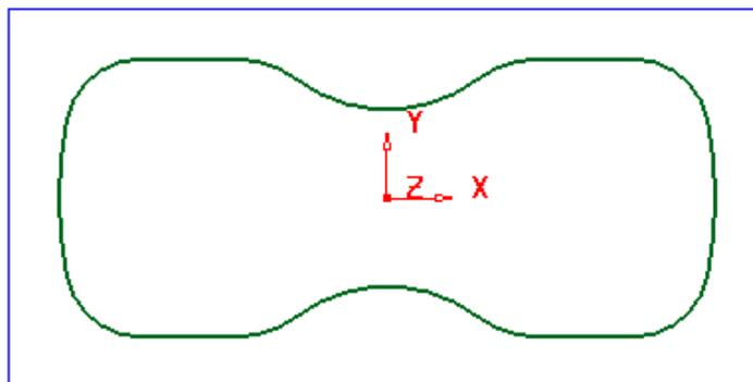
The above **Pattern segment** was created by using **Insert - Model** with the required **wireframe segment**.selected. The same **Pattern** will be used in the creation of the next **Toolpath**.
