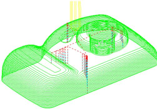
If the **Boundary** had not been used the toolpath would have looked like this. It can be seen that the parts of the toolpath on the shallow areas have an excessive **Stepover**.
