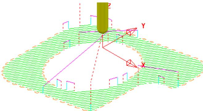
Note that the **distance** between the ends of adjacent **tool tracks** is greater than the **Short/Long Threshold** value in several areas of the toolpath (**Skim Link** moves apply).
