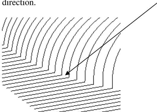
Selecting the **High speed** page **Arc fit corners** option in the form will *arcfit* these to a maximum radius of **0.2 TDU**.
