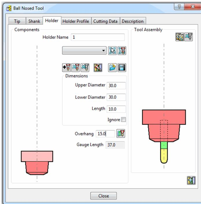
If it is required to modify or delete a **Holder** element, select (left click) on one of them in the assembly illustration and it will turn pale. The current values for that element will be displayed and available for modification.
