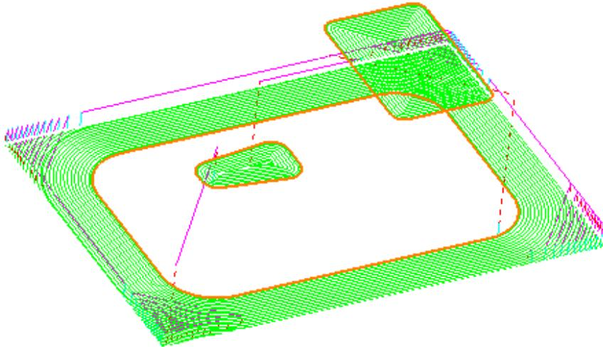
Observe the current **direction** and **ordering** of the strategy considering potential improvements. For example, the lower area machining would benefit from climb milling inwards towards the component form and the pocket machining could start central and climb mill outwards towards the sidewall.
