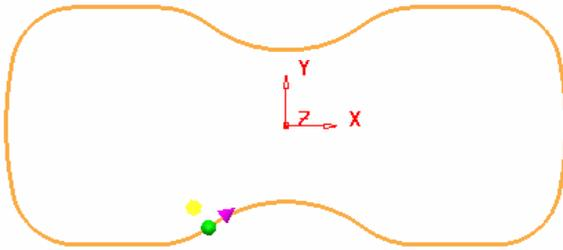
If the **Curve Profile** strategy is used from scratch, the **Mark all sections for machining** option must be selected to provide full control over which side and sections of the **Pattern** are to be machined.
