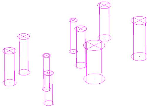
The **tops of the holes** are defined as the shortest distance from the **top** or **bottom** of the material **Block**.
