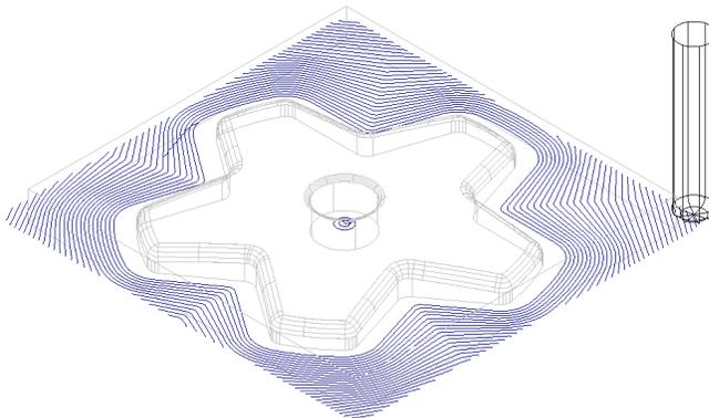
Compare both of the **Model Area Clearance** toolpaths noting the progressive straightening of tool tracks on the second strategy (25% smoothing applied).
