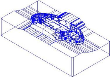
Although it is possible to rotate the actual component this is not generally regarded as the ideal approach. An additional moveable datum (**Workplane**) will be created and rotated through 90 Degrees to effectively create the condition that the longer side of the component is parallel with the front of the machine. The original coordinate set-up can then easily be re-activated for tasks such as checking dimensions.
