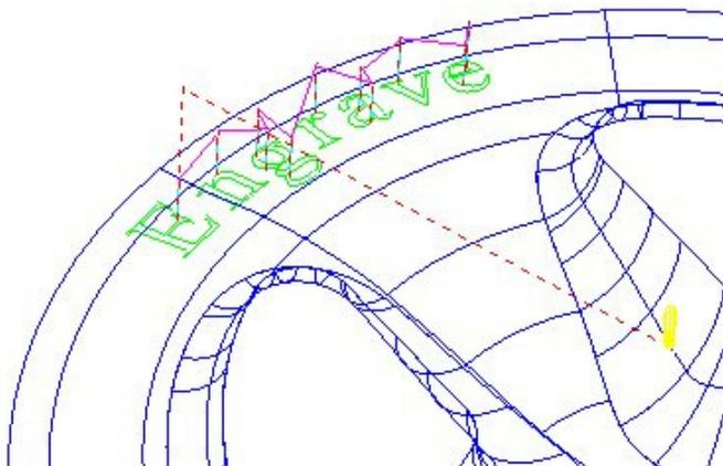
By entering a negative **Thickness** the tool will machine into the previously finished surface. This is frequently used for engraving. Note: It is not possible to use a **-ve thickness value** that is greater than the **Tool Tip Radius**. There is however a way to achieve this if the user has a **PowerMILL PRO** license (Chapter 11 **Patterns**, page 20 - **Deep Pattern Machining**).
