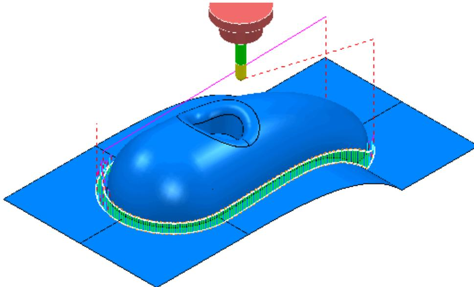
Note that **Automatic Collision Checking** is still active and as can be seen in the above illustration there is no evidence of the **toolpath** being fragmented.
