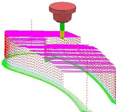
This toolpath contains segments of the original toolpath that can only be machined with the newly adjusted tool **Overhang**.
