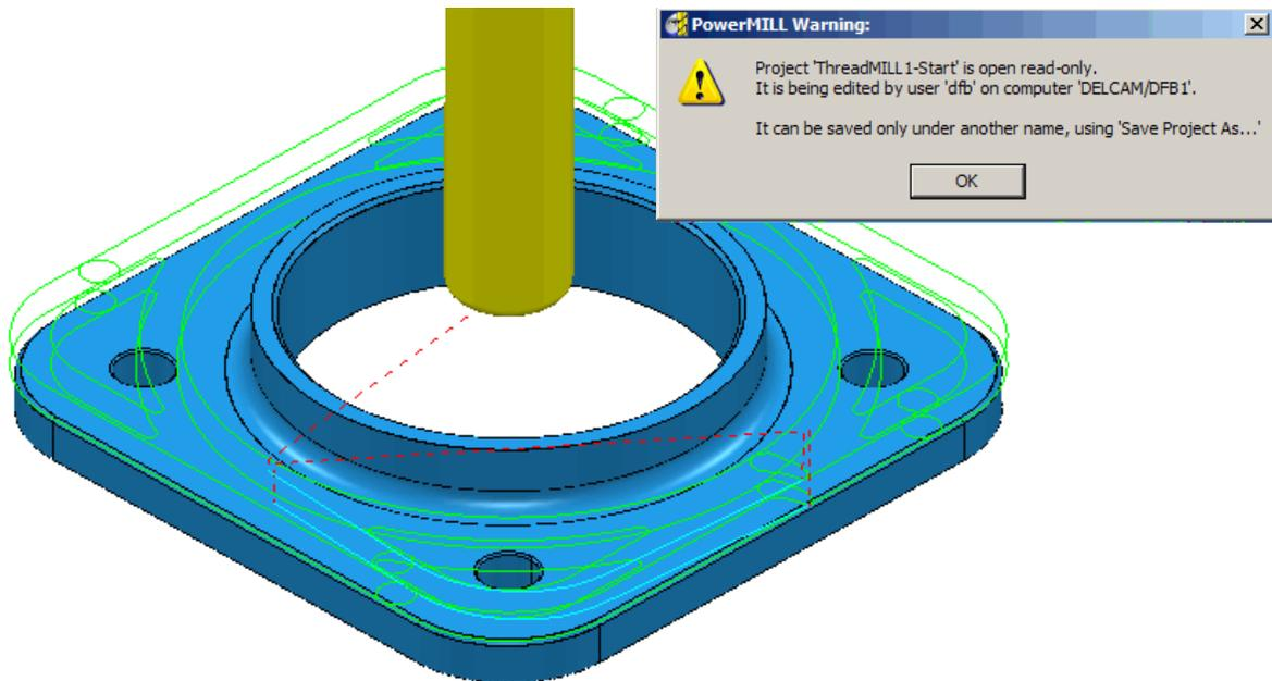
The imported **Project** basically contains a **Cad model**, a predefined **Hole Feature**, a **3D Offset Area Clearance** strategy using a **Tip Radius** cutter, and a **Thread Milling** tool. The original **Project** is **Locked** to prevent it from being altered, hence the first step is to **Save As** a separate **Project** locally with a different name.
