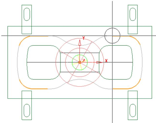
Note:-The **Tool Dia** and **Cross Hairs** are displayed on the **cursor**. This will provide an essential visual aid while **snapping** new **break points** along the **Pattern**.
