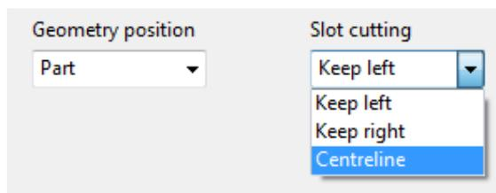
Width of Slot is achieved by creating *multiple toolpaths* that use the 3 different **Slot Cutting** options starting with **Centreline**.
