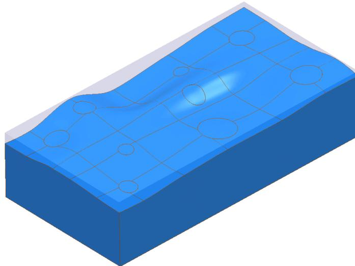
Note; the **Capping Surfaces** are automatically assigned to the new **Level** for easy selection.
