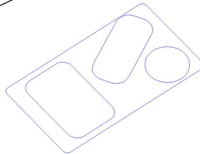
The **boundary** produced has 4 segments. For this example only the two smallest segments are required.
