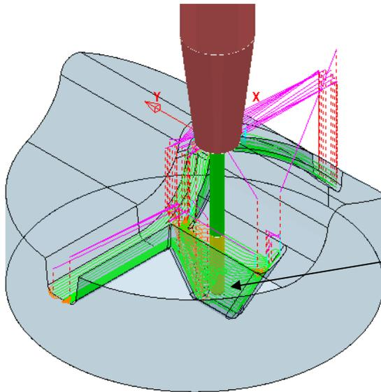
The **Corner Finishing** has operated all the way down to the base of the deep pocket. Due to the *excess stock* this could cause the cutter to break.
