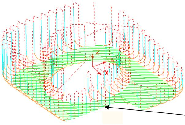
There is now a **Vertical Arc** leading onto most of the tool tracks. If the required **Lead Out** is to be exactly the same as the **Lead In** and vice versa the **Copy to Lead Out** option allows easy copying of the settings between the two. The **Leads** in this area have remained unchanged as any **Vertical Lead In/Out** using the current **Radius** value would **gouge** the **model** if allowed to appear.
