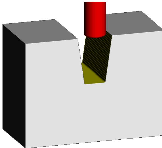
The **Roughing** strategy has not fully machined a large volume of **stock** towards the base of the slot. This will have to be removed as part of a **Constant Z finishing** strategy.
