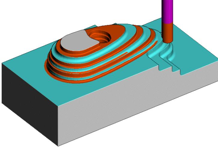
The **Rainbow ViewMILL Shading** option displays the resultant material removal for each **toolpath** as a different colour.
