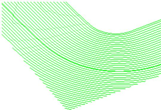
The **Pattern** segments have now taken over from the **Boundary** to *control* the actual toolpath shape.
