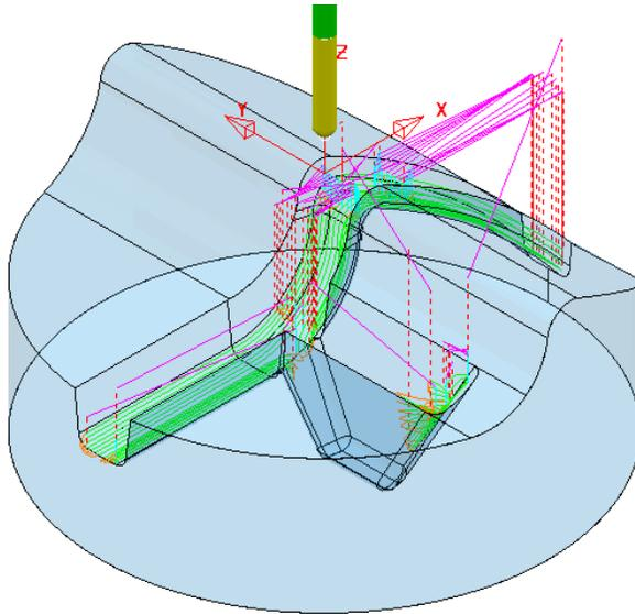
The **Corner Finishing** has not occurred in the deep pocket that is inaccessible to the **BN10** reference tool
