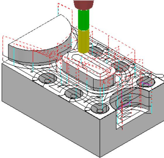
The **Model Area Clearance** toolpath now removes material locally across each **Flat** face leaving **0.6mm** stock (The **thickness** plus the **tolerance**).
