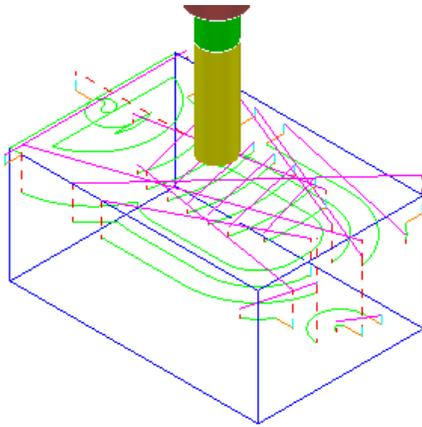
The **Flat** areas have been finish machined apart from between the 'D' shaped and oval **Bosses** as well as at the base of the **holes** due to the 20mm diameter tool being too large. We will now use a smaller tool to **Rest** machine these areas.
