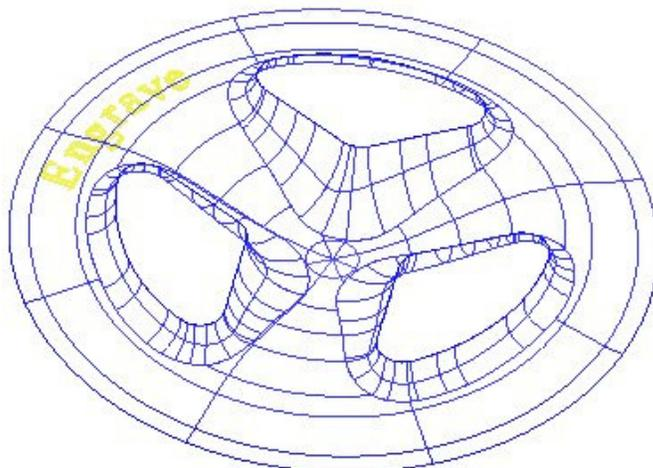
The **Pattern** is made up of **2D geometry** and is positioned at the bottom of the **Block**. This will be projected along **Z** through the **3D model** form to create a single **toolpath** with a negative **Thickness** value.
