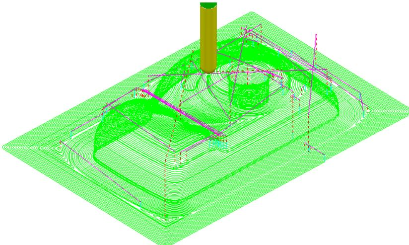
The user is able to control the angular threshold between the **3D Offset** and **Constant Z** components of the hybrid **Steep and Shallow finishing** strategy.
