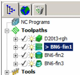
The **Project** contains 1 **Roughing toolpath** and 3 **Finishing toolpaths**. The following example will illustrate the retrospective addition of suitable **Leads and Links** to the 3 finishing toolpaths.
