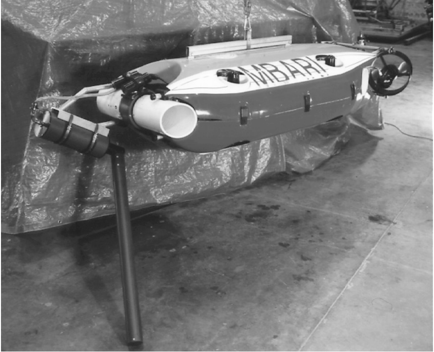
Fig. 7.1. OTTER vehicle developed in the Aerospace Robotics Laboratory at Stanford University (courtesy of T. McLain, Brigham Young University)
