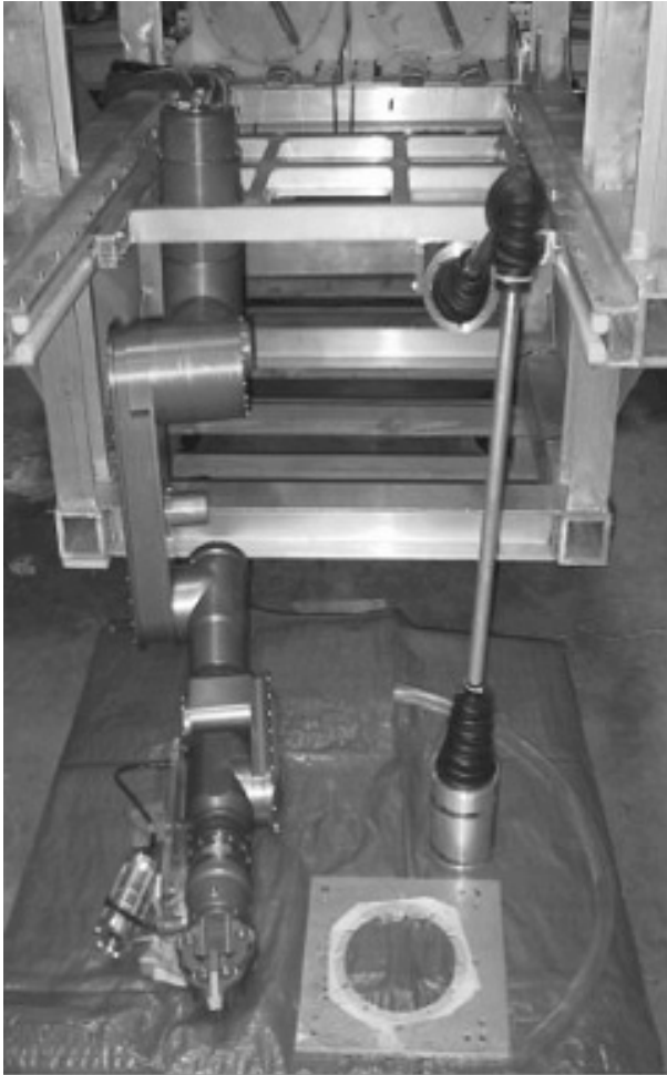
Fig. 7.4. SAUVIM under development and the Autonomous Systems Laboratory, University of Hawaii (courtesy of J. Yuh). The passive joint used for position measurement can be observed
