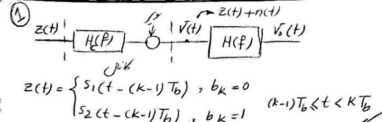
$z(t) = \begin{cases} s_1(t - (k-1)T_b), & b_k=0 \\ s_2(t - (k-1)T_b), & b_k=1 \end{cases} \quad (k-1)T_b \leq t < kT_b$
