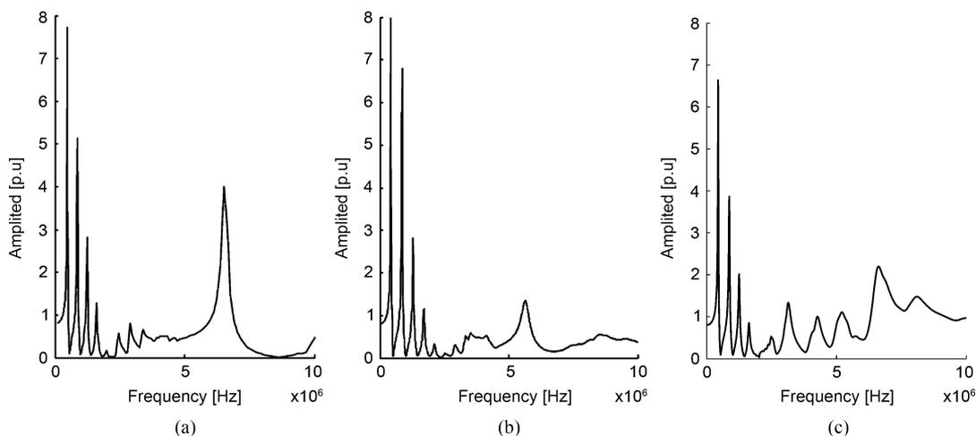
Fig. 4. Amplitudes of transfer function between the terminal of turn 40 and the input [(a) and (b) reprinted from [19]].
