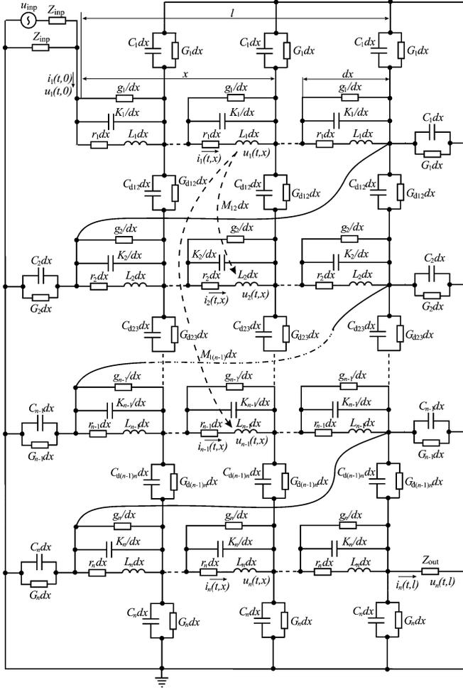
Fig. 1. Equivalent circuit of a disc-type transformer winding.
