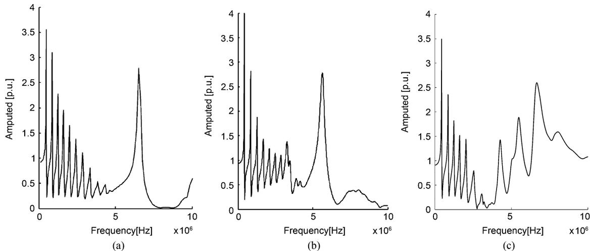
Fig. 3. Amplitudes of transfer function between the terminal of turn 20 and the input [(a) and (b) reprinted from [19]].
