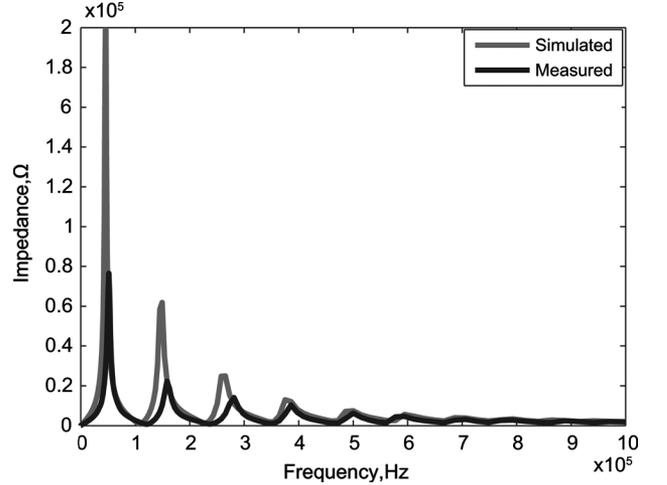
Fig. 2. Simulated with the proposed model and measured responses of open circuit impedance of the experimental transformer.
