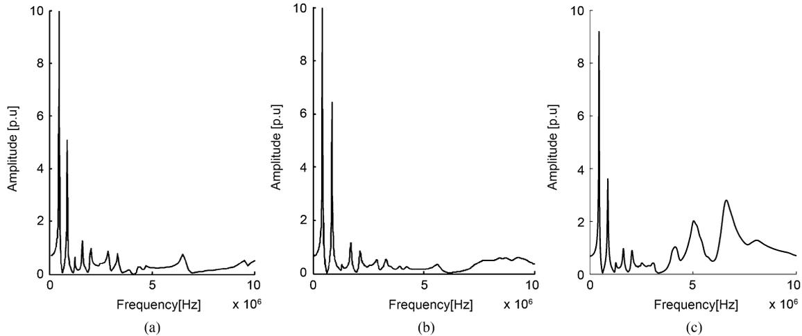
Fig. 5. Amplitudes of transfer function between the terminal of turn 60 and the input [(a) and (b) reprinted from [19]].
