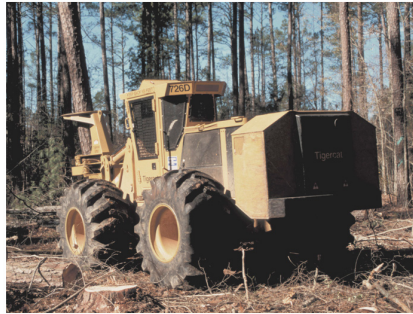
FIGURE 23: THE FELLING HEAD OF A FELLER-BUNCHER BY TIGERCAT, OF BRANDFORD, ONTARIO WAS DESIGNED IN SOLIDWORKS AND SIMULATED IN SOLIDWORKS MOTION AND SOLIDWORKS SIMULATION.
