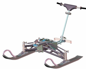
FIGURE 6: A FRONT-END SUSPENSION OF A SNOWMOBILE CONSISTS OF NUMEROUS LINKS INCLUDING SPRINGS AND DAMPERS.
