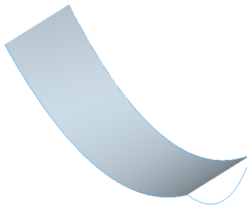
Figure 13-17 Boundary blend surface
