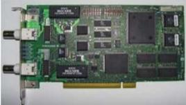
**Control Bus adapter (VF701) and RS-232 Serial Card (AIP261; in case of console type HIS) installed in the PCI slot.**
