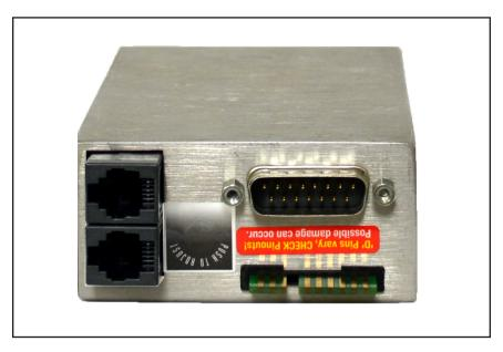
Figure 3-4 9000 Series Controller with 15-Pin D Connector and Cardedge Connector
