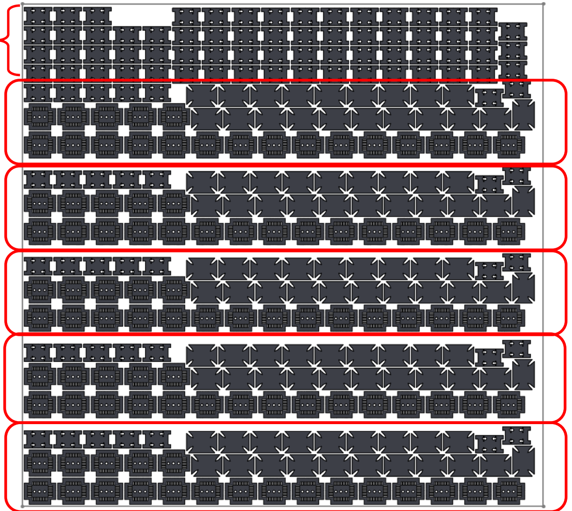
Nesting layout with 5 identical regions created using 5 tool heads
