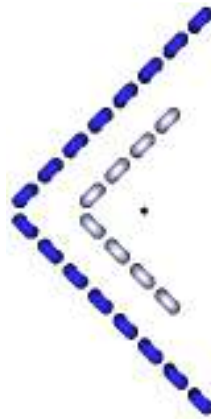
Figure 3.90 – CRA2 is ON ( L_2 is 8) and CRA1 is OFF at the same time (blue color represents activated element).
