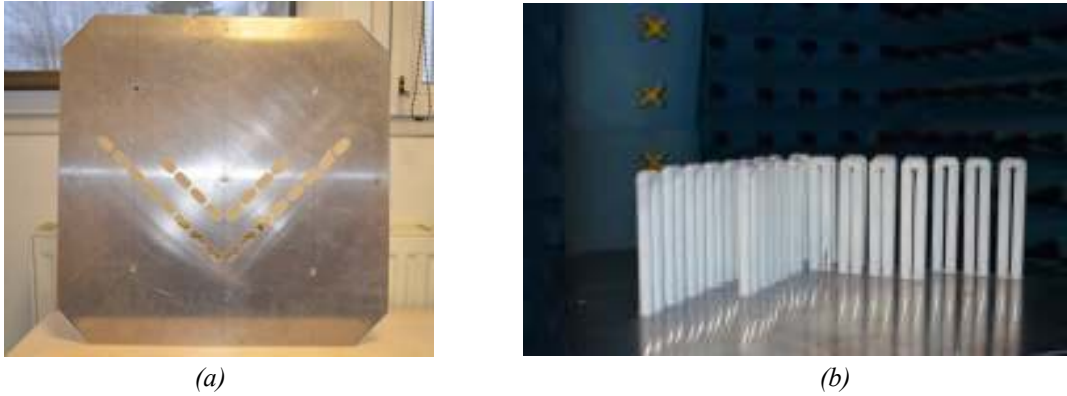
Figure 3.78 – CRA prototype. (a) 500 mm x 500 mm ground plane. (b) The 24 plasma elements with a monopole antenna in the center of the ground plane.
