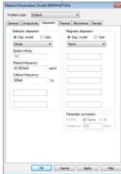
Figure 2.7 – Material parameter definition window in CST [23].
