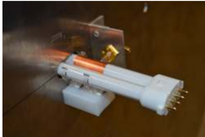
Figure 4.27 – Photographs of lower parts of the fabricated plasma antennas. (a) Plasma antenna with h_{\text{radiate}} = 77 mm. The inset shows a copper rod (17.5 mm) used to connect the SMA jack and copper sleeve. (b) Plasma antenna with h_{\text{radiate}} = 35.7 mm.
