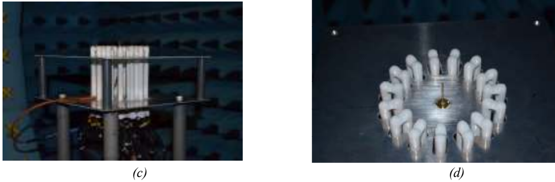
Figure 3.52– Photograph of the secondary ground plane and its equivalent RRA. (a)-(b) The h is 54 mm with the inserted secondary ground plane. (c)-(d) The h is 15 mm with the inserted second layer of the ground plane.
