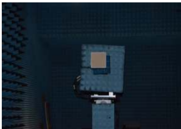
Figure 5.13 – Single horn antenna is being utilized during RCS measurement. The transmitter and the target are separated with a distance of 3.58 meter.
