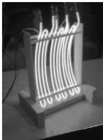
Figure 3.29 – Earliest design of plasma reflector [57].
