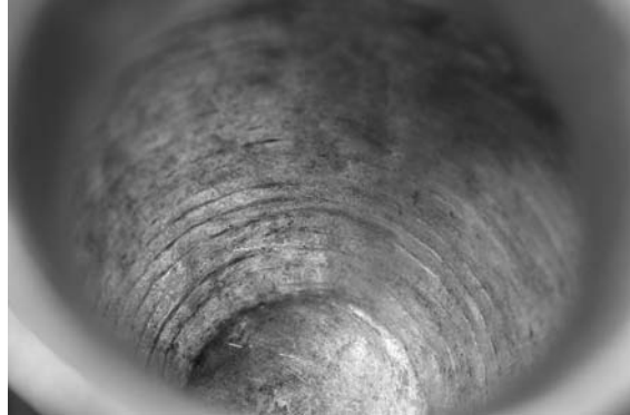
Fig. 36.18 Interior of jug: raw cast surface. (Photograph B. Armbruster)
