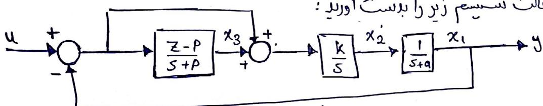
$$\begin{cases} x_1 = \left(\frac{1}{s+\alpha}\right)x_2 \\ x_2 = (u - x_1 + x_3) \frac{k}{s} \\ x_3 = \left(\frac{z-p}{z+p}\right)(u - x_1) \end{cases} \Rightarrow \begin{cases} sx_1 = -\alpha x_1 + x_2 \\ sx_2 = -kx_1 + kx_3 + ku \\ sx_3 = -(z-p)x_1 - px_3 + (z-p)u \end{cases}$$
