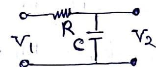
$$I(s) = \frac{V_1 - V_2}{R}, \quad V_2 = \frac{I(s)}{Cs}$$
