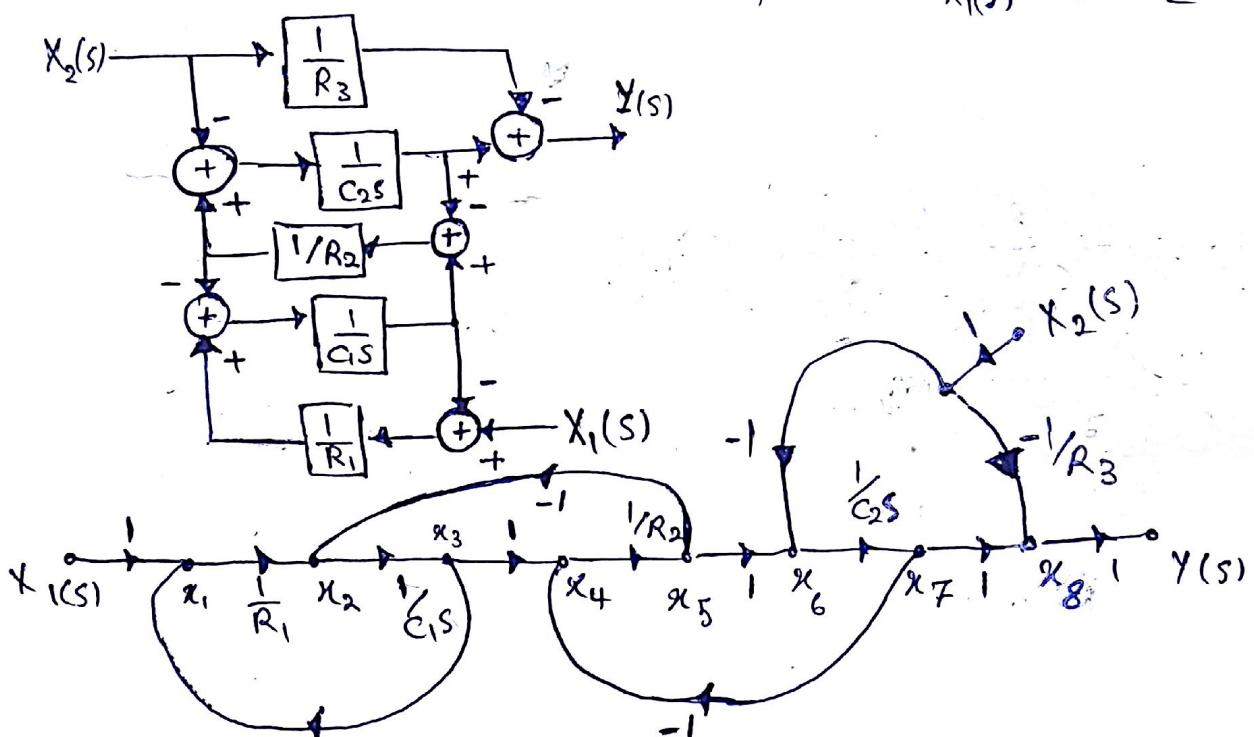
$$\frac{Y(s)}{X_1(s)} = \frac{\sum_{k=1}^N P_k \Delta_k^{-1}}{\Delta}, \quad P_1 = \frac{1}{R_1} \times \frac{1}{C_1 s} \times \frac{1}{R_2} \times \frac{1}{C_2 s} \quad \Delta_1 = 1$$
