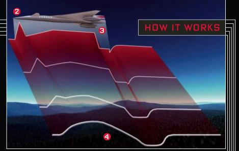
WAVE FORM Sonic booms happen when pressure builds up too fast around wings and engines. In a conventional boom [right], the pressure migrates forward and backward. That movement generates two pressure spikes at the front and rear, creating a classic N-shaped-wave [1], and the result is a loud double bang. To soften the boom, QSST aerodynamicists sought to spread out the pressure points along the fuselage [left]. The new aircraft [above] generates
