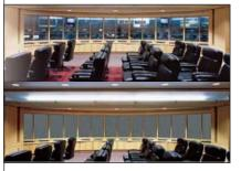
**PRIVACY GLASS Liquid crystals have** the fluidity of a liquid but the ordered structure of a solid. In privacy glass, applying an electrical charge causes the molecules to switch from a random, light-admitting arrangement to an orderly, light-blocking one.
