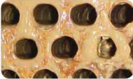
Biofilm on a heat exchanger tube sheet
