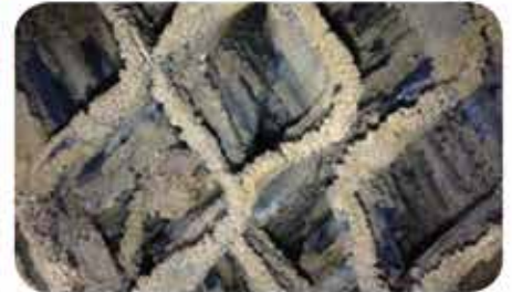
Scale embedded in biofilm on tower pack
