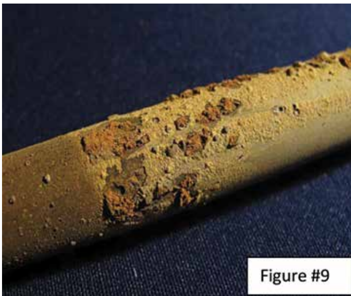
Several deep pits were revealed under the deposits on Exchanger Tube #2 where tubercles were removed as shown in Figures #8 & #9.
