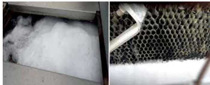
Figure 10: CMIT/MIT Surfactant C formulation causes excessive foaming during field trial testing.
