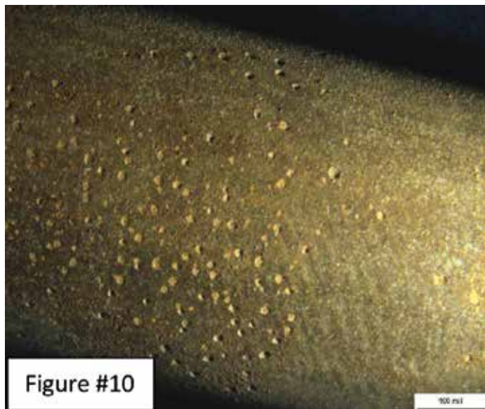
Several deep pits were revealed under the deposits on Exchanger Tube #2 where tubercles were removed as shown in Figures #8 & #9.
