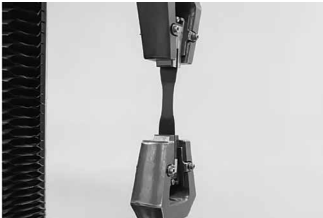
Figure 8: Lab Test, Coupon in Tension [7]
