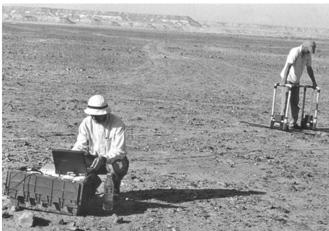
Figure 10.3 PulseEKKO radar unit in field use. The aerials are to the right, the CRU is in the foreground on the left. (Reproduced by permission of Dr C. Bristow.)
