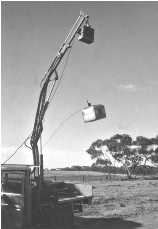
Figure 11.3 Impact source. A half-ton weight being dropped from a portable crane during a survey of the low-velocity layer.
