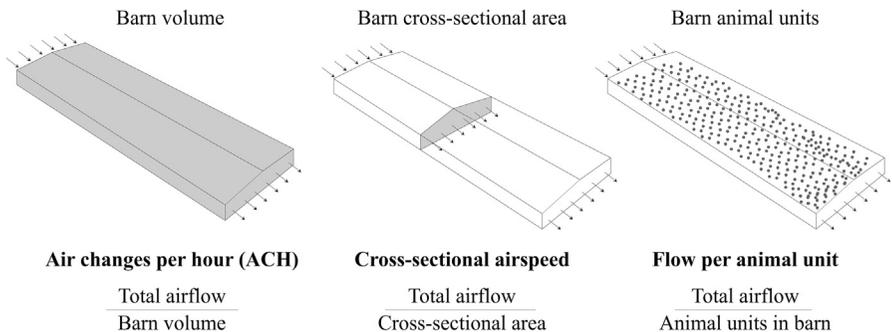
**Fig. 1.** Three key ventilation parameters comparing the total flow to the barn’s volume, cross-sectional area, and number of animals.
