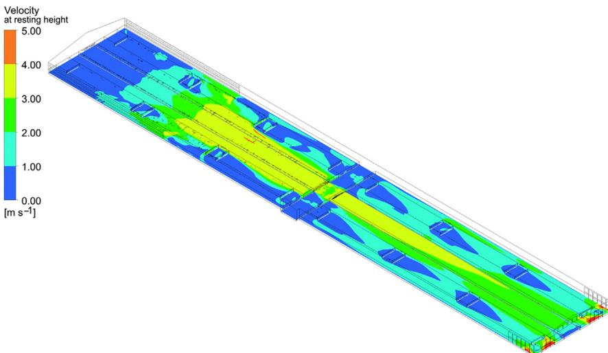
Fig. 4. Computational fluid dynamics model of a tunnel-ventilated barn at 41 ACH.
