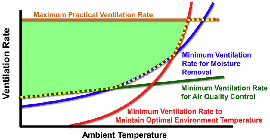
Fig. 12. The ideal ventilation design curve. (Adapted from Christianson LL. Ventilation - energy and economics - Figure 14.2. In: Hellickson MA and Walker JN, editors. Ventilation of agricultural structures. St. Joseph (MI): American Society of Agricultural Engineers; 1983. p. 336; with permission.)
