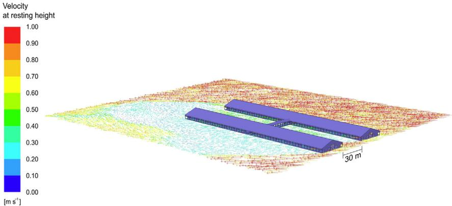
**Fig. 2.** Computational fluid dynamics results of natural ventilated barns separated by 30-m distance and the resulting velocity vectors at  $1 \text{ m s}^{-1}$  in a  $45^\circ$  direction.
