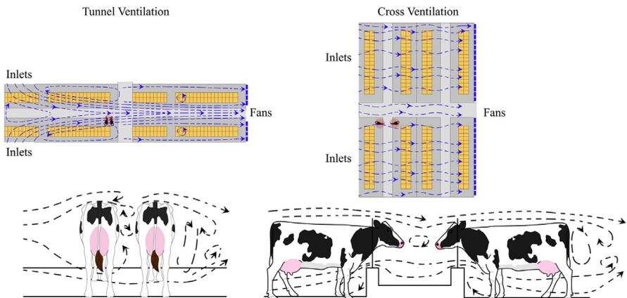
**Fig. 3.** Typical flow profiles for tunnel-ventilation (*left*) and cross-ventilation (*right*) systems; tunnel ventilation flows (*left*) parallel to the feed lane. Cross-ventilation (*right*) flows perpendicular to the feed lane.
