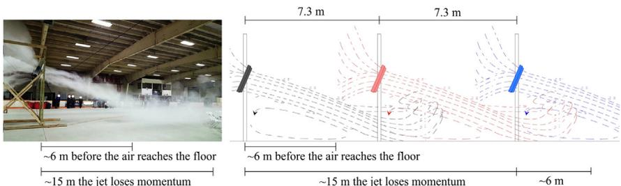
**Fig. 7.** A 54-inch fan smoking trial (*left*) and fans installed at 7.3 and 14.6 m from each other (*right*). If the red fan was not included, the black fan's jets would not reach the 6-m zone of still air in front of the blue fan.
