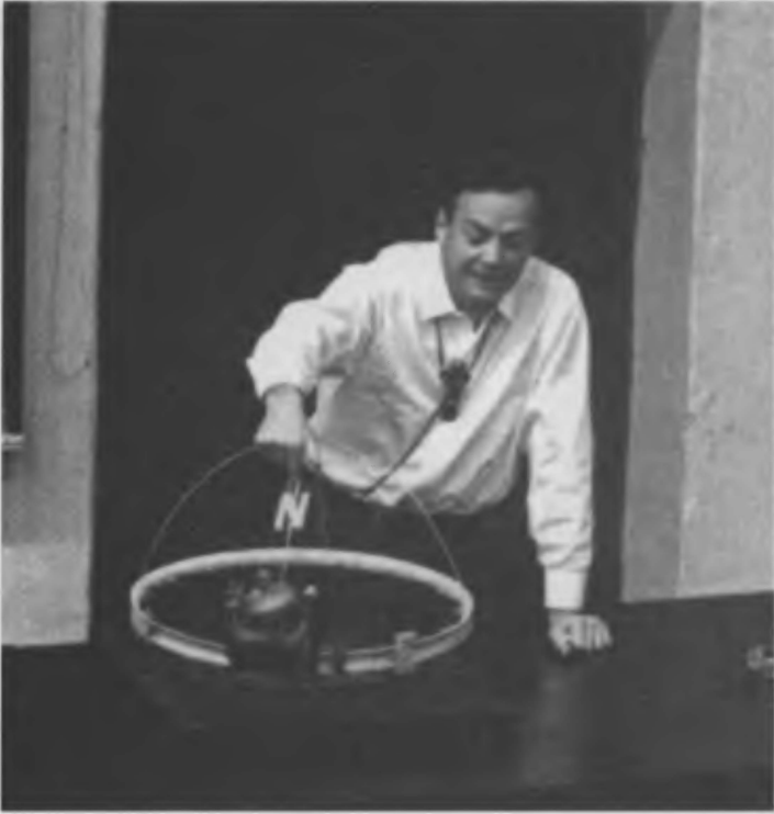
FIGURE 4-9 Feynman demonstrates an artificial gyrocompass.
