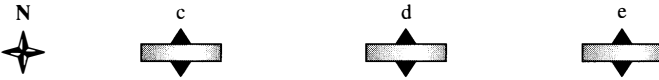
FIGURE 4-8 A gyrocompass with its spin axis parallel to Earth's tends to stay that way.
