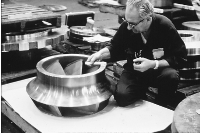
FIGURE 12.49 Mixed-flow impeller. ( Dresser-Rand Company, Olean, N.Y. )
