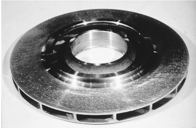
FIGURE 12.104 Two-piece impeller with integrally milled blades. ( Dresser-Rand Company, Olean, N.Y. )
