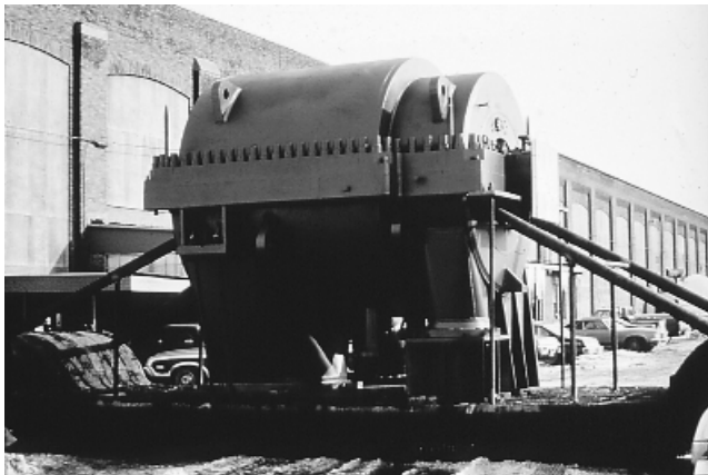
FIGURE 12.83 Centrifugal compressor with a fabricated casing. ( Dresser-Rand Company, Olean, N.Y. )
