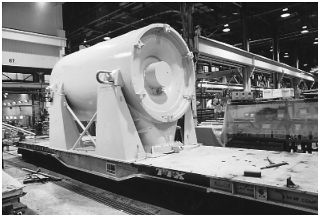
FIGURE 12.2 Radially split compressor with a shear-ring head closure. ( Dresser-Rand Company, Olean, N.Y. )
