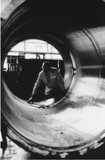
FIGURE 12.80 Compressor casing bore. ( Dresser-Rand Company, Olean, N.Y. )
