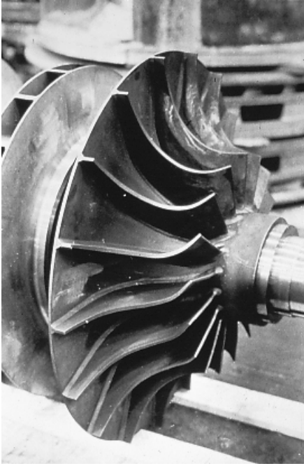
FIGURE 12.102 Three-dimensional, welded impeller. ( Dresser-Rand Company, Olean, N.Y. )
