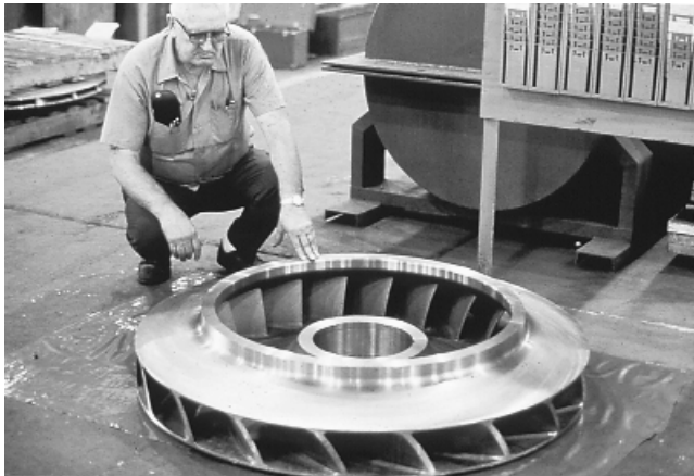
FIGURE 12.43 Three-piece welded impeller. ( Dresser-Rand Company, Olean, N.Y. )
