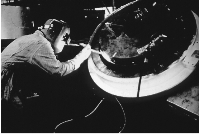
FIGURE 12.109 Impeller undergoing semiautomatic welding. ( Dresser-Rand Company, Olean, N.Y. )
