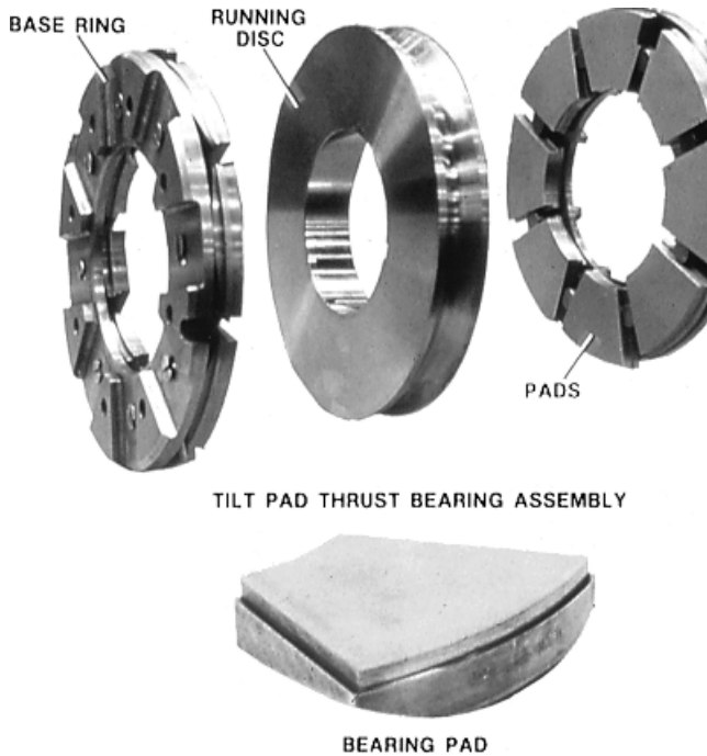
FIGURE 12.65 Thrust bearing assembly. ( Dresser-Rand Company, Olean, N.Y. )
