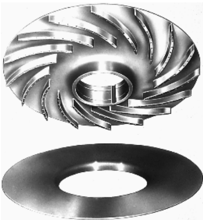
FIGURE 12.41 Integrally riveted impeller. (Dresser-Rand Company, Olean, N.Y.)
