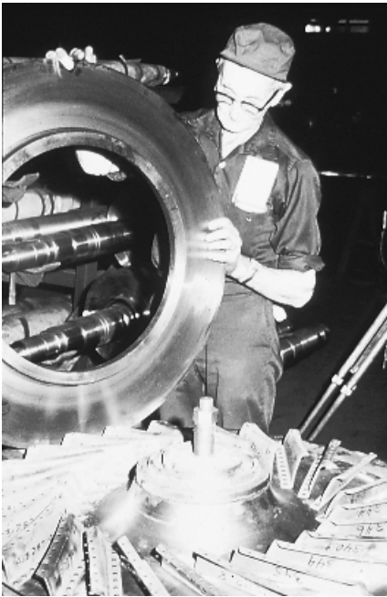
FIGURE 12.40 Riveted impeller, Z-type blading. (Dresser-Rand Company, Olean, N.Y.)
