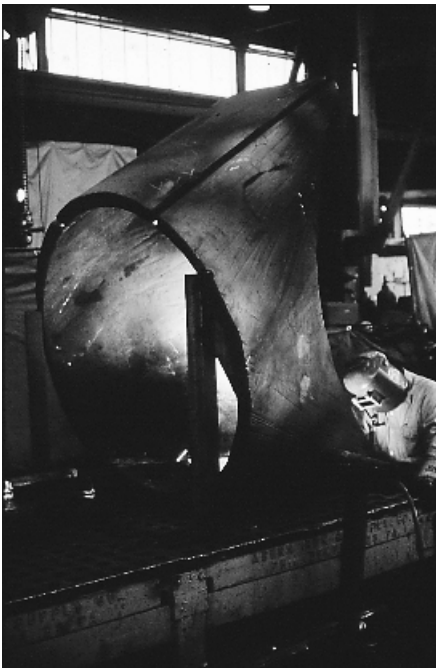
FIGURE 12.85 Nozzle welding in progress. ( Dresser-Rand Company, Olean, N.Y. )
