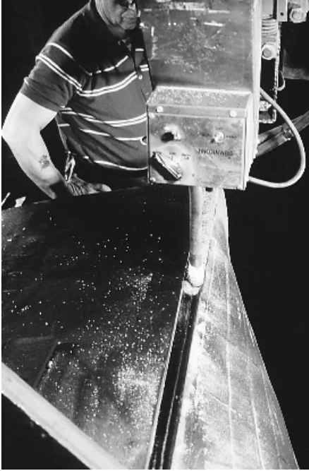
FIGURE 12.86 Automatic submerged arc welding. ( Dresser-Rand Company, Olean, N.Y. )
