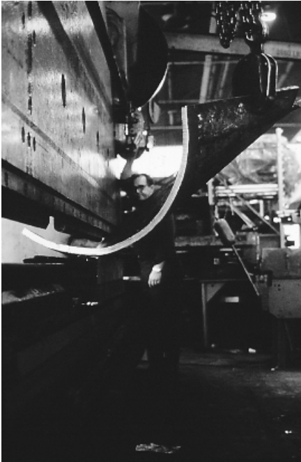
FIGURE 12.84 Straight-line brake bending produces a cylindrical casing contour. ( Dresser-Rand Company, Olean, N.Y. )
