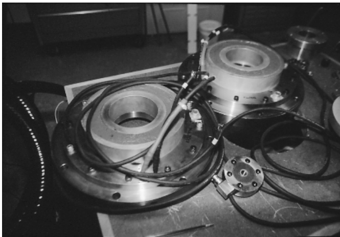
FIGURE 13.10 Axial magnetic bearing stator. ( Revolve Technologies, Calgary, Alberta, Canada )
