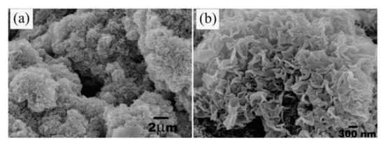
**FIGURE** 4 | (a) Low-magnification FEG–SEM image of loose graphene nanosheet (GNS) powders. (b) High-magnification FEG–SEM view of GNS petals. (Reprinted with permission from Ref 47. Copyright 2010, Elsevier.)
