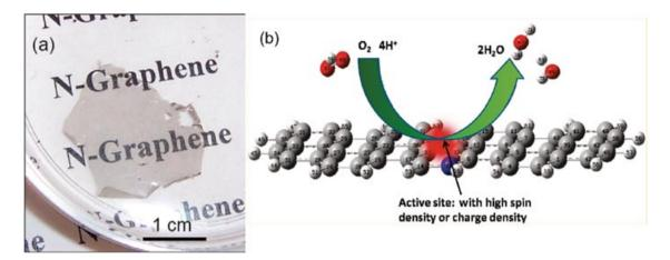
**FIGURE 11** (a) Digital photo image of transparent nitrogen-doped graphene film floating on water after removal of the nickel layer by dissolving in an aqueous acid solution. (b) The electrocatalytical mechanism of nitrogen-doped graphene in acidic environment. (Reprinted with permission from Refs 99 and 100. Copyright 2010 and 2011, American Chemical Society.)
