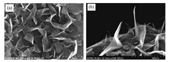
**FIGURE 3** | (a) Scanning electron microscopy (SEM) micrograph of coated Ni electrode. (b) SEM micrograph of a coated fiber, showing plan and shallow-angle views. (Reprinted with permission from Ref 31. Copyright 2010, AAAS.)
