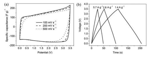
**FIGURE 2** | Supercapacitor performance of a-MEGO (SSA  $\sim$  2400 m<sup>2</sup> g<sup>-1</sup>) in the BMIM BF<sub>4</sub>/AN electrolyte. (a) CV curves at different scan rates. Rectangular shapes indicate the capacitive behavior. (b) Galvanostatic charge–discharge curves of a MEGO-based supercapacitor under different constant currents. (Reprinted with permission from Ref 29. Copyright 2011, AAAS.)
