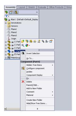
Automatically the software will assume some motion constraints according to the assembly mate constraints that have been created. These motion constraints have to be checked.
