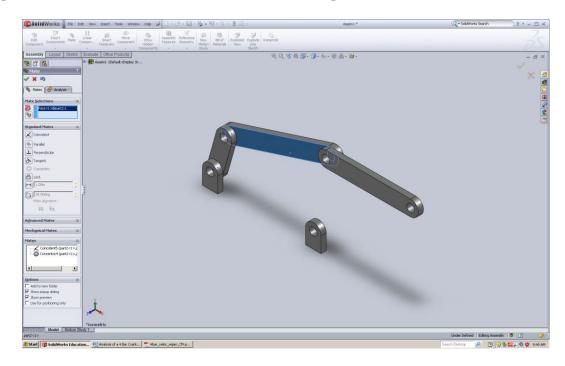
Select the internal faces of coincident holes and click concentric, repeat the procedure for the constraints between the third bar and the second support.
