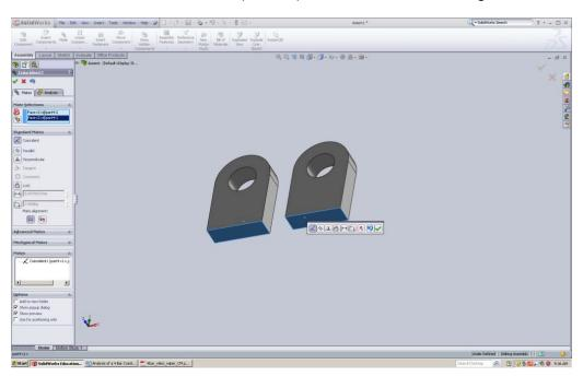
Click any single point or vertex on the support. Then, hold shift and click the same point on the other support. Create a distance mate that satisfies the dimensional constraints of the crank rocker mechanism. This defines the length of the ground link. For example, you could click these two vertices.
