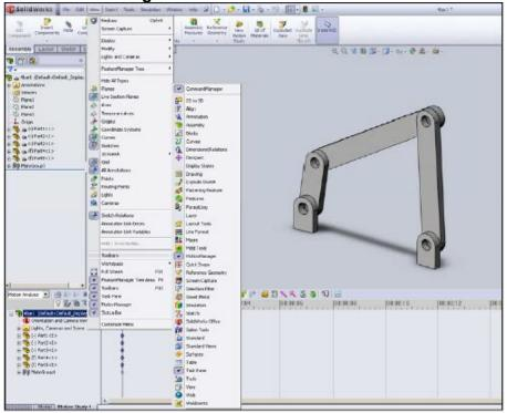
If the supports are already fixed, a lowercase 'f' will appear next to the part name in the parts tree and no further action is necessary.
