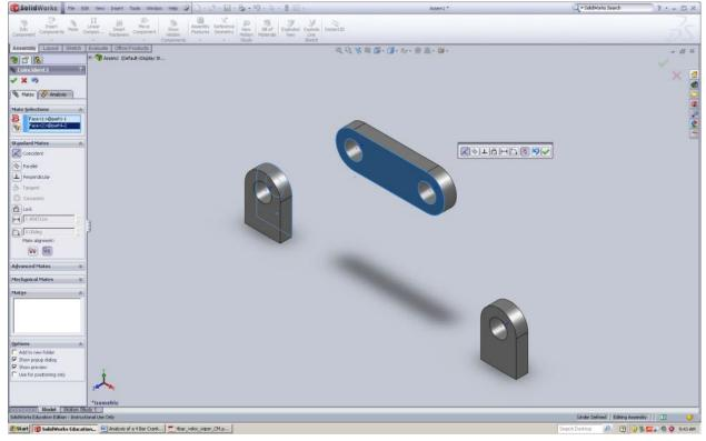
Now, select the internal faces of the holes (the bar and support), and select the concentric button, click the move component button and select the bar and move it to the best position to assemble the next one:
