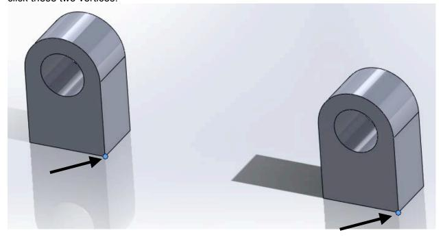
On this page, take note of the location of the distance mate button (Mate  $\rightarrow$ Advanced mates). Your distance is allowed to be different than as shown in the figure. A distance of "6" may not work with the lengths you chose for your links.
