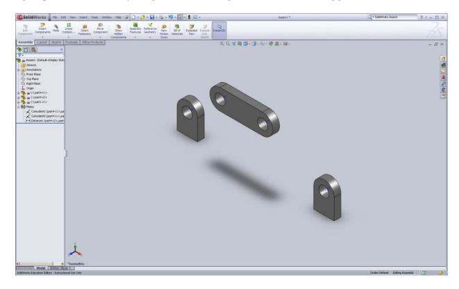
Select the opposite face of the **support** part (keeping the above graphic as reference), and the front face of the bar, and click on the coincident button:
