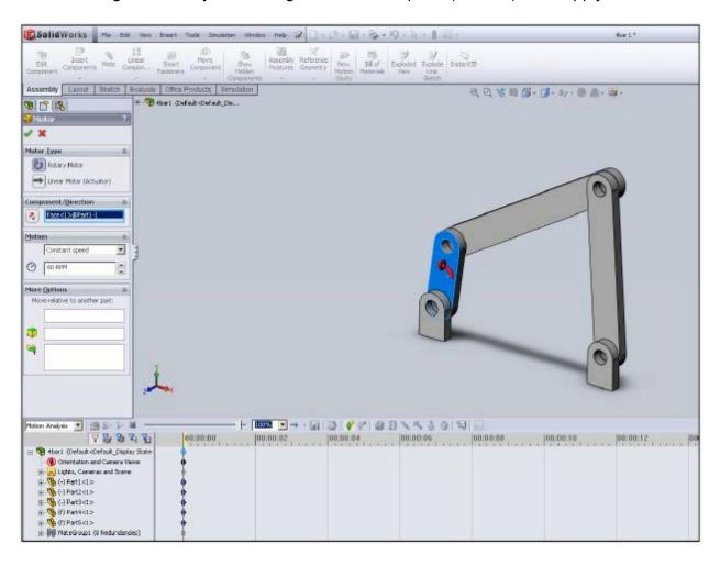
Click on the results button - the results menu opens on the left. In the three drop down menus, select **Displacement/Velocity/Acceleration**, **Linear Velocity** and **X-Component**. Select the coupler (**part2**), and click the check mark.
