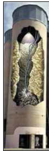
FIGURE 9. Giro whips are powered by compressed air and manipulated by operators
