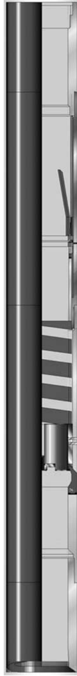
FIGURE 7.3 Type "A" Outside Mechanical Cutter. (Courtesy Weatherford International)
