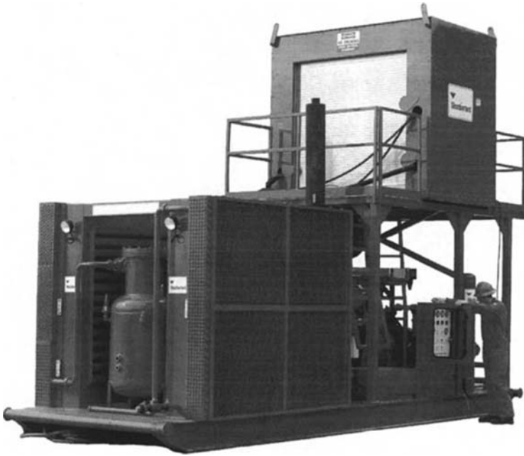
FIGURE 3.8 Sea Wolf combined primary compressor and inert air generation unit (Courtesy of Weatherford International Limited).
