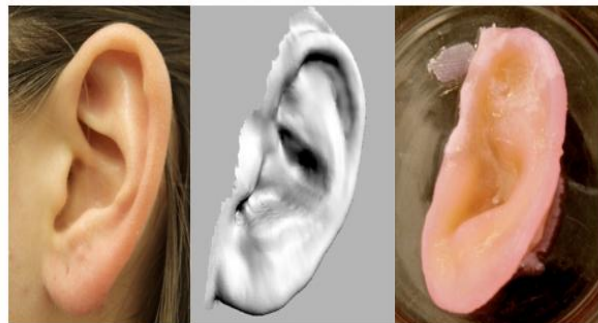
Figure: Image-based tissue engineering of human ear cartilage. Comparison of photograph (left), digitized image (middle), and tissue engineered ear cartilage after two weeks in culture.
