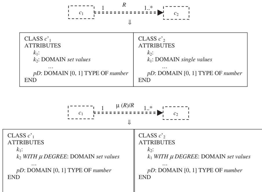
Fig. 10. Transformation of the associations in the fuzzy UML to the fuzzy object-oriented database schema.
