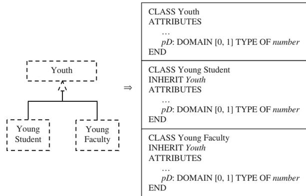
Fig. 8. Transformation of the subclasses in the fuzzy UML to the fuzzy object-oriented database scheme.
