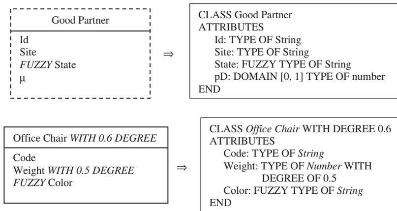
Fig. 7. Transformation of the classes in the fuzzy UML to the fuzzy object-oriented database scheme.
