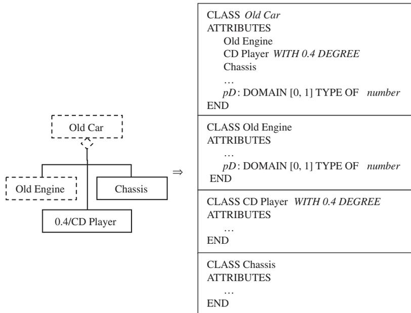
Fig. 9. Transformation of the aggregations in the fuzzy UML to the fuzzy object-oriented database scheme.
