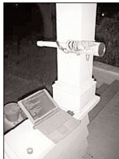
Figure 10-5 Pringles Can Used as a Yagi Antenna
