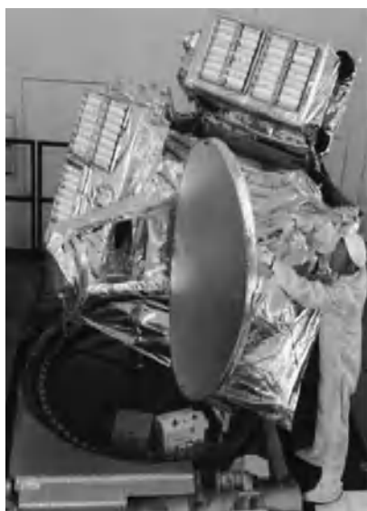
Figure 7.17 Photograph of the first spaceborne microwave limb sounder on NASA's UARS satellite and diagram of its quasi-optics radiometers [39]. Courtesy of NASA/JPL-Caltech.
