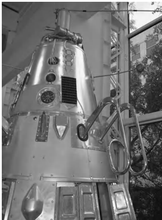
Figure 7.3 Sputnik III with element of the 66 MHz turnstile antenna. Reproduced by permission of Sven Grahn.
