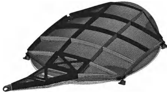
Figure 5.16 Ka-Sat 2.6 m antenna reflector FE model. First eigenmode shape superposed on FEM mesh. Courtesy of EADS-CASA.
