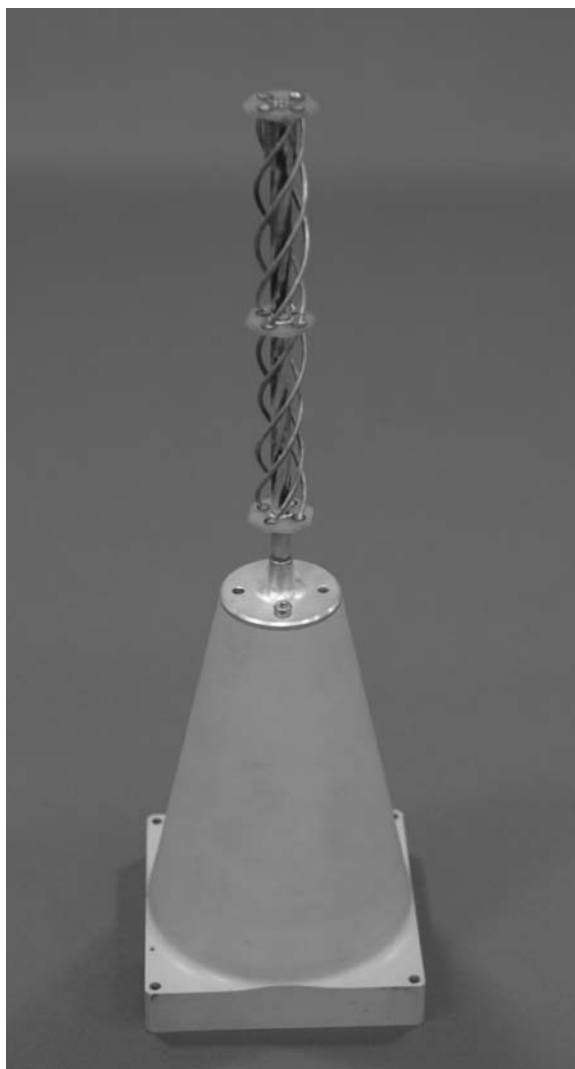
Figure 15.13 A space-qualified quadrifilar helix antenna. Courtesy of Surrey Satellite Technology Ltd, UK [4].
