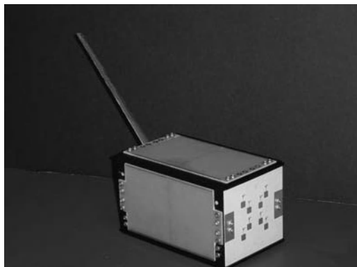
Figure 15.26 Circularly polarized, cross-shaped, microstrip patch retro-directive array mounted on one face of a CubeSat. The resonant frequency is 10.5 GHz [14]. © 2005 IEEE. Reprinted, with permission from Proceedings of the IEEE/ACES International Conference on Wireless Communications and Applied Computational Electromagnetics , Honolulu, HI, April 2005, pp. 606–609.
