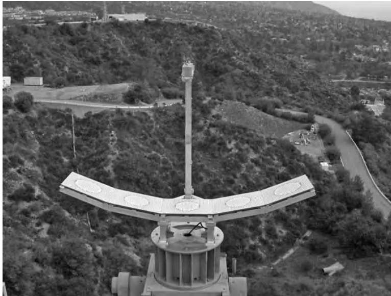
Figure 10.24 Photo of the piecewise flat reflectarray for WSOA in Ku-band. Courtesy of Dr. John Huang, retiree from JPL, Reproduced by permission of John Wiley & Sons, Inc.[71].
