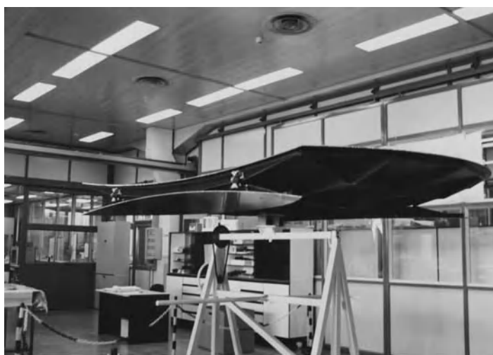
Figure 7.36 The 4 m hinged-tip reflector. Courtesy of Thales Alenia Space Italia.
