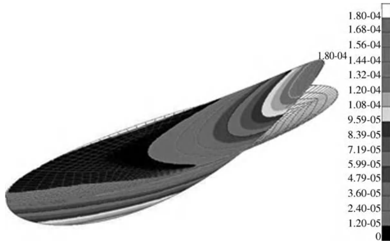
Figure 5.31 Distortions of 5 mm core CFRP skins (layup2) parabolic reflector with temperature transverse gradient case. Displacements in m.
