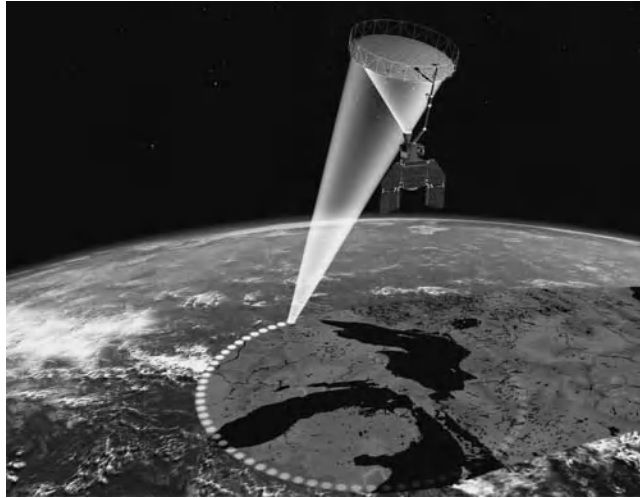
Figure 8.8 An artist's rendition of the SMAP spacecraft. The 6 m deployable mesh reflector is designed to spin at an approximate rate of 14 rpm, creating a 1000 km swath on the ground. The reflector will be shared between the radar, with a center frequency of 1.26 GHz, and the radiometer, operating at 1.41 GHz. Courtesy of NASA.
