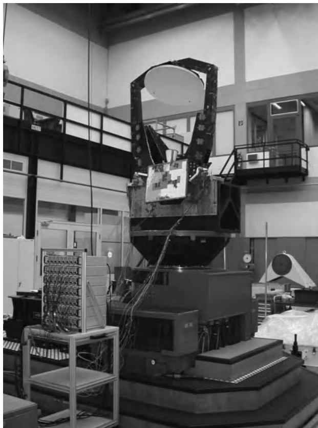
Figure 6.34 Vibration test setup of top-deck antenna for vertical test axis; moving coil shaker system of 500 kN with mounted test antenna at adapter cube.
