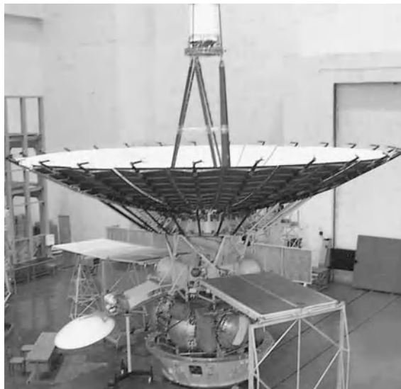
Figure 16.16 RadioAstron antenna in deployed configuration. The spacecraft bus, solar cells, and telemetry antenna are seen below the 10m diameter primary reflector. Reproduced with permission by N. Kardashev.
