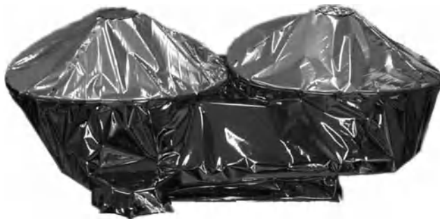
Figure 5.33 SIRAL antenna subsystem of CryoSat under thermal tent. Courtesy of RUAG Space AB, Sweden, under ESA contract.
