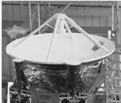
Figure 7.43 MARECS satellite (1981) with shaped reflector. Courtesy of ESA.
