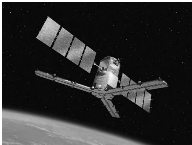
Figure 7.66 SMOS satellite and its Microwave Imaging Radiometer MIRAS. Courtesy of ESA – P. Carril.
