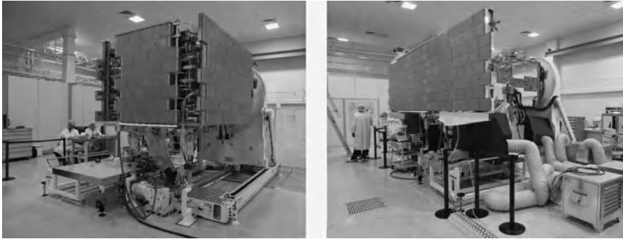
Figure 13.11 COSMO SkyMed active SAR antenna (stowed and deployed). Courtesy of ASI and Thales Alenia Space Italia.
