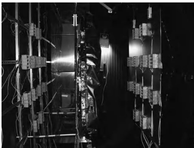
Figure 6.32 Thermal vacuum chamber with solar simulator by IR radiator array.
