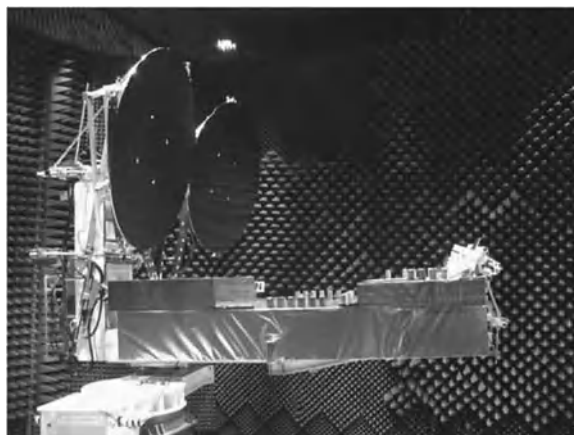
Figure 12.16 Ka-band multibeam antennas in the compact RF test range. Reproduced by permission of MDA.
