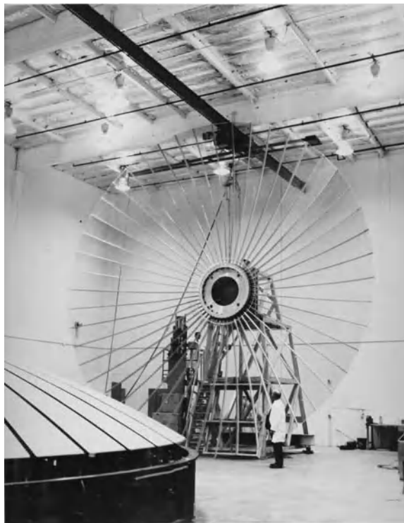
Figure 8.1 Photograph of NASA's ATS-6 satellite. The 9.1 m diameter telecommunications antenna, built by Lockheed Missile and Space Company, operated at multiple frequency bands from VHF to C-band. The satellite operated in a geosynchronous orbit for five years and demonstrated several new technologies, including direct-broadcast television. Courtesy of NASA.
