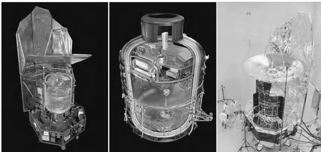
Figure 16.11 Left: the Herschel spacecraft showing the solar panel/sunshield (solar panels facing away), telescope, cryostat, and service module with the warm electronics. Middle: cutaway of the cryostat showing the three focal plane instruments at the top with the liquid helium reservoir below. Right: Herschel being prepared for acoustic testing. From Pilbratt et al. 2010, A&A , 518 , L1 [41]. Reproduced with permission © ESO.
