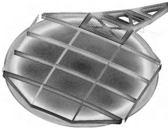
Figure 5.22 Ka-Sat 2.6 m antenna reflector. Acoustic RMS pressure computed with BEM VA-One. Courtesy of EADS-CASA under ESA ARTES contract.
