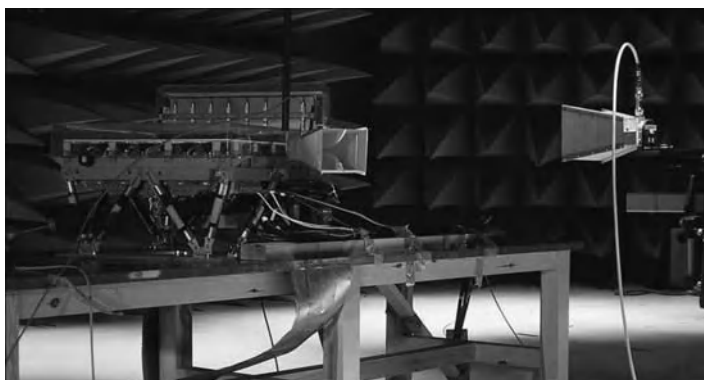
Figure 9.24 Active antenna during EMC testing. Reproduced by permission of EADS CASA Espacio.
