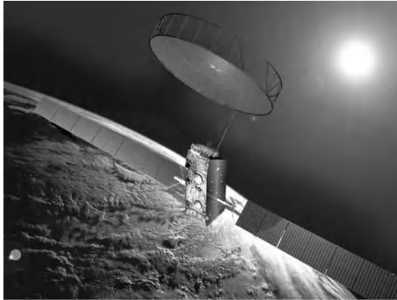
Figure 12.4 INMARSAT-4 satellite with unfurlable reflector. Reproduced by permission of Inmarsat.
