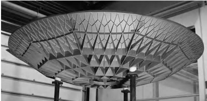
Figure 5.4 Example of monolithic stiffened shell reflector. Herschel telescope 3.5 m M1 rear view. Courtesy of EADS Astrium, under ESA contract.
