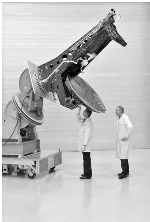
Figure 12.11 Deck-mounted steerable Ku-band Gregorian antenna. Reproduced by permission of MDA.
