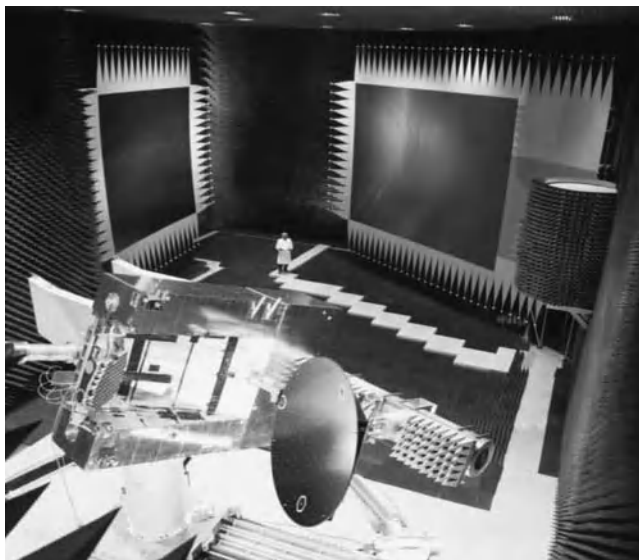
Figure 6.19 A compensated compact range of the Cassegrain type.
