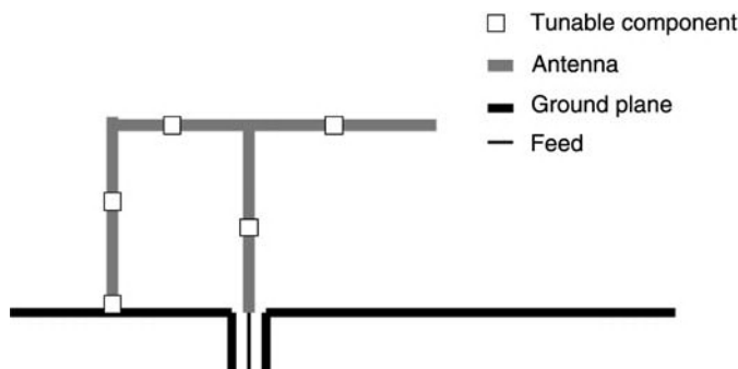
Figure 15.27 An example of an exciter which uses an inverted-F antenna [15].
