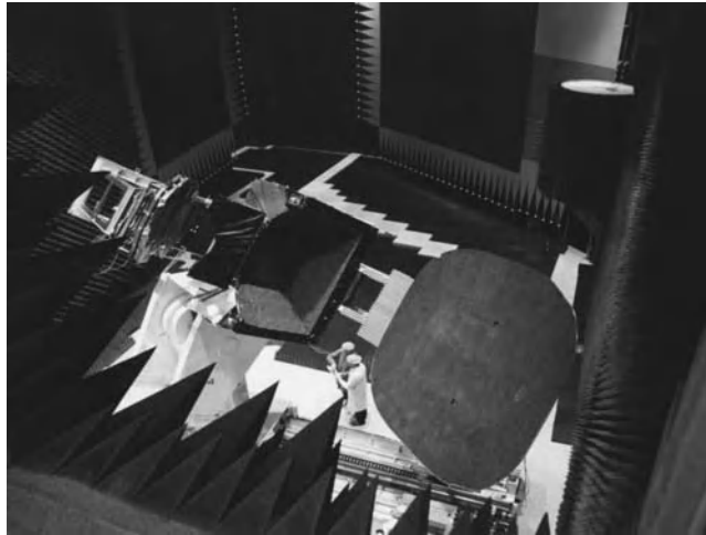
Figure 6.8 Transmit antenna including mock-up installed in the CCR75/60 of EADS Astrium.
