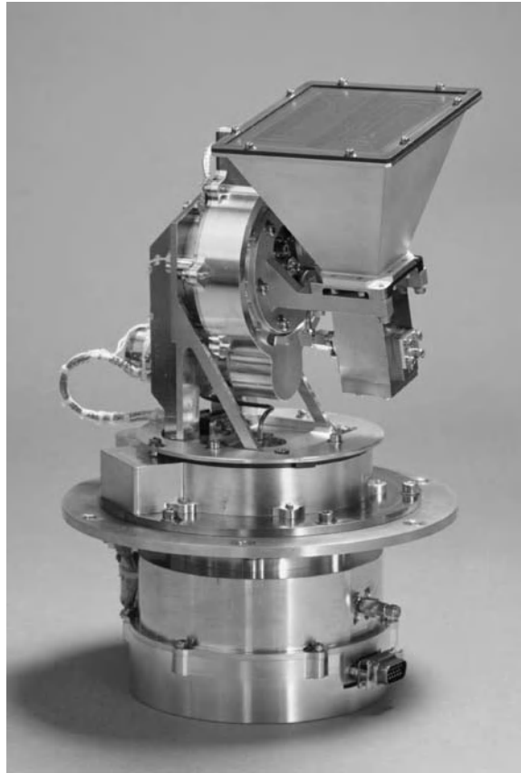
Figure 15.14 Small-satellite antenna pointing mechanism with horn antenna. Courtesy of Surrey Satellite Technology Ltd, UK [4].
