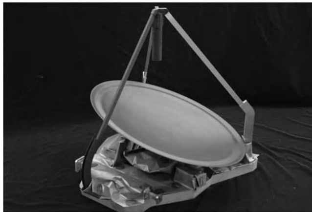
Figure 12.23 Steerable ground link antenna. Reproduced by permission of MDA.
