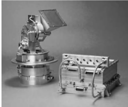
Figure 15.29 A complete tracking X-band transmitter. Courtesy of Surrey Satellite Technology Ltd, UK [4].
