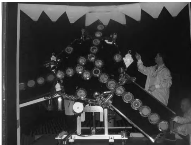
Figure 6.47 Dry-run test of the MGSE and test setup of MIRAS in the DTU Antenna Test Facility.
