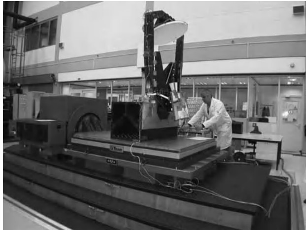
Figure 6.33 Vibration test setup of top-deck antenna with horizontal test axis; moving coil shaker system (left side) and lateral moving slip table (with specimen).
