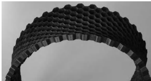
Figure 5.14 Carbon fibre honeycomb core. Courtesy of HPS and Invent GmbH, under ESA contract.
