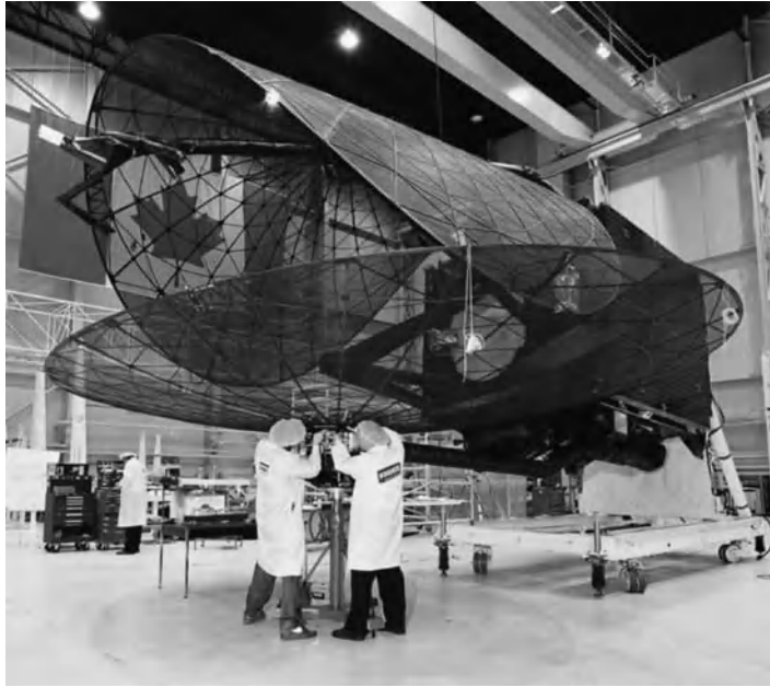
Figure 7.28 Hughes Springback reflector. Courtesy of Canadian Space Agency www.asc-csa.gc.ca .
