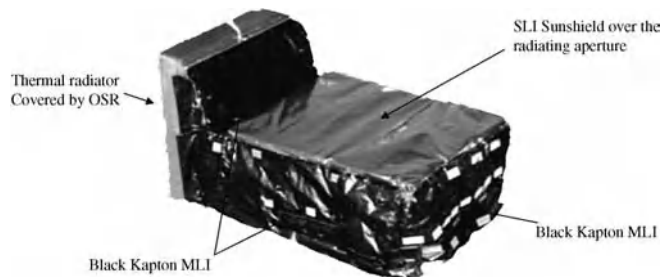
Figure 9.21 External thermal control of an active antenna (OSR=Optical Solar Reflector). Reproduced by permission of EADS CASA Espacio.
