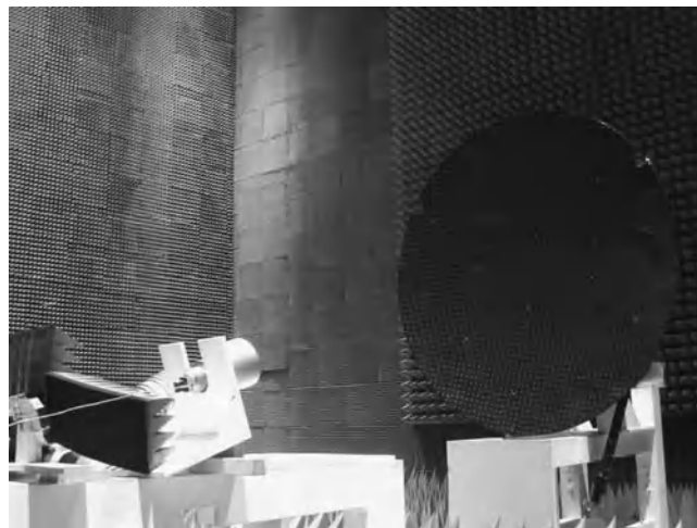
Figure 6.37 PIM setup with wooden MGSE and anechoic environment.
