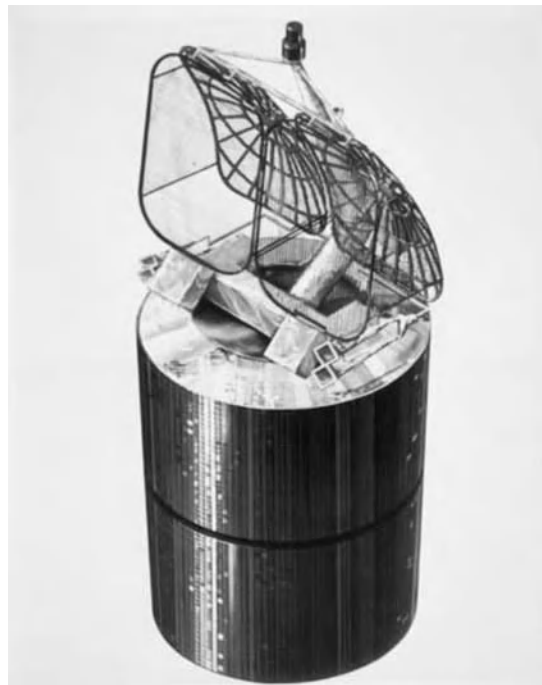
Figure 7.40 COMSTAR 1 antennas with polarization screens. Courtesy of NASA.
