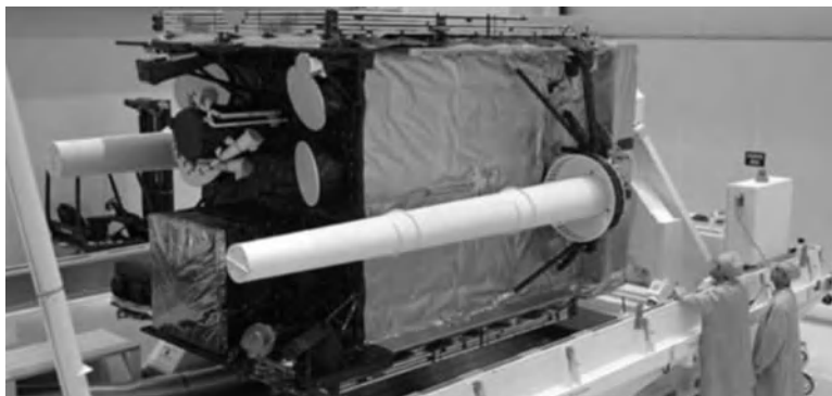
Figure 12.2 Deployable rigid helices, with separate Tx and Rx. Reproduced by permission of Astrium.
