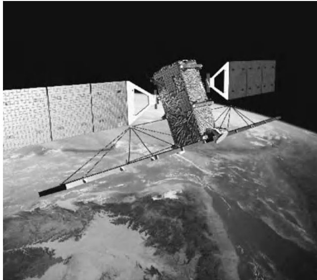
Figure 7.65 Radarsat 2 and its 15 \times 1.5 m C-band antenna. Courtesy of MDA – Eric Amyotte.
