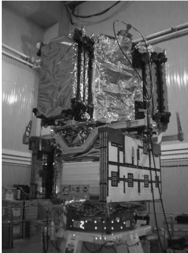
Figure 6.44 SMOS payload during AIT activities at the Plestezk launch site. MIRAS arms and PROTEUS solar panels stowed. Protective Ge Kapton foils cover the payload.
