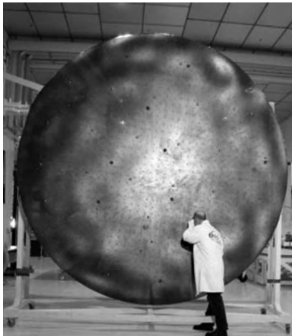
Figure 5.5 Example of ultralight reflector: ASAS 3.8 m shaped reflector. Courtesy of Astrium-ST, under ESA contract.
