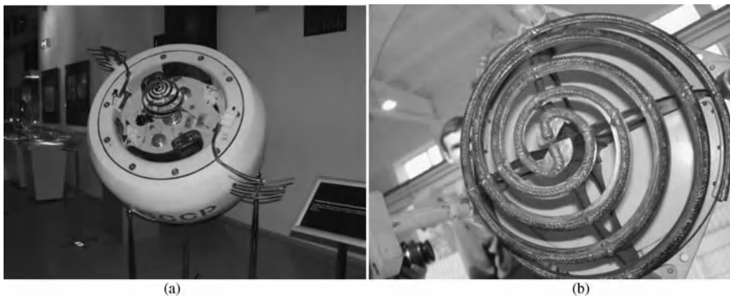
Figure 7.12 Telemetry and command antennas of early Russian landers. (a) Venera 4 lander with its spiral and Yagi antenna. (b) Blown-up model of a spiral antenna. Reproduced by permission of Sven Grahn.
