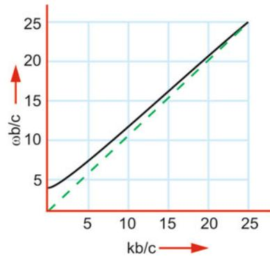
**Fig. 14.12** Dispersion diagram for the  $TE_{01}$  mode of rectangular waveguide for  $b = 2$  cm
