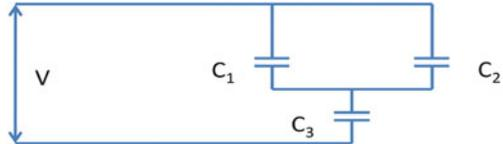
11.91 Capacitors  $C_1 = 8 \mu\text{F}$ ,  $C_2 = 4 \mu\text{F}$  and  $C_3 = 3 \mu\text{F}$  are arranged as in Fig. 11.15. A voltage of  $V = 100 \text{ V}$  is applied. Determine
