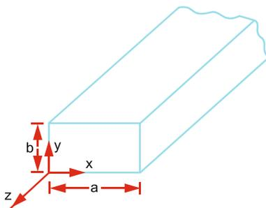
**Fig. 14.13** Rectangular hollow metal waveguide
