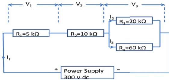
12.54 Apply Kirchhoff's rules to the circuit shown in Fig. 12.28 to produce three equations with three unknown branch currents. You do not have to solve these equations for individual  $I$ .
