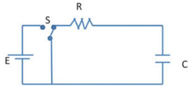
**11.93** Consider a circuit consisting of a resistor  $R$  and a capacitor  $C$  in series with a battery of emf  $\xi$  and a switch (Fig. 11.17). The capacitor is initially uncharged and the switch is closed at time  $t = 0$ . By considering the potential drop across each of the components of the circuit, verify that the charge  $Q$  on the capacitor has the form
