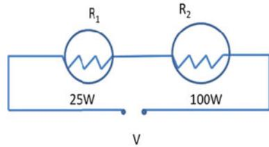
**12.17** A 25 W bulb and a 100 W bulb are joined in parallel and connected to the mains (Fig. 12.13). Which bulb will glow brighter?
