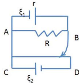
**12.32** A thin uniform wire 50 cm long and of  $1 \Omega$  resistance is connected to the terminals of an accumulator of emf 2.2 V and the internal resistance  $0.1 \Omega$  (Fig. 12.17). If the terminals of another cell can be connected to two points 26 cm apart on the wire without altering the current in the wire, what is the emf of the cell?
