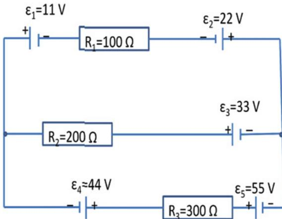
**12.53** Figure 12.27 shows a series parallel resistive circuit connected to a dc supply. For the circuit shown work out the following:
