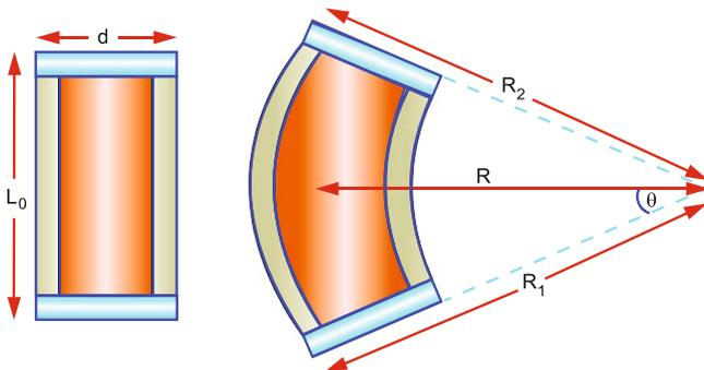
**Fig. 10.2** Expansion of a bimetal strip of bars
