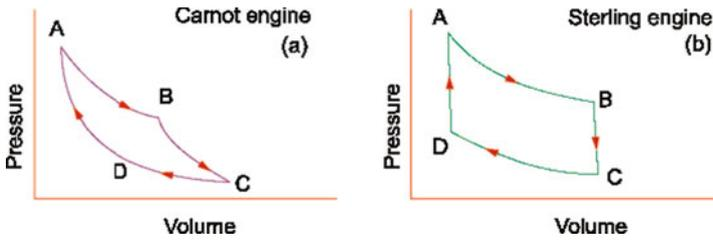
**Fig. 10.12** (a) Carnot cycle consisting of two isothermic processes AB and CD; two adiabatic processes BC and DA. (b) Sterling cycle consisting of two isothermic process AB and CD, two isochoric processes BC and DA
