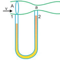
The pitot tube is a device to measure the flow speed of a gas. If  $\rho'$  is the density of the liquid in the manometer,  $\rho$  the density of the flowing gas and  $h$  the difference in height in the limbs of the manometer, then
