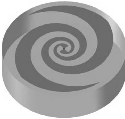
Figure 2.9 A two-arm log-spiral antenna backed with a cavity.
