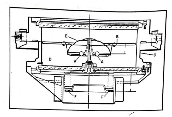
Magnets (A): These are four (two in older compasses) cylindrical bundles of magnetic steel wire or bar magnets which are attached to the compass card to supply directive force.
