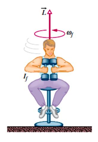
No net external torque acts on the system consisting of the student, stool, and dumbbells. Thus, the angular momentum of that system about the rotation axis must remain constant
