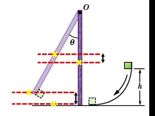
$$\frac{1}{2}I_{tot}\omega^{2} = mg(d - d\cos\theta) + Mg(\frac{d}{2} - \frac{d}{2}\cos\theta) \implies (1 - \cos\theta) = \frac{\frac{1}{2}I_{tot}\omega^{2}}{mgd + Mg\frac{d}{2}} = 0.15$$
